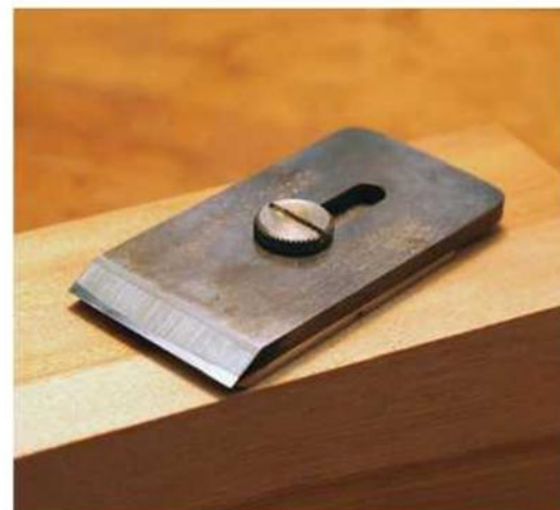
Solid combination. The Hock blade assembly was designed for this type of plane. It has a thick cutter and cap iron.
