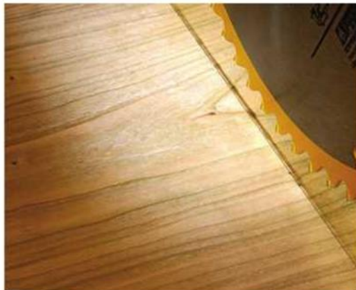
The shadow knows. DeWalt offers an optional light that uses the shadow of the blade for lining up cuts. It works as well as a laser, and lights the work area.
