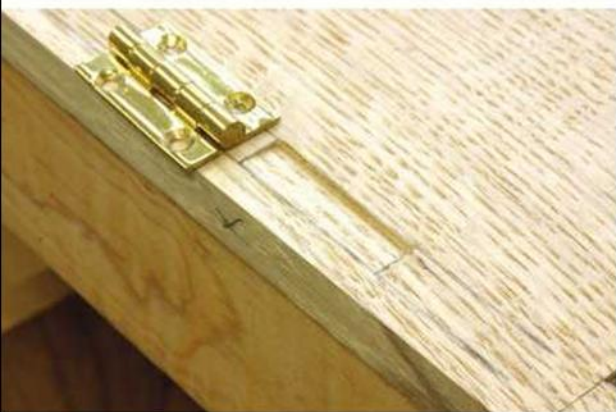
Ramping up a hinge mortise. Installation of the hinges is tricky because the door is slightly recessed into the clock. A ramped mortise allows you to bury the hinge leaf and keep the barrel aligned as needed.
