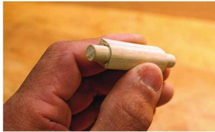
Turned tenons, planed radius. The cross bar features turned tenons; the center section has a flat side to secure the wedge, with the opposite edge rounded to help clear shavings.
