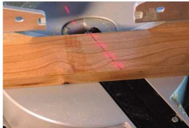
No spin zone. Laser guides mounted on the saw can be used to set precise angles as well as to align the blade to a line. Blade-mounted lasers require the blade to be spinning to turn them on.
