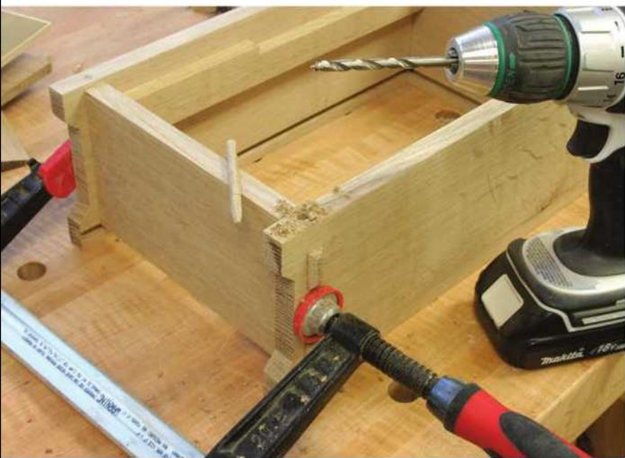
Pegged joint. The mortise-and-tenon joint is held together with a dowel that extends well into the first tenon. I made this matching-hardwood dowel by driving the stock through a series of graduated holes in a dowel plate until I reached the 1/4" diameter.
