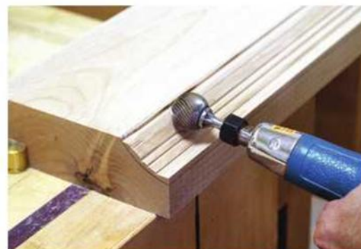
Big coves, no problem. A hand-held die grinder with a ball mill is the tool of choice for creating large coves.
