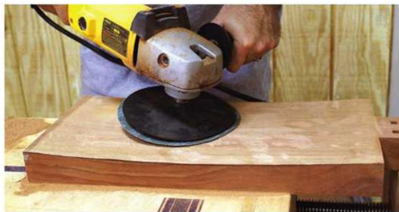
Smooth out the rough spots. A polisher makes quick work of leveling the surface.
