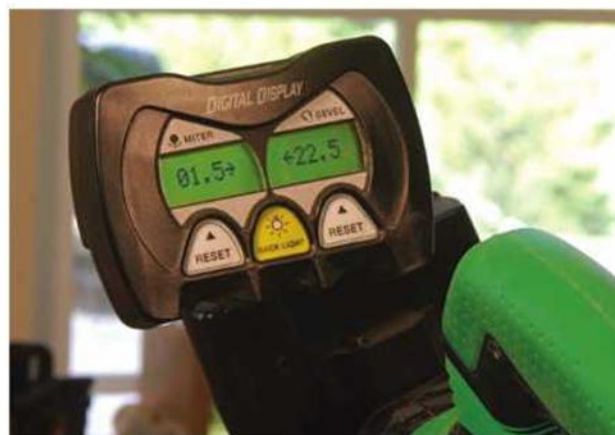
Digital double-play. Hitachi has a digital display and fine adjustment knobs for both miter and bevel angles, reading to 0.5°.
