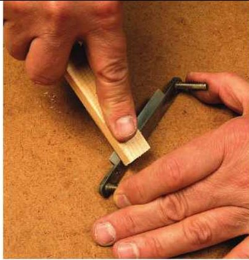
Cheap sharpening jig. A piece of sandpaper stuck on a small piece of wood is perfect for removing any rounding in the blade. But this is a time consuming method.
