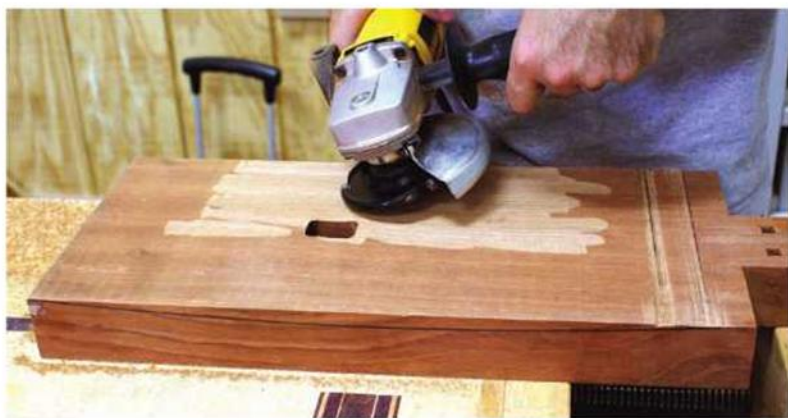
Let the chips fly. An angle grinder and a carving blade make one powerful combination! Hold the tool close to horizontal to avoid sculping deep gouges.
