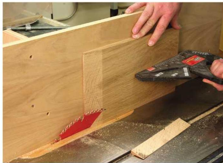
Know your period. I found myself stuck in the 18th century when I made the clock back. If you're positioned differently, you might just want to mill your stock to a 1/4" thickness and do away with the bevels.
