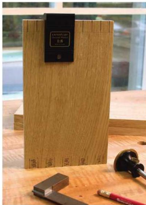
Measure and mark. Layout on the dovetails begins with accurate sizing. Work from the face to the angled lines on the board's end.
