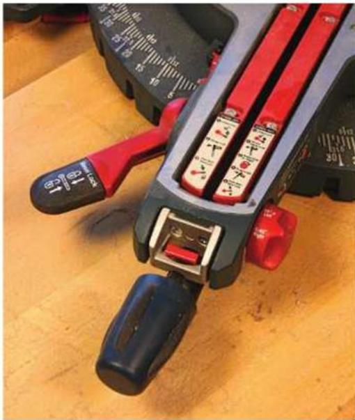
Front and center. Bosch puts all the controls for setting miter and bevel angles in one convenient location.
