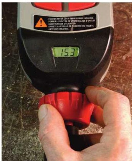
To a fine degree. Milwaukee adds a digital readout and fine-adjustment knob to set miter angles to 0.1°.
