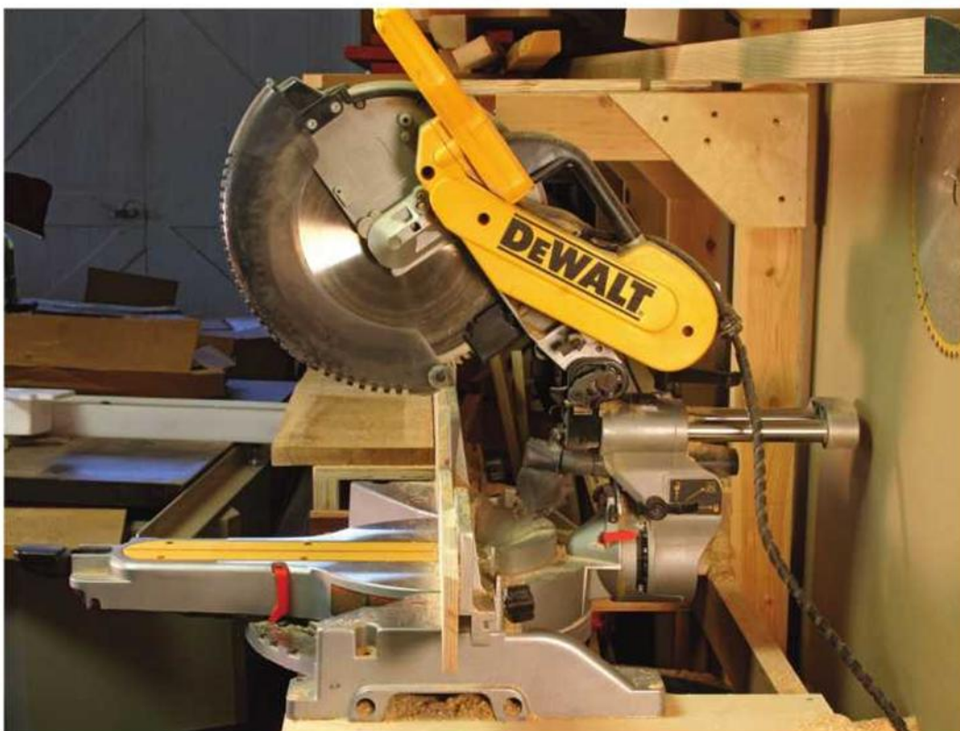
Consider the back. Most of the saws in the test require a lot of space behind the fence. The DeWalt (with the dust bag removed) and the Hitachi take less room than the others.
