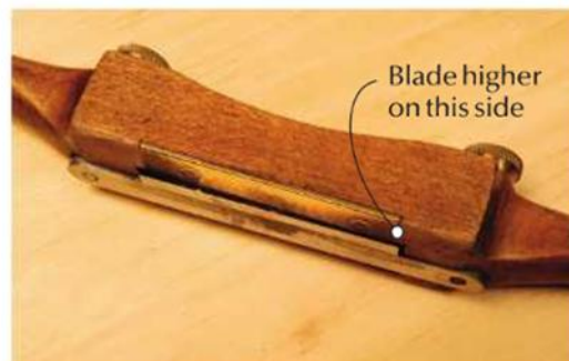
Tricky setup. Set the blade so that it’s a bit higher on one side; that way, by moving the tool left and right, you have every setting you need without changing the tool’s setup.
