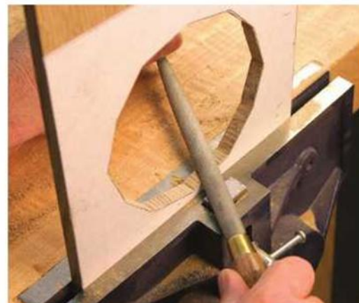
Raspy detail. Small variations in the faceted edges are magnified when viewed as a whole. Spend some time to bring the edges to your layout lines.
