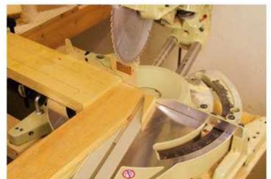
The right angle. The setup shown above allows you to create the beveled feet with a miter saw.
