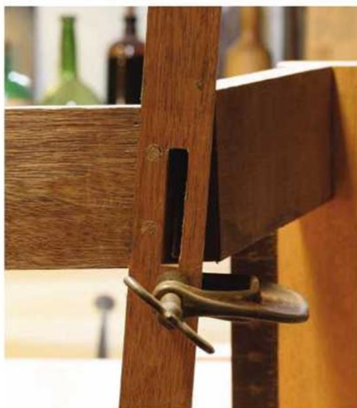
In position. I have the side seat rail positioned correctly. The exposed material to the right of the leg will get planed flush with the back leg later.
