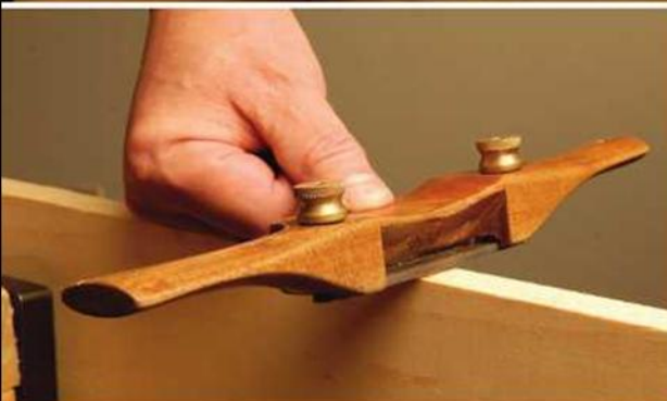
Training. Set the shave flat on your work, then place your thumb in the curve to slightly increase the angle; that's the correct angle for use.
