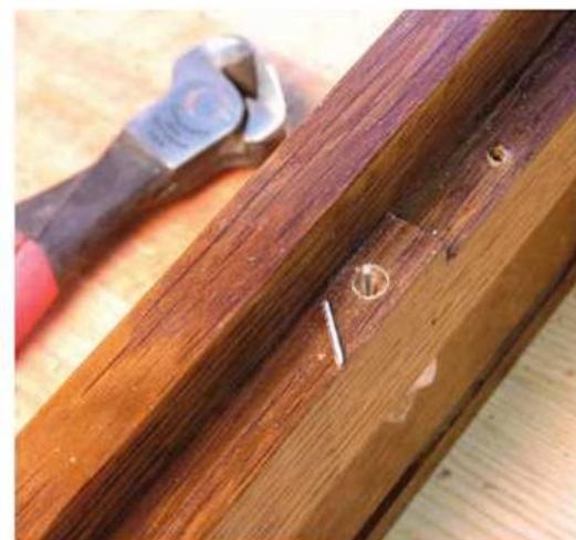
A trick to install magnets. A brad driven into the center of a hole sized for a magnet will locate a second hole location by simply closing the door.
