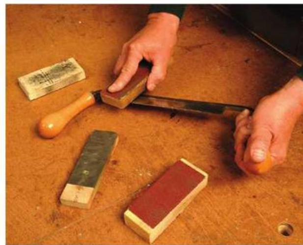
Dress all surfaces. Make sure you dress the entire curve on the front of the blade to maintain its original shape. Don't just dress the edge, or the angle will gradually increase.
