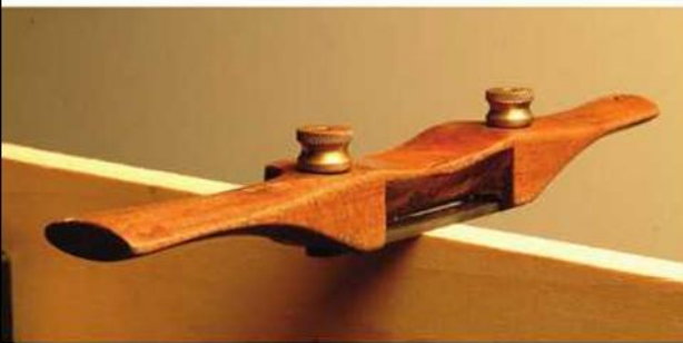
In a pinch. The handles suggest that one grip the shave by the handles. However, more control is gained by pinching it in the center.
