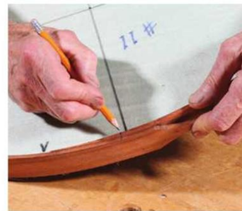
Mark it. Record your tight wrap by a pencil mark. Remove the band from the foam core, and use this mark as a reference for sizing the tray. By going 1/8" past the mark when tacking, the resulting size will fit snugly back on the form.
