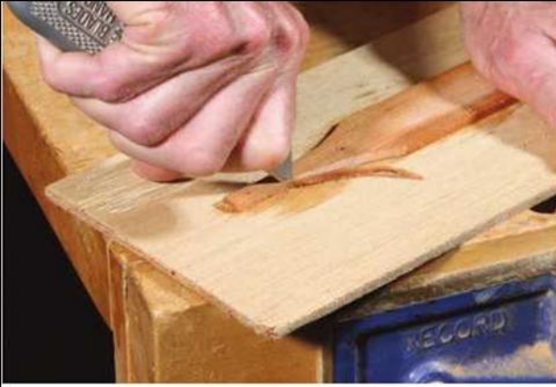
All trim. After cutting the profile of the finger and drilling \frac{1}{16} " holes for tacks, the edges are trimmed with a sharp knife.
