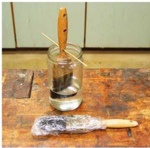
Storing brushes. If you are using a brush almost every day, you can store it by hanging the brush in the solvent for the finish or by wrapping the brush in plastic wrap. Notice the holes in the brush handle for suspending it in different-sized jars. You shouldn't let the bristles rest on the bottom for any length of time or they will adopt a permanent curved shape.
