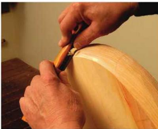
In a pinch. The handles suggest that one grip the shave by the handles. However, more control is gained by pinching it in the center.
