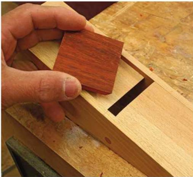
Watch your mouth. Carefully measure and fit the fill-in piece to ensure a tight mouth.
