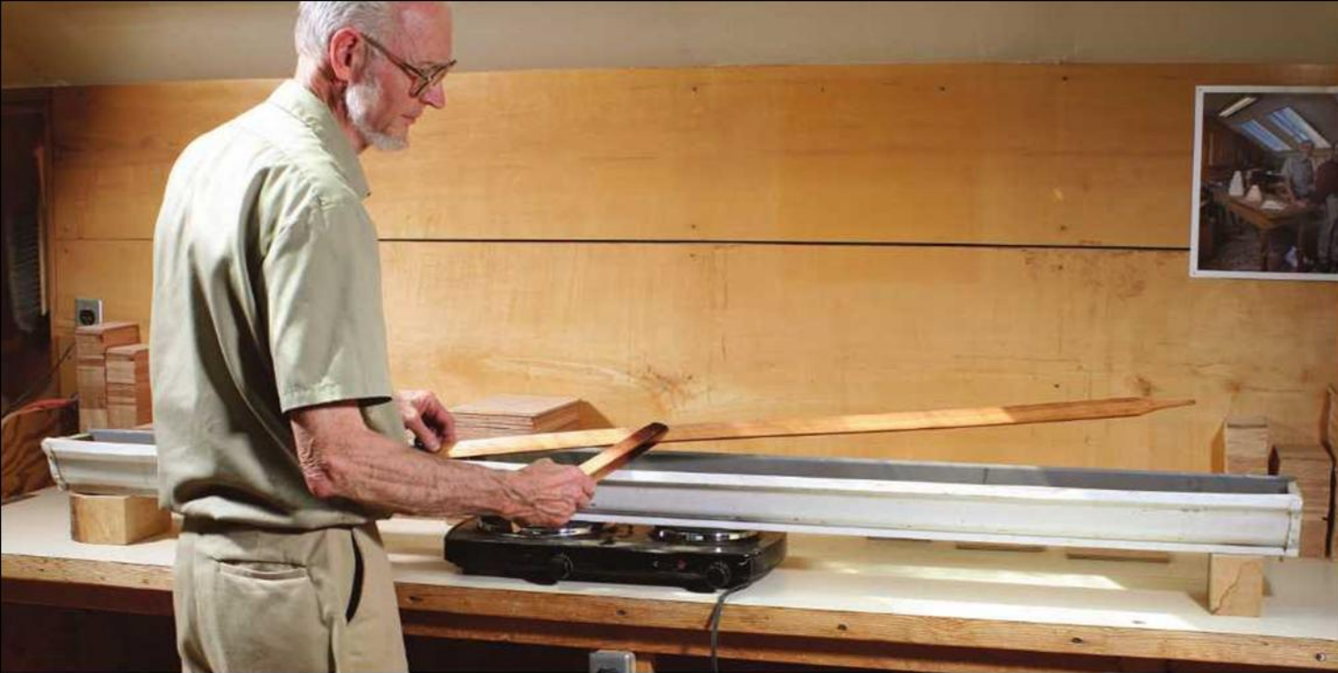
A nice hot bath. Bands need to soak to make them flexible for bending. Hot water is heated in a 6' length of rain gutter. A hot plate provides the heat. Wood blocks under each end give stability to the long tray.
