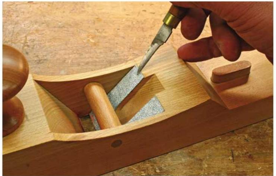
A simple solution. Sandpaper shims can be used to fine-tune the mouth opening if it is larger than desired.
