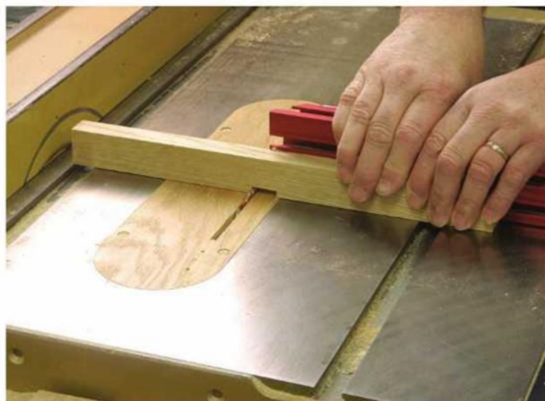
The first of two steps. Form a notch in the supports that will eventually accept the dial back. A number of passes over the saw blade will carve out an area that makes finishing the rabbet a breeze.
