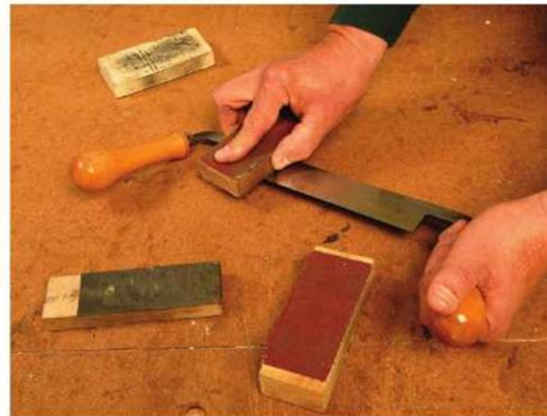
Flat bottom. Although the blade should be ground with a knife edge, the back of the drawknife should be flat, like a chisel.
