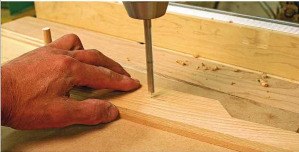
Save your place. Drill both holes for the cross bar at one time on the drill press.
