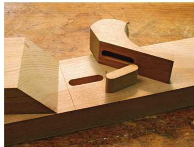
Hold on before gluing. The handhold and plane body are mortised before regluing the body.
