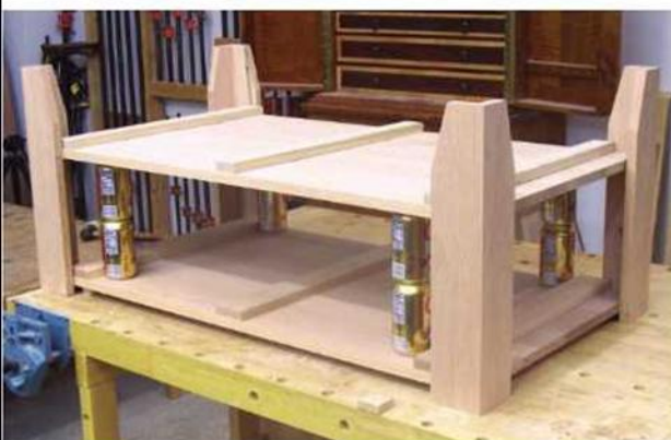
Squared up. Everything may be in position, but if your table is not square to the flat surface, you will find it extremely difficult to add the finishing pieces to the table.
