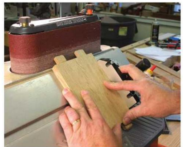
Hybrid woodworking. This sander's table adjusts to 45°. Another way to chamfer the tenon edges is with a miter gauge at a disc sander. No matter which method you use, the ends of the tenons require handwork.
