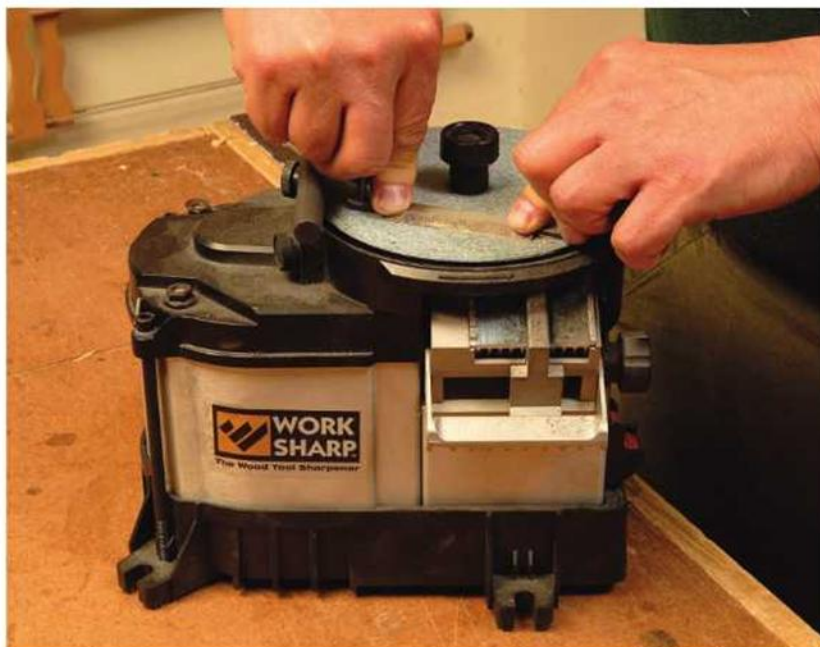
Work Sharp. A more expensive – but easier-to-handle – blade sharpening method is the Work Sharp.
