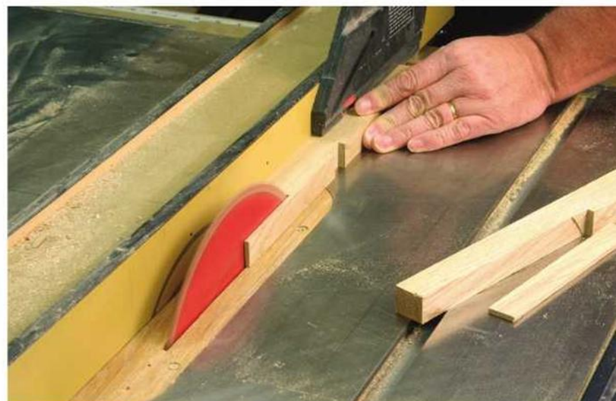
The second of two steps. The support rabbets are finished when you rip the material up to and including the notch. A small amount of waste needs to be cleared prior to the addition of the dial back.
