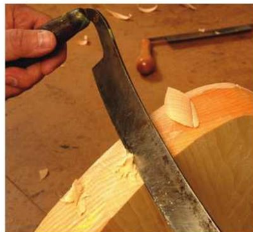
Unclean cut. If you hold the knife upside down, the angle of the blade is higher and you're likely to get a crumply shaving and rough surface.
