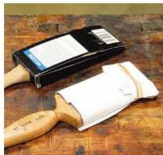
Storing clean brushes. When the bristles are clean, shake out the water and return the brush to the holder it came in or wrap the brush in paper so the bristles dry straight and stay clean. You can use a rubber band or masking tape to secure the paper.
