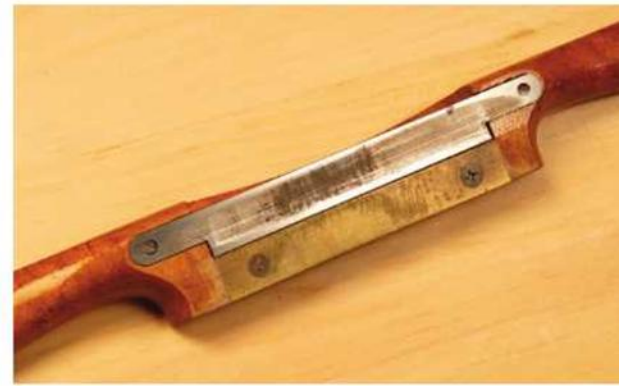
Hollow grind. Cutters with hollow-ground bottoms make sharpening fast – only two narrow strips of metal have to be dressed rather than the entire blade surface.
