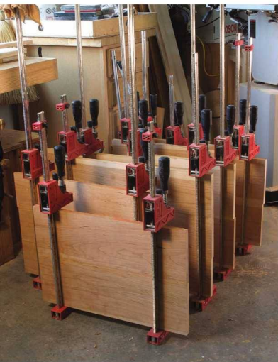
A sea of panels. I wanted to glue up all the panels at the same time—but I ran out of clamps and space. Above are the six door panels and two lower side panels.
