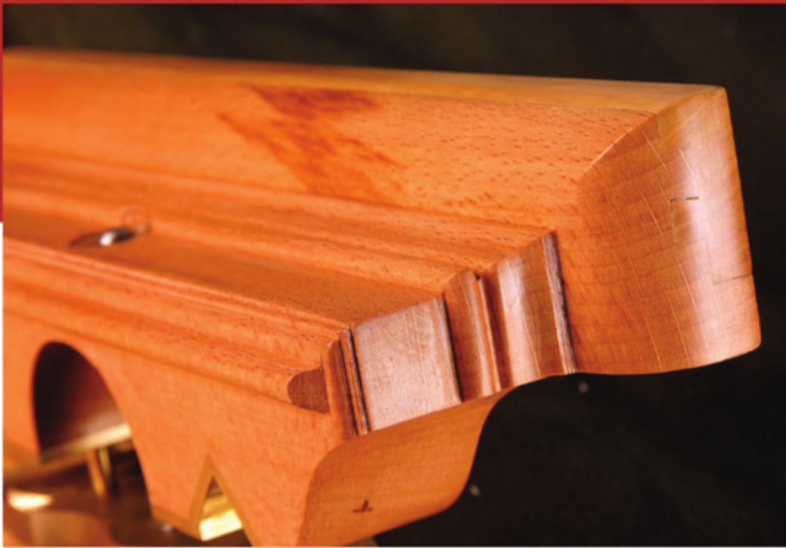
Complex and crisp. The moulding on the fence is remarkably crisp, even as it returns across the front. Here you also can see (if you look closely) the boxwood lining and the two sliding dovetails that attach it.
