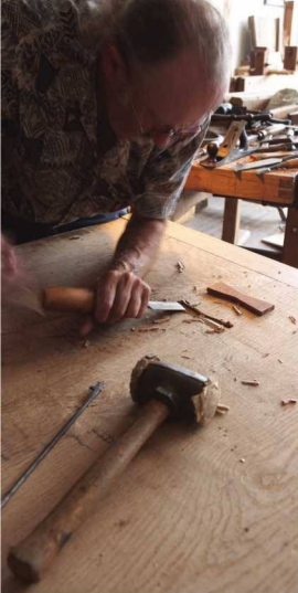
Fine-fitting the inlay. After cutting the butterfly inlay to shape, I cut the recesses to receive them using a chisel and then a router plane.
