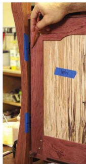
Quick, accurate locator. A few shims hold the door and allow for direct transfer of the mortise centerlines from masking tape to door.
