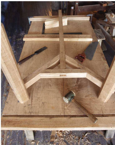
Almost assembled. Here you can see how the stretcher assembly comes together. All the tenons are through-tenons, with the exception of the angled tenons that meet.
