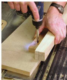
2 Position blocks. \frac{3}{4} " x 1\frac{3}{4} " blocks are screwed to a \frac{3}{4} "-MDF base that's 8" wide and 6" longer than your leg to position the legs for tapering. Attaching the stops with #6 x 1\frac{1}{4} " drywall screws alone (no glue) allows you to quickly reconfigure this jig to cut different tapers.
