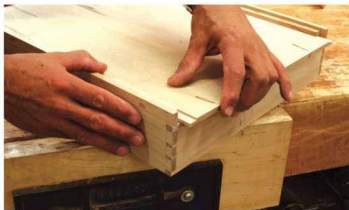
Match the groove. The rabbet in the drawer bottom matches the width of the grooves in the drawer sides and front. The extra thickness in the bottom keeps it from sagging.
