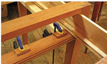
Stop right there. Assembling and fitting the drawer before installing the drawer bottom allows precise placement of stops glued to the lower rail.
