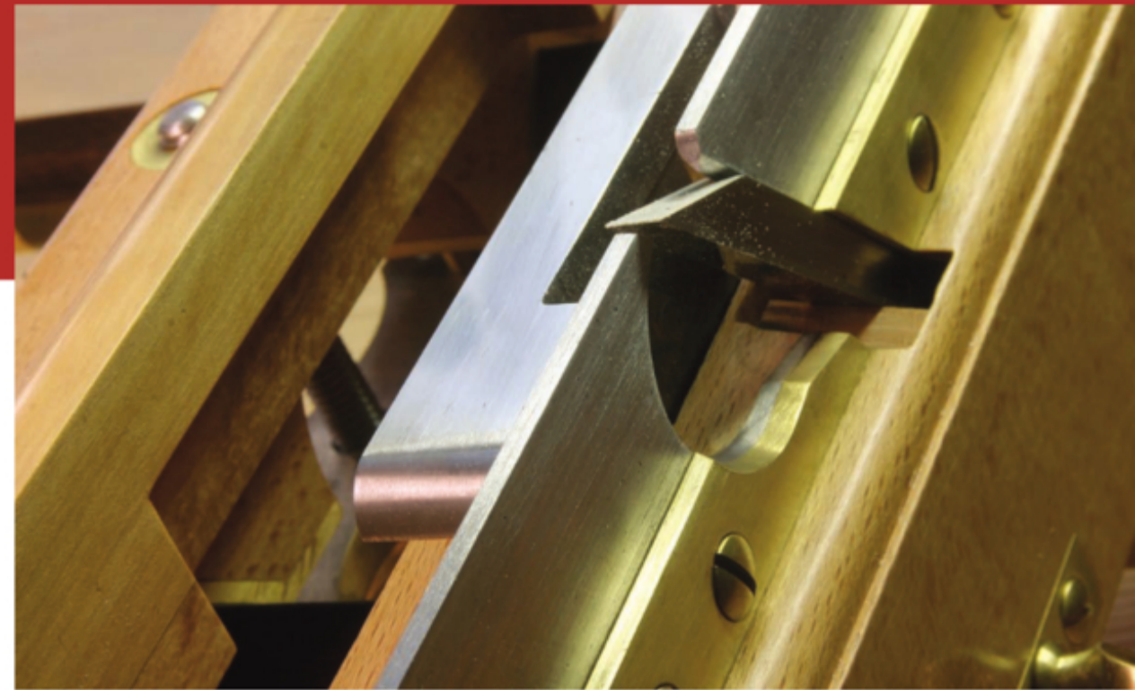
Brass, iron and wood. The skate iron and depth stop all come together seamlessly. The tapered A2 irons all seat firmly against the skate and are held securely by the wedge. The set of eight well-made irons is just one of the selling points of this tool.
