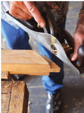
Plane to fit. I use a carriage maker's plane to trim the cheeks of the tenons for the hay rake stretcher.
