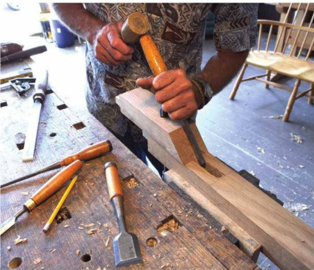
Let your waste be your guide. Use a guide block to steer your chisel when you chop the angled mortises for the hay rake stretcher.
