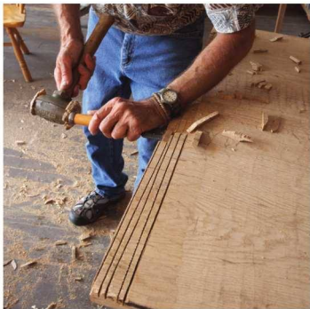
Remove waste in haste. A few good whacks with a chisel and mallet popped out most of the waste.
