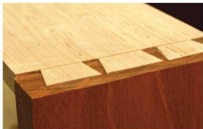
Proud sides. Cutting the dovetails to leave the sides extended from the drawer front simplifies fitting and maintains the smallest possible gap between the drawer and carcass.
