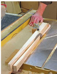
1 Simple setup. A few pieces from the scrap bin and a handful of screws are all you need to make this jig.
