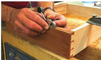
Rabbeted reveal. A small rabbet on the underside of the drawer front provides an even reveal to match the gaps at the top and sides.
