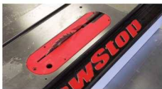
Steel reinforced plastic. Even with a steel backing, the insert flexes a bit at the back.
