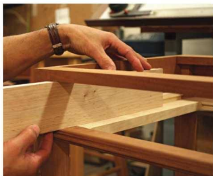
A fitting start. Fitting the width of the drawer side to the height of the opening before building the drawer gives more control of the process.
