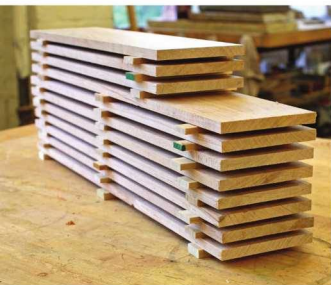
Let it rest. If you resaw thicker boards for drawer material, sticker them and let them sit for several days to acclimate before milling the stock to final dimensions.
