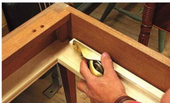
Short and sweet. The drawer guides have a rabbet on the bottom and stop short of the back. This allows them to be planed during the fitting process.
