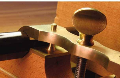
No-fail locking mechanism. The bridle mechanism is flawless in workmanship and in function. The fence locks parallel to the skate every time, which saves an immense amount of fussing.
