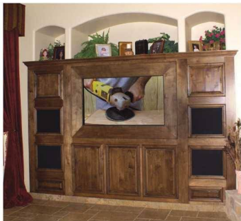
Not in inches or feet. Two story sticks were all it took to determine size and length, as well as position, of each piece of this entertainment center facade.
