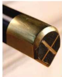
Handworked details. The brass caps on the ends of the ebony stems are wedged tight. The amount of detail on this plane is extraordinary.
