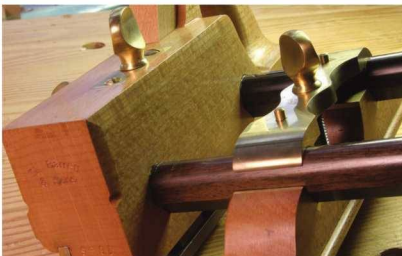
No-fail locking mechanism. The bridle mechanism is flawless in workmanship and in function. The fence locks parallel to the skate every time, which saves an immense amount of fussing.
