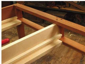
Details make the difference. The drawers ride on the rails of the web frame, and the guides restrain movement from side to side.
