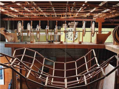
The Square Wave. Two camshafts work in unison to add together orthogonal waves in a suspended wooden grid.
