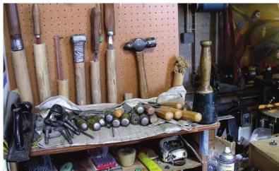
Chisels, gouges and rasps. The handles for the files and rasps are made from an acacia tree that was cut down nearby. The holders are made of bamboo.
