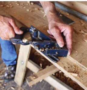
Trimming by hand. Then I cleaned up the cheek and shoulder using my rabbit plane.
