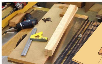
1 Simple setup. A few pieces from the scrap bin and a handful of screws are all you need to make this jig.
