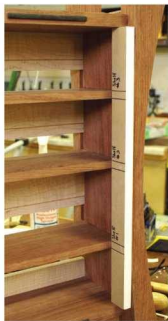
On the level. This small story stick was used to position the shelves in this cabinet, ensuring the shelves were equally spaced.
