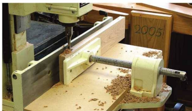
Many mortises. The majority of joints in this project are mortise and tenon. Take the time to set the hollow-chisel mortiser to cut dead-on centered mortises, 1/4 " deep—it will save you a lot of frustration and time later.
