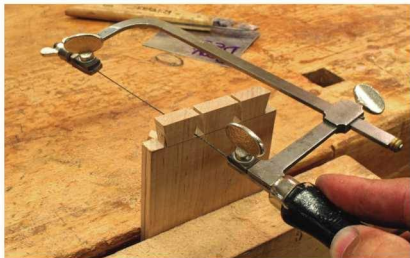
Wasting away. With thin drawer stock a jeweler's saw or coping saw will remove the waste between tails quickly and without the risk of damaging the work by chopping between the tails with a chisel.
