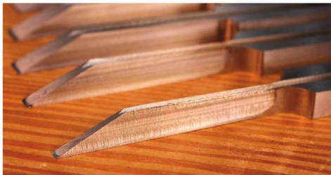
The right irons. The irons that come with the Barrett plow plane are a joy, especially if you have been messing with vintage ones for so long. The irons are well ground and properly shaped.
