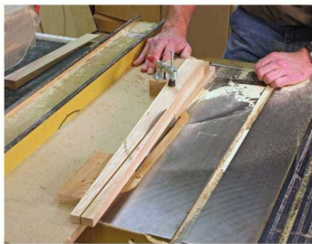
4 Turn for second cut. After the first cut is complete, turn the leg 90^\circ and clamp it back in the jig.
