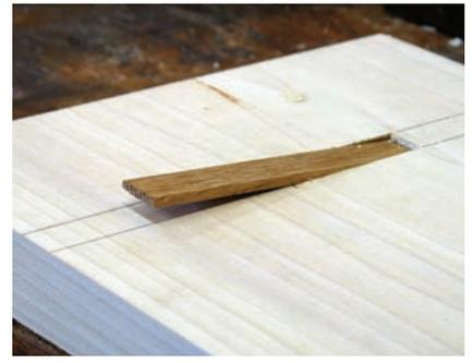
**A different application.** A spring lock is fit into a drawer bottom. From here, it's easy to fine-tune the fit so the lock catches the drawer face and holds the drawer closed.
