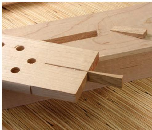
**Ready for wedging.** Here's the parallel guide right before we glued it in place and wedged it with a sliver of oak. We cut a kerf down the middle of the tenon to give the wedge a place to go.
