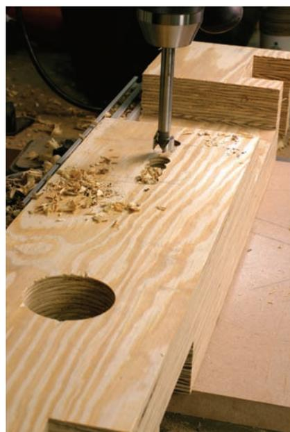
**Holes to guide you.** The through-mortise in the leg allows the parallel guide to pass freely in and out. You don't need to square the ends of this mortise. Leave them round. The parallel guide is narrow enough to pass through.
