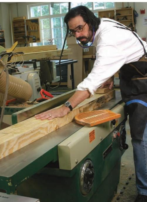
**Jointing with carbide.** Our jointer has a carbide-insert cutterhead, and it had no problems dealing with the glue in the LVL. I was more worried about the planer, which has high-speed steel knives.
