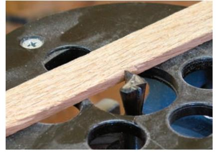
**Is power the choice?** The sliding key is flush, so you can use a router to make the dovetailed slot. Set the depth of cut equal to the sliding key thickness, set a straight fence to run against then cut the slot. Or cut the slot by hand.
