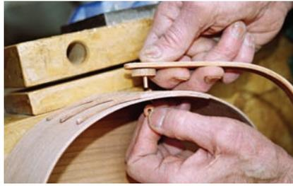
**14 Rivet sequence.** The rivet sequence is: copper trunk rivet, handle,  $\frac{3}{16}$ "-thick wood spacer, the box side in which has been drilled a  $\frac{5}{32}$ " hole, the copper washer for the inside end of the washer.
