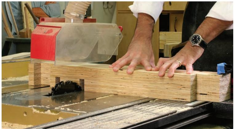
**The whole stack for half-laps.** This is a lot of meat for a table saw to remove, but our cabinet saw was up to the task. If your saw isn't, a band saw will remove most of the waste and the dado stack can clean up the cuts.
