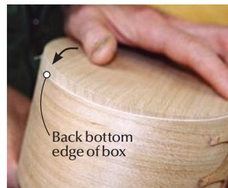
**10 Fit the bottom.** The oval board is fitted into the bottom by setting it against the front lap and then working the back into place. This will ensure that the feathered end will not be damaged in the process of pushing the oval.
