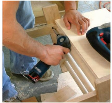
**Quick assembly.** A few screws in concealed locations hold the pieces securely together.
