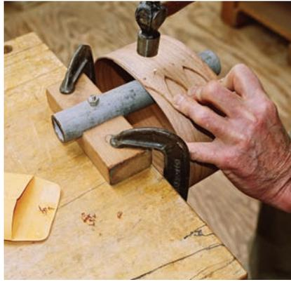
**6 Tacks.** Small copper tacks  $\frac{1}{16}$ " longer than the two thicknesses of veneer are used to clinch the lap. No glue is used. The wood cradle secures the pipe anvil to the bench.
