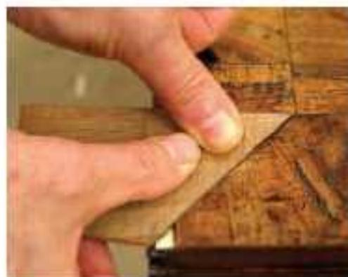
**8 Rub joint.** Because of its thickness, I can glue the veneer patch, which I cut thicker than needed (called "leaving proud"), quickly and simply using a rub joint. But clamps wouldn't be difficult to arrange here.
