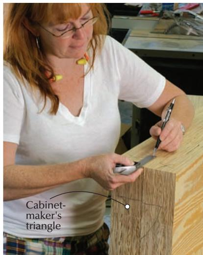
**Triangles and squares.** Note the "cabinet-maker's triangle" scribed across the tops of the four legs. This helped you keep all the legs oriented as you mark out the half-lap joints for the stretchers.
