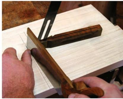
**It's a compound cut.** Use a bevel gauge, set to the angle planed on your key, to align your saw as you define the dovetailed channel. After the edges of the channel are sawn, use a chisel to waste out the material.
