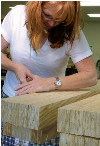
**Scraping glue.** After gluing up four strips into a chunk, we scraped off the excess yellow glue before dressing the lamination on the jointer. After all, the knives were already taking a beating from the glue between the plies so removing any glue we could was an act of kindness.
