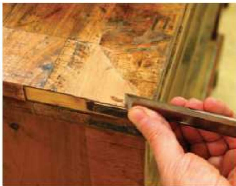
**9 Leveling.** I use a block plane, scraper and sandpaper to level the veneer patch to the surrounding wood. It's important to avoid cutting into the surrounding old veneer. If you cut off some of the aged surface wood, you may expose wood that is lighter or darker and create difficult color-matching problems. Applying masking tape around the patch can be helpful. Working slowly and carefully is essential.
