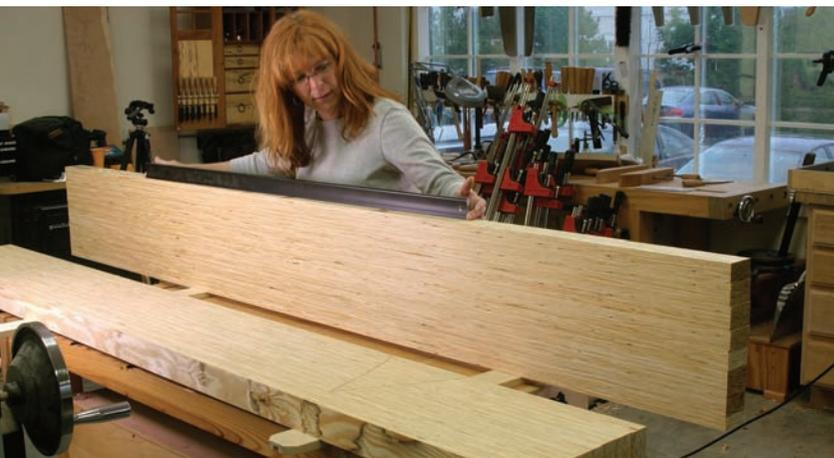
**Looking for bumps and hollows.** When dealing with an 8'-long edge, it can be difficult to find the source of the problem with an edge. We balanced a straightedge at several places along the edge, then pinched the ends of the straightedge. If the straightedge rotated easily, there was a hump under it. If the corners dragged and there was light under the straightedge, we had a hollow on that edge.
