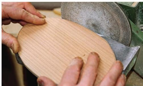
**9 Two-degree angle.** The disc sander finishes the edge up to the pattern line. The sander table is elevated to 2° to provide a slight cork effect to this ellipse for a tight fit. To make this adjustment, you may need to file out the slide slot so it no longer stops at 0°, or you can remove the thumb screw and use a small C-clamp.
