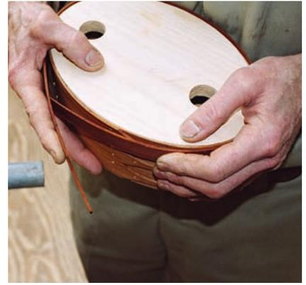
**7 Shapers.** Once tacked, wood corks called shapers are put in both sides to hold the box shape for one to two days of drying. The  $10^\circ$  edge bevel and the holes for ventilation are a hallmark of this piece of bench equipment that is key to the Shaker system of production. The top band is wrapped on the box itself. It will be tacked then returned to the box for drying. Note that the direction of the band finger matches that of the bottom band fingers.
