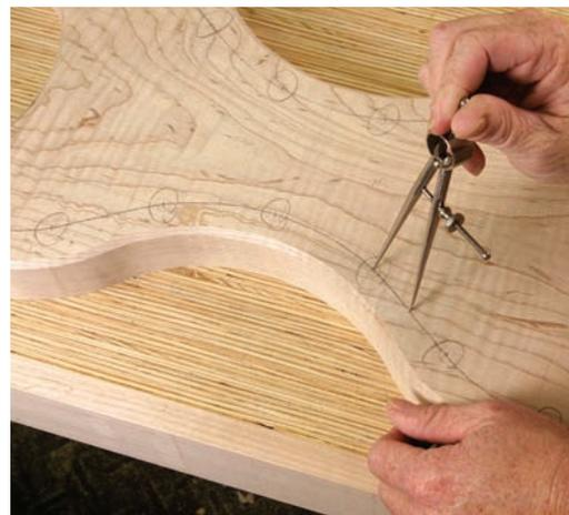
**Walk it off.** Dividers are the absolute best way to space the holes in the deadwoman. To offset the holes, simply bore a hole at every other mark left by the dividers.
