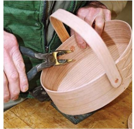
**15 Trim excess.** Snip off the excess length of the rivet, or take it out and grind it to the proper length.
