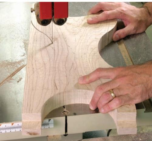
**Cutting curves.** These curves actually are more than eye appeal. They are convenient places to grab the board jack to slide it or to sneak a clamp into.
