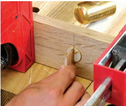
**A short drive home.** The wedges spread the ends of the tenons, making them tight in the mortises in the legs.
