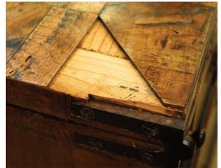
**4 The challenge.** Above the hinge you can see damage to the substrate that must be repaired so the veneer has something to bond to. Also, you can see that the veneer is considerably thicker than modern 1/32"-thick veneer. Thick veneer is common on furniture made before the machine age. Veneer seems to get thicker the older the furniture.
