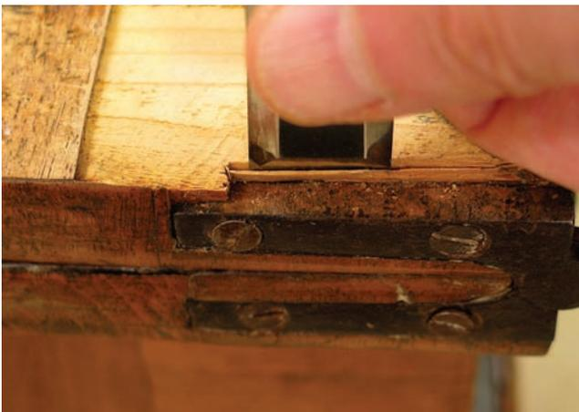
**5 Straight edges.** Again, it's always easiest to work with straight edges. So I'm cutting one using a chisel.
