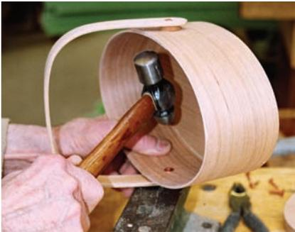
**16 Peen.** Peen the rivet until the handle is secured and will stay put.
