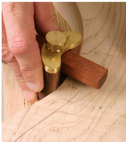
**A special marking gauge.** Because I do a lot of work with chairs, I have this marking gauge with a special fence that allows it to follow curves. If you don't have a gauge like this, it's easy to modify your standard gauge. Take some  $\frac{3}{4}$ " dowels, plane a flat on them and glue two short sections to the back of your fence. Turn your fence around and you'll have a gauge that does two operations.
