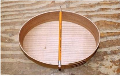
**13 Location.** Locating the center front and back from which the hole location is 1" down. Set your box on the floor and look down from a standing position.
