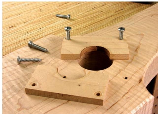
**Can't-miss garter hole.** Clamp the two halves of your garter together and bore the hole right through them. Our garter hole needed to be 1<sup>5</sup>/<sub>8</sub>" in diameter to match the dimension of the shaft of the vise's screw.
