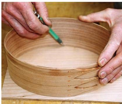
**8 Mechanical pencil.** Here I'm tracing the oval on the 1/4" boards used for tops and bottoms. A mechanical pencil will ensure accuracy of this line.
