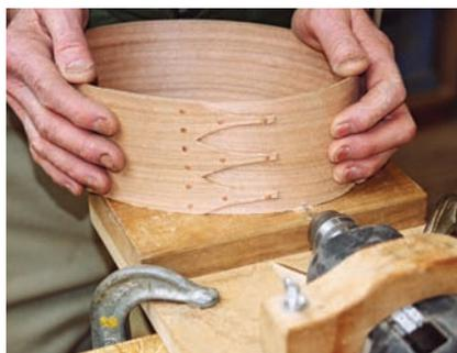
**11 Drill for pegs.** After the oval board is in place and sanded flush, drill the perimeter every 2" to 3" for wood pegs. This drill jig locks a spare drill to a board with a front table the right height to center the hole on the 1/4" board inside.
