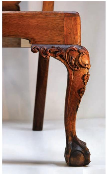
**Sealed.** The dry pigments can be removed pretty effectively by adding more oil and wiping. So I applied a light coat of butonlac shellac to seal in the color. Much more needs to be done to this knee and obviously the foot. From here I can add more tinted oils (with less of a chance of disturbing what is under the shellac) or just tint the shellac.
