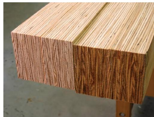
**Ripped and ready.** We began by ripping down the LVL 2x12s we needed for the benchtop and were surprised by how easily the material cut on the table saw with a combination blade.
