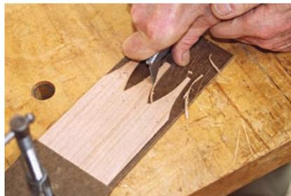
**2 Trimming.** My preference for trimming is a utility knife with a fixed, not retractable, blade. This gives the necessary control. Use heavy-duty blades, not the lighter ones that come with a new knife.
