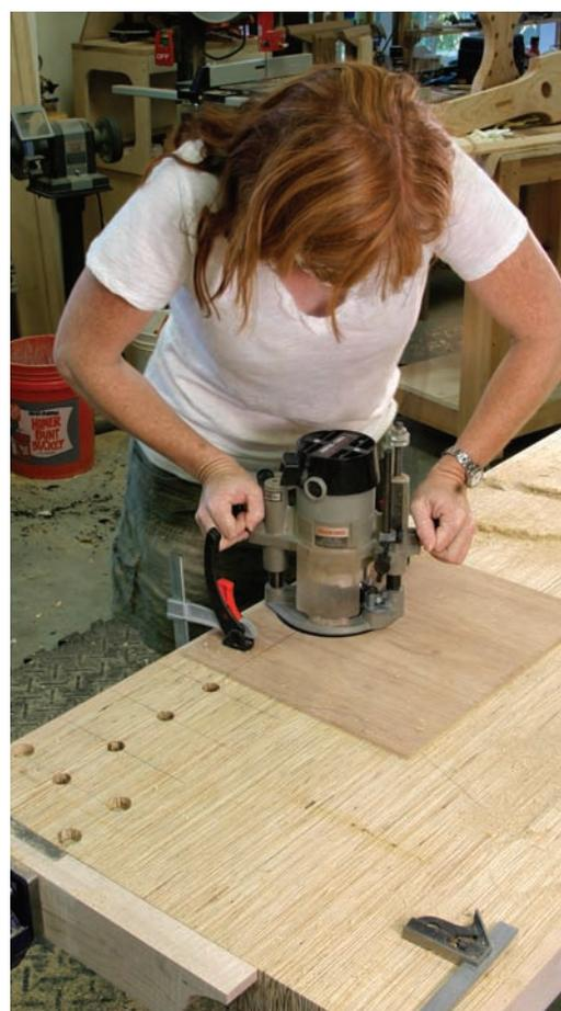
**More nasty dust.** The  $\frac{3}{4}$ " upcut spiral bit and template makes short work of this operation. Lay out all your holes on the benchtop, then position the template and make your plunge. The template is marked with crosshairs that align things with your layout marks.
