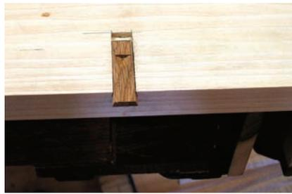
**Compact and flush.** The sliding dovetailed key, nestled into its slot, is sometimes missed during inspection due to the flush fit.
