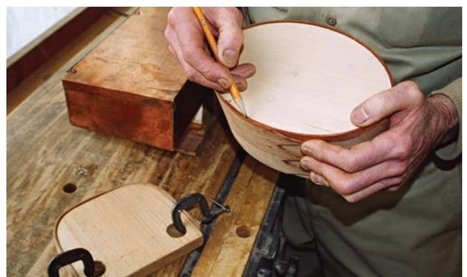
**5 Core.** The wet band is wrapped around a core the size of the inside of the box. Here the wrapped band is marked so that the core can be removed and the band returned to its proper size. Note that all the band's fingers are held to prevent them from splitting. The mismatch at the lapped edges of the band is common at this stage and will be made even when tacking.
