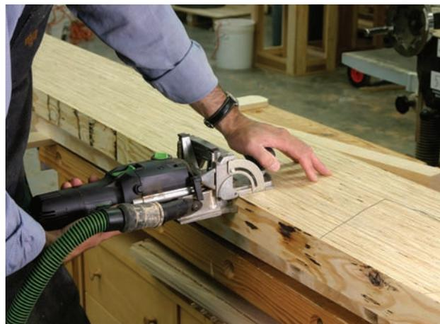
**Dominos will do 'ya.** You can use almost any method to align the two edges you are gluing up for the top: biscuits, splines or even dowels. We have a Festool Domino in the shop, and it's perfect for this sort of accurate work.
