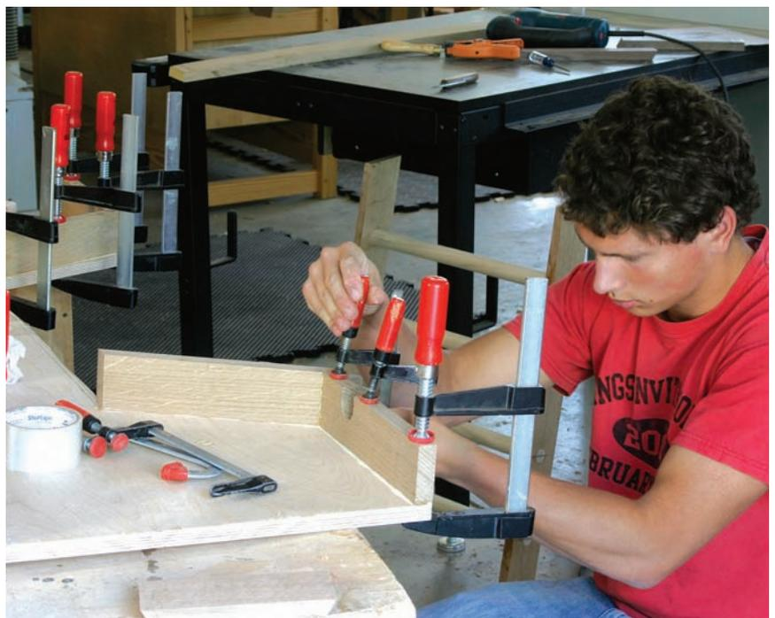
**Glue is enough.** The connection between the plywood and solid wood is long-grain to long-grain, so a glue-only joint will be solid.
