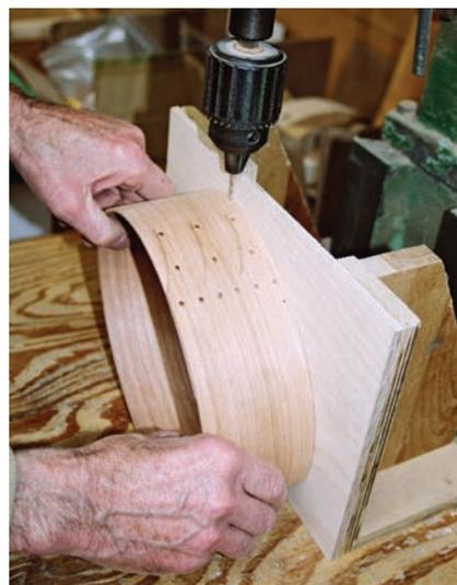
**12 Alternate approach.** An alternative drilling method makes use of a drill press. The jig, which is shaped like a bookend, creates a vertical drilling station.
