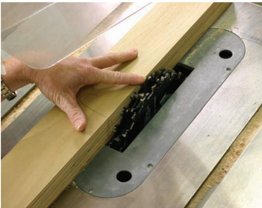
**How high? This high.** The actual height of the dado stack isn't important. What's key is that the cutters be just as high as your stretchers are thick. Place a sawtooth at top dead center and compare it to a stretcher.
