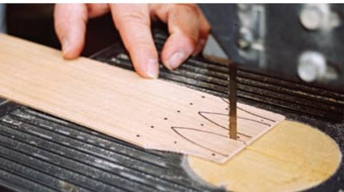
**1 Fingers.** Profile the finger design to rough dimensions before final trimming with a utility knife. The locations for copper tacks are drilled at this time, too.
