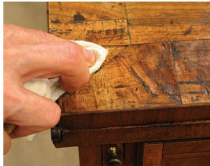
**3 Cleaning up.** Though it's possible to reglue right over old hide glue using hot hide glue, it's best to clean off the old crumbly glue (and whatever contaminants, such as wax, that might be on the surface) before gluing the patch. Here I'm washing off the old glue with hot water. All contaminants come off with the glue.
