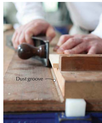
Dust collection. The improved joint-and-square board distributes the cutting action across the plane blade’s cutting edge. The dust groove collects any shavings that could lift the plane out of square.
