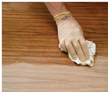
Wiping on. To apply a gel varnish, simply wipe it on the wood like you would an oil/varnish blend. You can use a brush to help get the thickened varnish into recesses and inside corners, but wiping is much faster on level surfaces. You can wipe in any direction.
