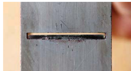
Straight edge. Your plane blade's cutting edge should be straight.
