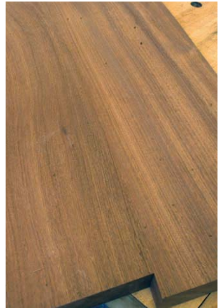
Where's the joint? Two routed edges, joined together, produce a tight, clean and nearly invisible seam.
