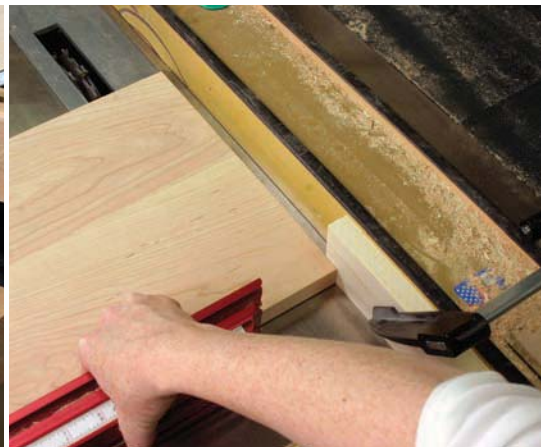
More jigs. Again faced with secure workholding problems at the table saw, I used a handscrew attached to the sliding table to support one end, and an stepoff block at the other to safely locate the groove for the bottom fixed shelf.
