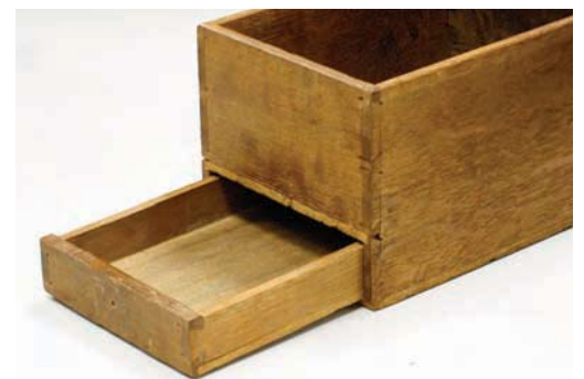
Mixed materials. This chest's drawers are constructed of 1/2" walnut drawer fronts, 1/4" riven white oak sides and 1/4" sawn yellow pine bottoms. Was this choice of materials based on utility, availability, or ease of stock preparation?
