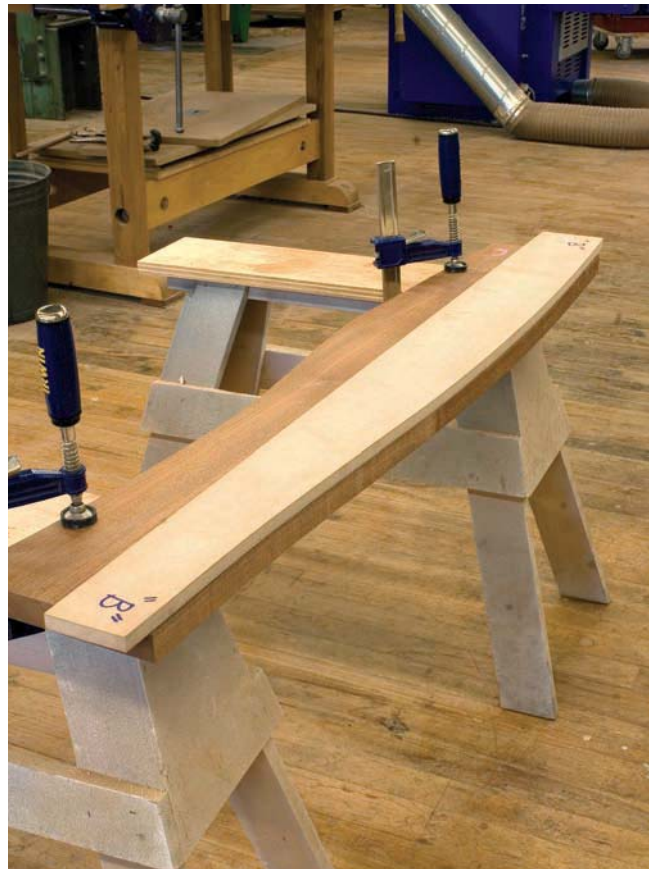
Ready to rout. The working pattern should be securely attached to the workpiece before routing. In this case, I used double-sided tape.
