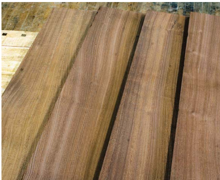
Nice arrangement. Rough-cut boards are arranged for the best color and grain match.
