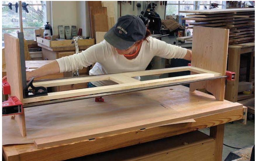
Framed. The pocket-screwed web frame was glued into the side panel grooves and squared up before I tightened down the clamps.
