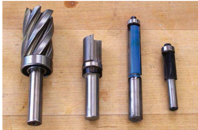
Flush trimming. All of these bits are flush-trimming bits. Notice that you can get bits with the bearing on the top or bottom, in different sizes and with different shank diameters. What you buy depends on your router and routing needs.
