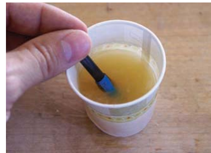
Keep it clean. If your bit isn't cutting well, it might not be dull, just dirty. Clean your bits after use with a toothbrush and a mild cleaning solution.
