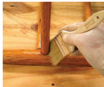
Removing. Use a cloth to remove the excess gel varnish before it begins to harden, which it does much faster than liquid varnish. To aid in getting the varnish out of recesses and inside corners, use a dry brush as I'm doing here.
