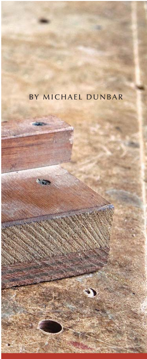
Common parts. This “joint-and-square” shooting board shows the three parts common to every iteration: the base, platform and stop.
