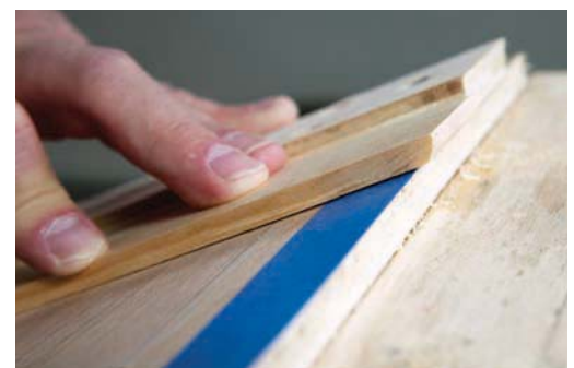
Tape trick. You can increase your board's precision by using a strip of painter's tape to lift (as shown) or lower the angle.
