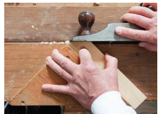
Perfect miters. The miter shooting board is used for truing and adjusting miters.
