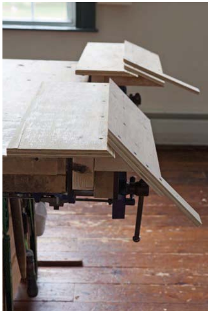
Donkey's ear. A 45° donkey's ear is used to trim standing miters and edges. For coopered work, make a board at another angle. The one on the right is 22½° and makes an octagonal form.
