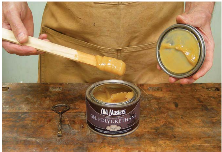
Thickness. Gel varnish is thick in the can, but it spreads easily because of its thixotropic quality.
