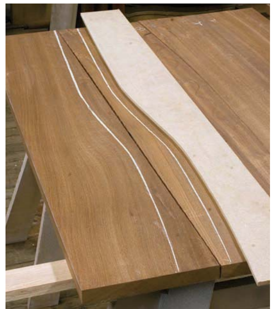
Double duty. The master pattern lays out a curve common to both boards.
