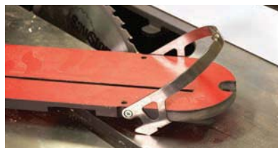
Locked out. The throat insert lock – lift the bail handle – is outstanding. But a shop-made replacement seems out of the picture and $39 is a lot to pay when you need a replacement.
