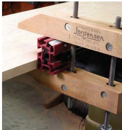
More jigs. Again faced with secure workholding problems at the table saw, I used a handscrew attached to the sliding table to support one end, and an stepoff block at the other to safely locate the groove for the bottom fixed shelf.
