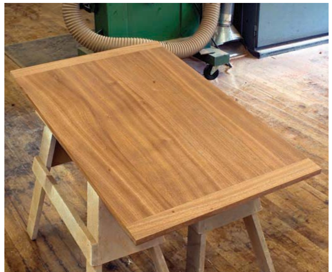
Unseen seams. Free from harsh colliding seams and abrupt changes in color, the completed top presents a clean and harmonious panel.
