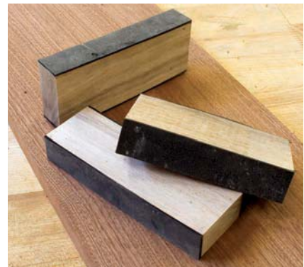
Careful clamping. Rubber-padded cauls are used to prevent clamp marks on routed edges.
