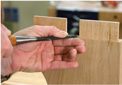
Split tenon. A 6 \frac{1}{2} "-wide tenon is too big, so I split it using a coping saw then chiseled out the remainder of the waste.
