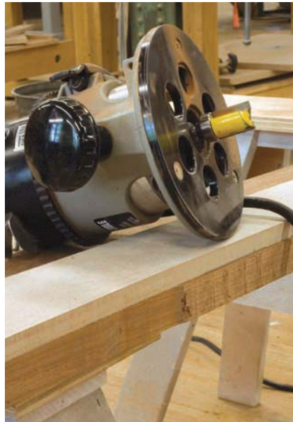
Size does matter. A \frac{3}{4} "-diameter flush-trim bit is perfect for trimming the workpiece edge flush to the curved pattern.
