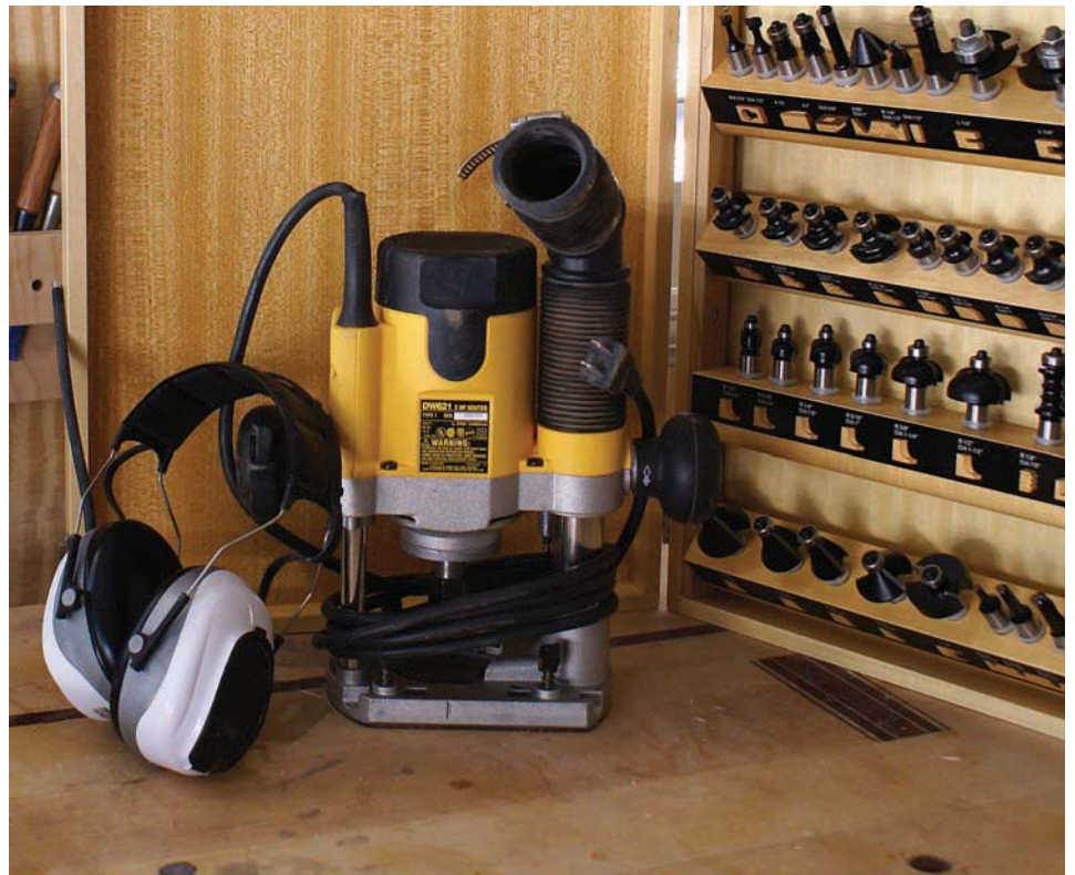
Bit arsenal. If you do a lot of routing, you'll surely build up a large collection of bits in a short time. Keep them neatly organized and clean, and they'll always be ready for the routing job at hand.
