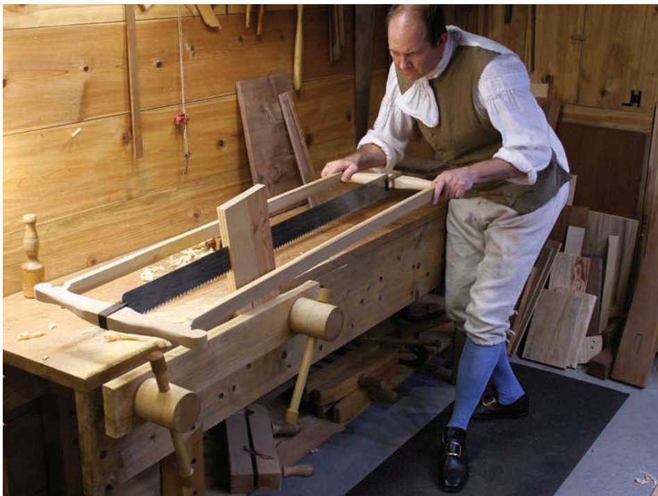
Not so hard. Despite the look of despair on my face, this saw is pretty easy to use. The problem I’ve had is controlling it! The tool is a reproduction of one depicted by Roubo dating from the 1760s. Its blade is 4' long and features two teeth per inch. It’s difficult to start but cuts aggressively once the kerf is established.
