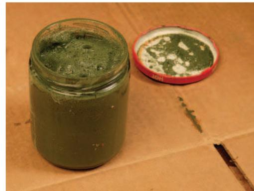
**Shaken, not stirred.** Simply put the lid on the jar and shake it for about a minute. The paint will be frothy at first; let it sit for an hour before applying.
