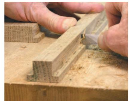
**Run in reverse.** The back of a chisel makes a great scraper, just the ticket for cleaning out the corner of rabbets.
