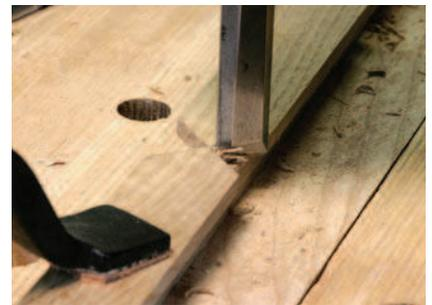
**Cutting corners.** The router will leave material in the corner, which can be removed with a chisel. The finished edges of the joint have been established with the knife and saw.
