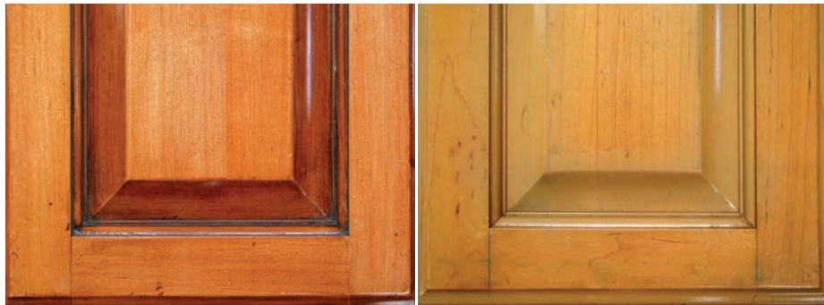
Glazing and toning. Both of these processes are a way to add color over sealed wood. Glazing (on the left) involves applying and manipulating a thick-pigmented stain; toning (on the right) is a thinned and lightly colored (pigment or dye) sprayed finish.
