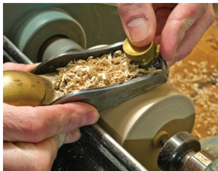
Eschew the skew. A low-angle block plane makes short work of producing an accurately sized cylindrical form.
