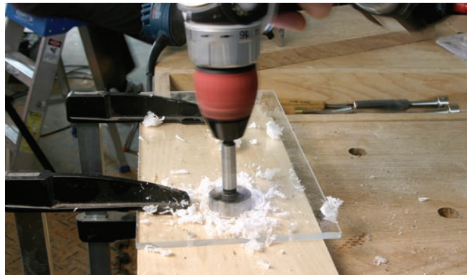
Big bit, same story. The larger bit clearance hole can be cut with a spade bit or a Forstner bit. A drill press is nice, but not necessary.
