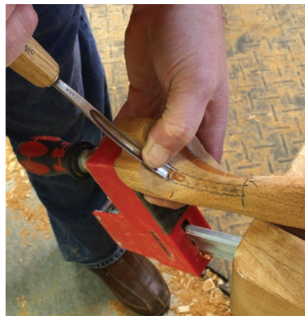
Crooked tool, not crooked lines. A bent gouge provides leverage as you carve the flutes. And the curved portion closely matches the roll from the foot to the ankle.
