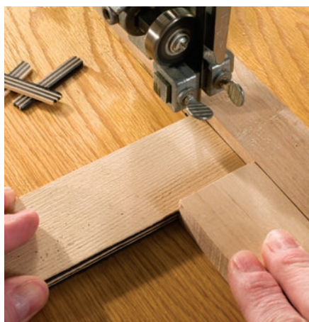
Keep a light touch. Hand placement and feed pressure are the keys to accurate sawing.
