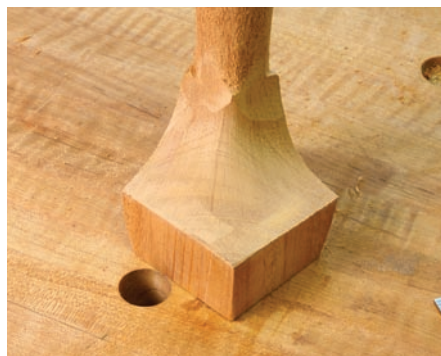
A place for power. Hand tools could shape the top of the foot, but you'll spend a lot of time working the end grain. A spindle sander quickens the work as you roll the area into the ankle.
