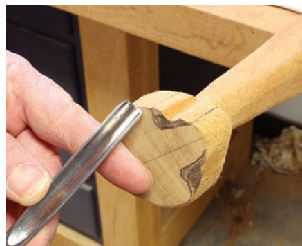
This little piggy. A carving gouge allows you to easily form the trifid toes. A round file is another option.
