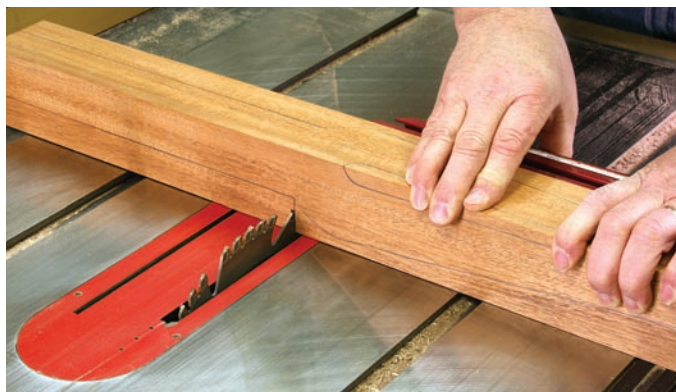
A defining time. Set the blade height to reach the post block and cut to define the knee/post intersection. Rotate the piece 90° and cut again to define the second face.
