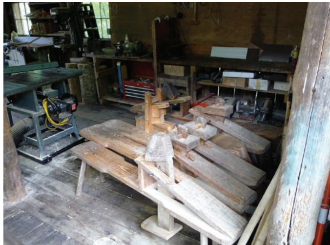
Old-world and new. An array of shaving horses for students' use rest alongside the familiar table saw.
