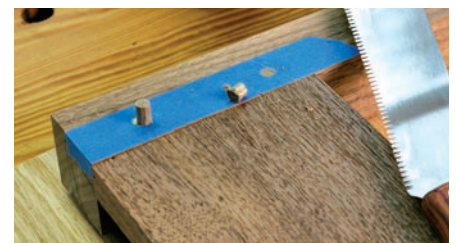
An error barrier. A strip of painter's tape can protect your finished work from glue squeeze-out and from the teeth of the saw. After you cut the peg flush, remove the tape.
