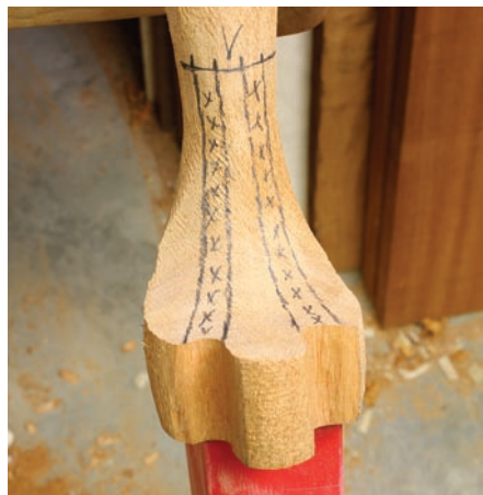
Best by eye. Layout of the flute area is key. Bending a straightedge into the curve just doesn't work – the lines appear bent. The best way to get a pleasing layout is to rely on your eye.
