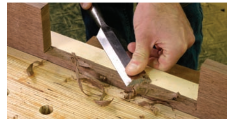
Chisel it clean. To clean up the bottom of the drawer opening, clamp a guide to the apron and use a chisel with its flat face against the guide. Skew the tool to shear the wood and you'll find the work quite easy.
