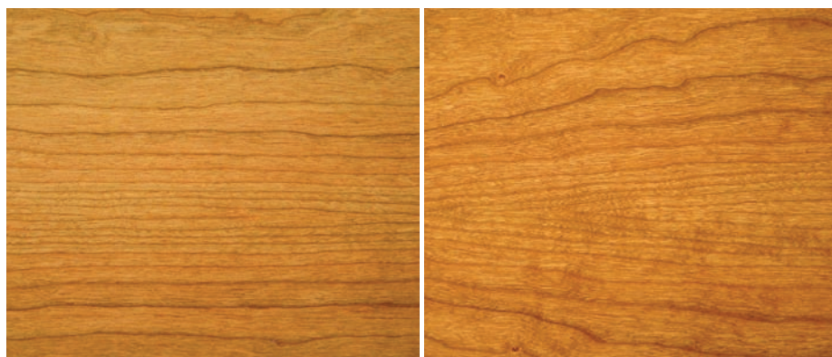
Oil vs. water. Oil- and water-based polyurethane look very different on wood. Water-based polyurethane (left panel) adds no color to the cherry. Oil-based polyurethane (right panel) adds a warmer yellow/orange coloring.
