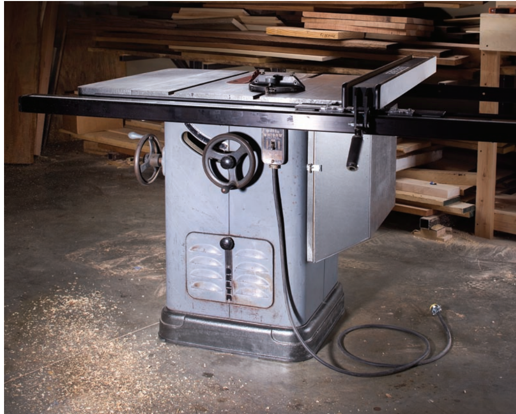
The refurbished 1944 Unisaw is ready for another 50 years of service. The labor of love included new arbor and motor bearings, a thorough cleaning, some paint and rewiring, among other chores. The original fence was upgraded to a modern Biesemeyer model.
