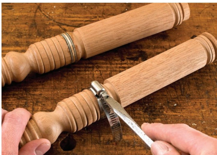
Doing the impossible. Bending a wide satinwood banding to a tight radius would be quite difficult. But formed as a circle, installation is easy.
