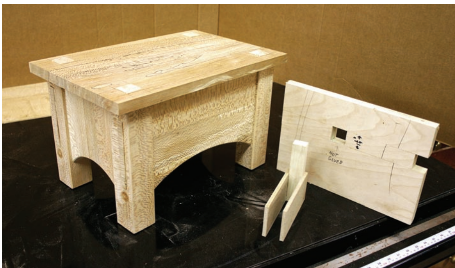
Head of the class. Here is the completed stool with the four through-tenons and the two simple jigs that make it so easy.
