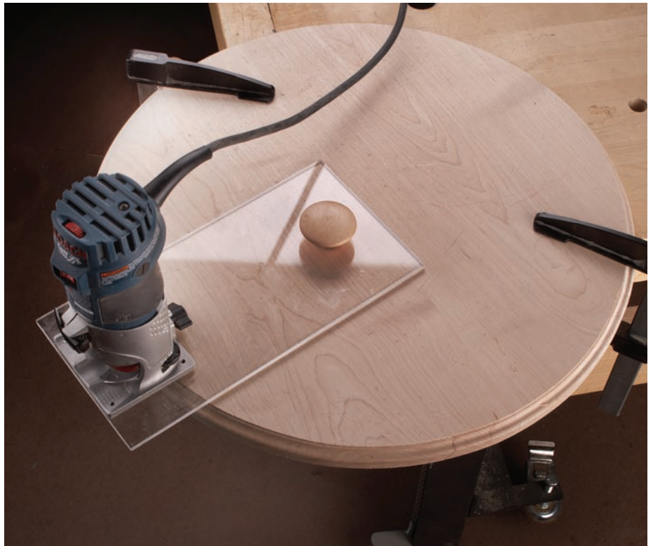
Quick fix. A custom-made baseplate provides a solid base for routing edges.
