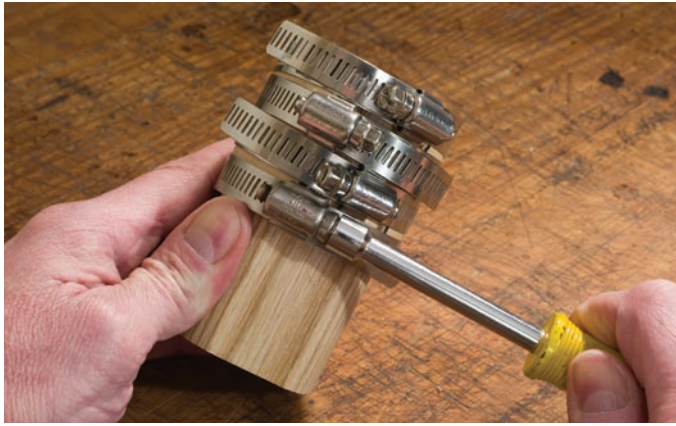
Who would have thought? Hose clamps from a hardware store supply all the clamping pressure you need – and then some.
