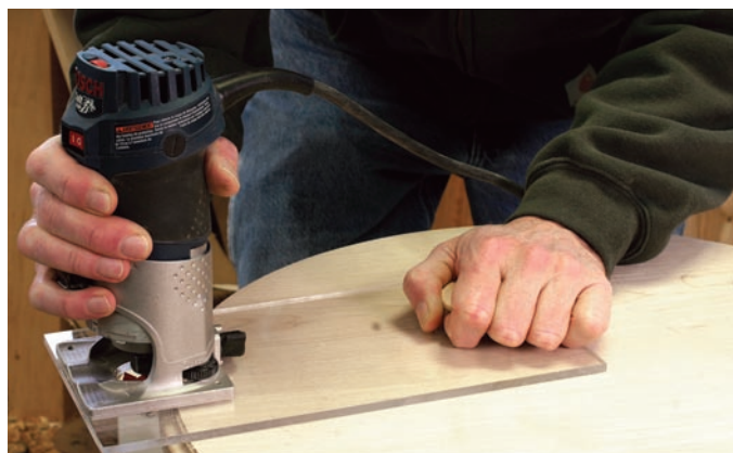
The solution. The extended base provides better control, eliminating the tendency of the router to tilt.
