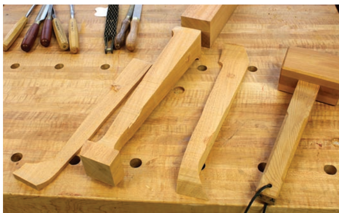
All squared up. After the band saw operations are complete, knock the reattached pieces from the blank to expose the ready-to-shape cabriole leg.
