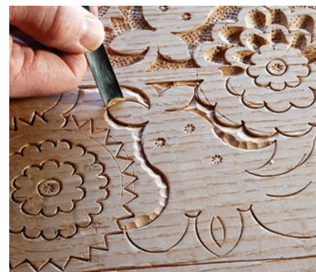
Carving. Carved decoration is ubiquitous on 17th-century pieces, so we know the joiners had a set of carving gouges and mallets, also compasses, a square and an awl.
