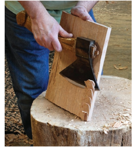
Hewing. Riven boards were further refined in thickness by hewing them with a hatchet. The tool marks are quite evident on period furniture.
