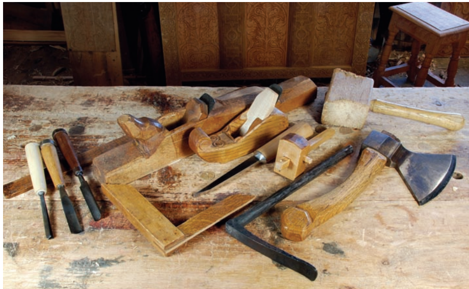
A typical kit? The few surviving period tool inventories don't tell the entire story, but here's what I think of as the core of a typical joiner's tool kit in the 1600s (clockwise from left): a set of gouges, a fore plane, smoothing plane, a mortise chisel, marking gauge and mallet, a hatchet, a holdfast and a square.
