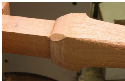
Soften the knee. The top of the knee is also rounded. Rasp a 45^\circ angle then transition the sides for a smoothed profile.
