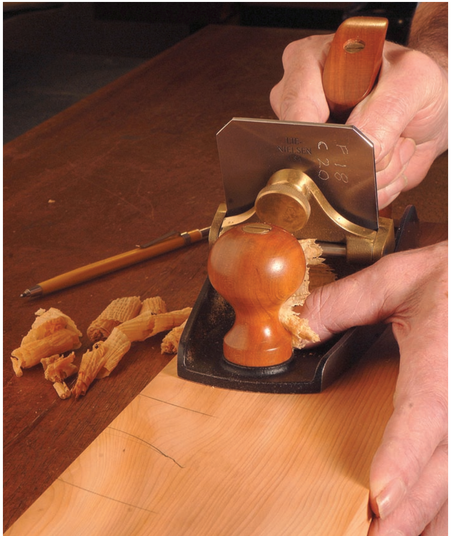
Getting you out of a bad scrape. Scraper planes are able to conquer unruly grain and maintain a flat surface. They are also ideal for dealing with veneer.
