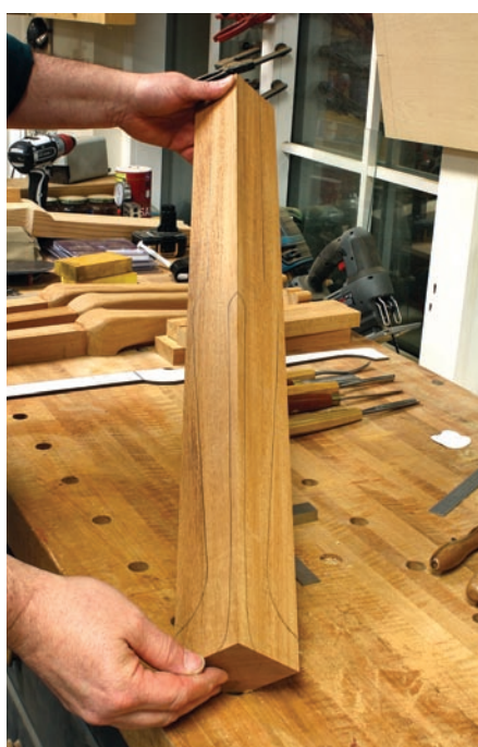
Proper layout. Keep the back edges of the pattern together for a properly sized post block and leg profile.
