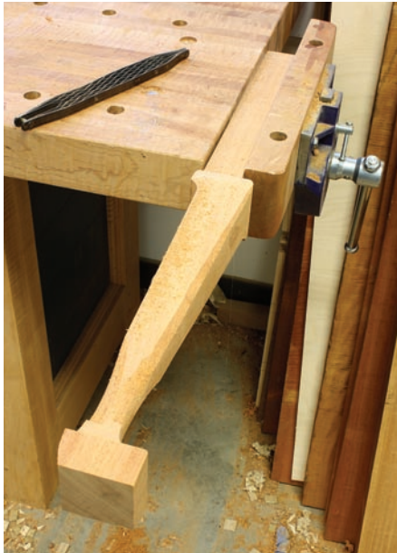
Shaping begins. After you establish a round ankle, shape the sharp corners of the leg for a smooth transition. Flatten the corners, then round the edges.
