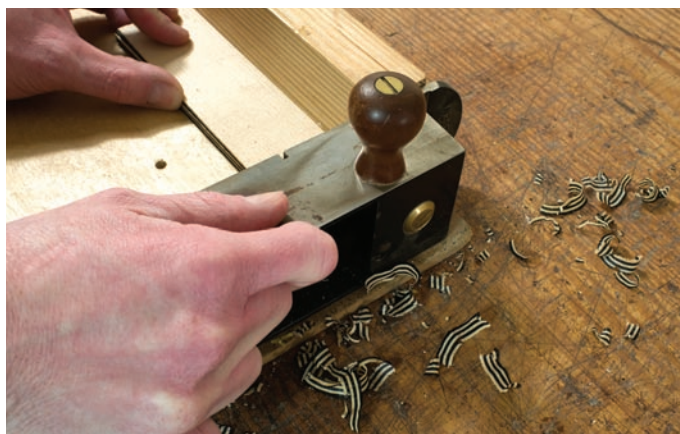
True your end. After a few strips are cut, you need to square up the ends of the stack at your shooting board.
