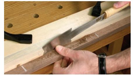
Dive to the bottom. An azebiki nokogiri is a Japanese saw with curved cutting blades (one for rips; the other for crosscuts). Used against a guide, you can start your cut in the middle of the apron and plunge through. This releases the drawer front from the apron.
