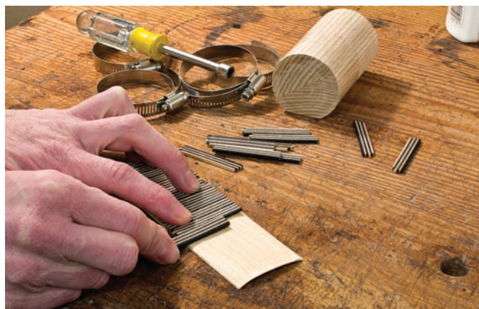
Work fast. Once the glue is brushed on, it starts to curl the veneer, making assembly frustrating.
