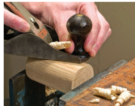
Keep it safe. A flat is planed on the form to provide stability as the inlay is later sawn at a band saw.
