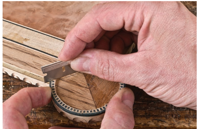
The eyes have it. Where the curved inlay meets the straight run of inlay, mitered corners are best done by eye.
