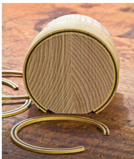
Doing the impossible. Bending a wide satinwood banding to a tight radius would be quite difficult. But formed as a circle, installation is easy.
