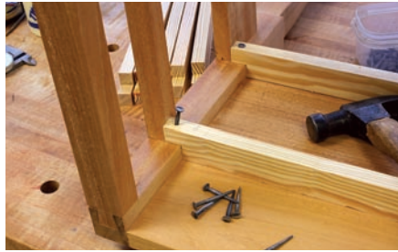
Nailed in place. A pilot hole helps to prevent a split in the runners as the nails are driven.
