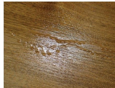
Reflected light. Always check for developing problems in a reflected light.
