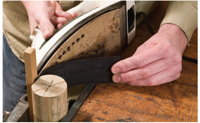
Tailor-made veneer. Using moisture and heat to bend the outer layer of black veneer is as easy as pressing a collar.
