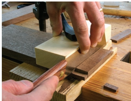
A cheat from the East. To cut the tenons' face shoulders you can use a scrap of wood to guide a flush-cutting saw. Just make sure the saw has no set and you've clamped the guide right on your knifed-in shoulder line.
