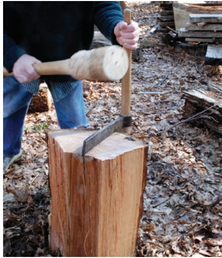
Riving. Panels were riven, or split, from logs using wedges and a "beetle," then a froe struck with a club as shown above.
