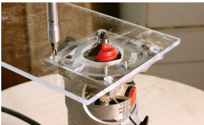
On the level. Countersink the holes so the screws are below the plate surface. You may need to make a trip to the hardware store for longer screws.
