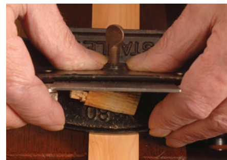
A good grip. Control the No. 80 with your thumbs and forefingers. The pressure you apply is much like planing a board.
