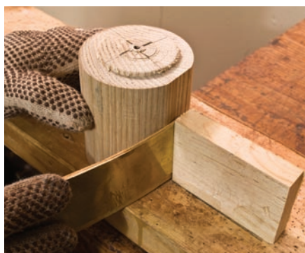
Back-up plan. A thin piece of shim stock compresses the wood fibers and takes the pressure off as you bend the inlay.
