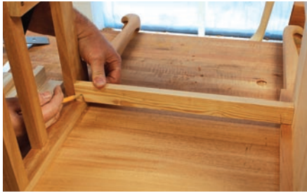
Easy, peasy. Mark the notches for the runners right off the case. It's precise and trouble-free.
