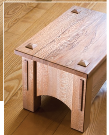
Arts & Crafts hallmark. Four through-tenons in a single board is a joinery challenge. The small stool at right is a great way to practice with the two simple jigs and careful work needed to meet the challenge.
