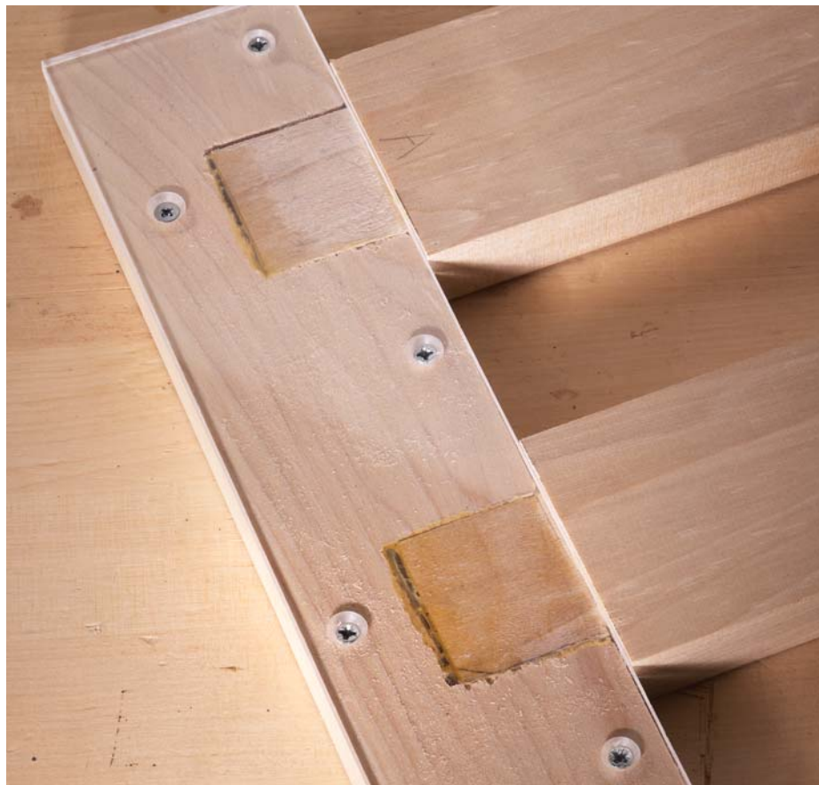
How – not how much. Roughly equal amounts of glue were used in each of these joints. The difference between them is in how the glue was applied.
