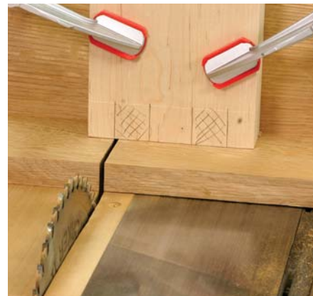
L of a solution. A simple jig attached to the table saw's miter gauge supports the work and indicates the exact line of the cut.
