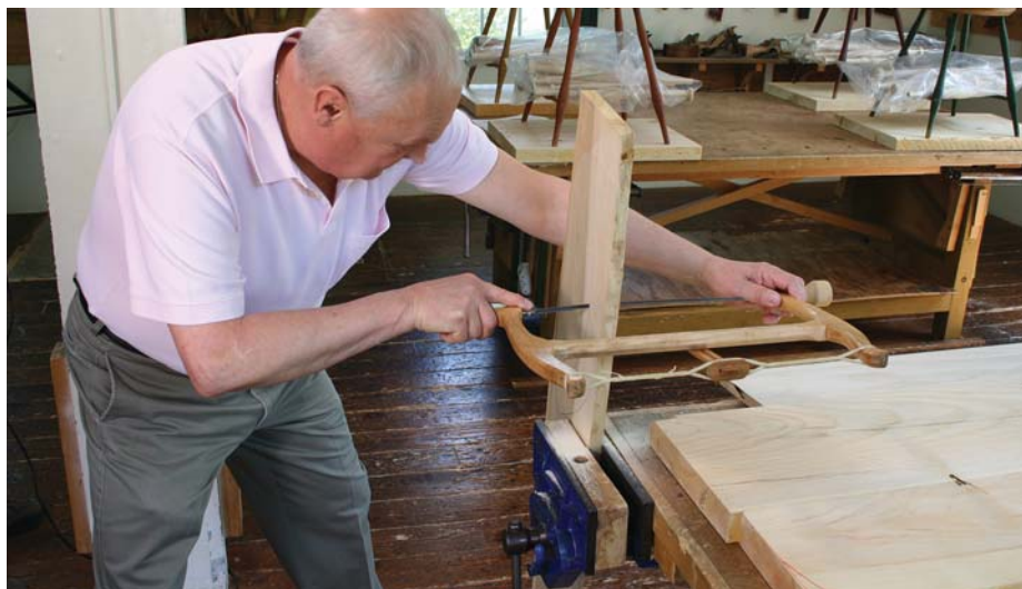
Armed with a small saw. When using the small bowsaw, move your arms in a reciprocating fashion. Keep your torso steady.
