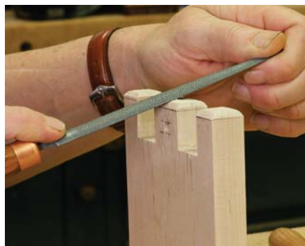
Cutting corners. Mark where the end of the drawer side intersects the fingers on the drawer front. Round over the edges to the pencil line.
