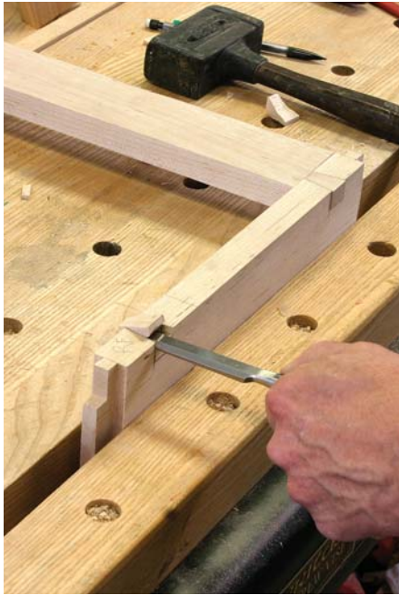
No-spread zone. A single through-dovetail on each of the top rails locks the sides of the case together and adds an attractive detail.
