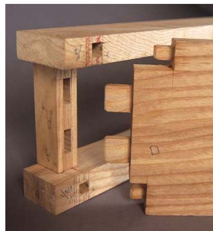
Four-pronged support. The end rails of the drawer frame not only attach to the dividers with mortise and tenons, the ends are notched to fit around the top and bottom pieces and the rail is tenoned into those pieces for additional support.
