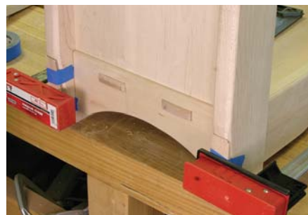
Tape for the tapers. Offcuts from tapering the legs are taped in place to provide a flat surface for the clamps.
