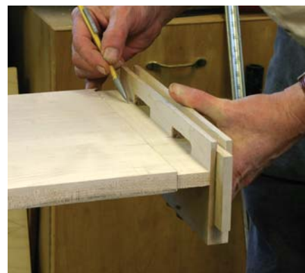
Where it belongs. Marking the tenons directly from the mortises is faster and far more accurate than measuring.
