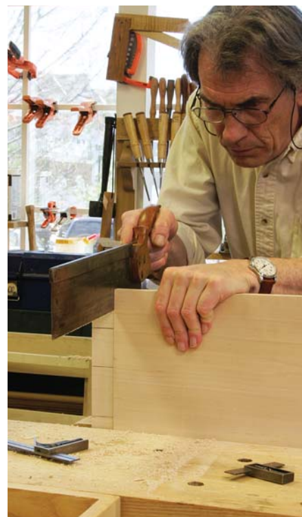
Easier by hand. These cuts could be made at the table saw, but that would be an awkward operation. Cutting the tenons by hand allows me to see what is going on.
