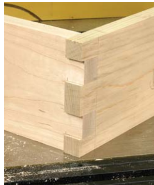
Easy now. The two parts should slide together easily – but without any slop. If it's too tight, file the fat fingers.
