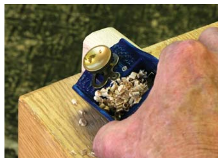
Big mouth, quick work. This side of the plane will take a coarse cut, removing a lot of material in a hurry.
