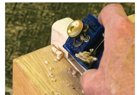
Fine on this side. The other side of the plane takes a small finishing cut. The amount of material removed and the quality of cut is controlled by moving the plane laterally.
