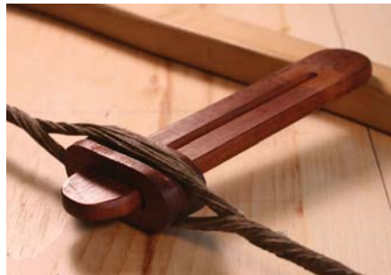
How to avoid the crack. A toggle such as this allows you to adjust the frame's tension by half-turns, which is better for the saw.
