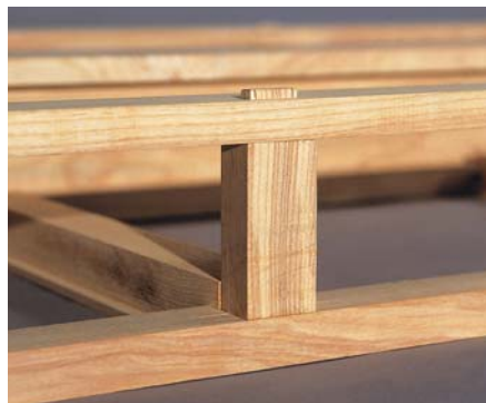
Long-lasting joinery. The center dividers join the rails with wedged mortise-and-tenon joints. The top tenon, to be pared flush after the wedges are installed, extends above the rail while the bottom tenon is blind wedged – a technical joint that is as strong as a tree.
