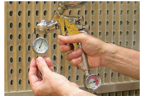
Pressure gauges. Optimizing can also be done using a pressure gauge attached to the air-inlet nipple at the bottom of the gun's handle, but no advantage is gained over simply using the regulator. To determine if you are complying with the HVLP standard of not exceeding 10 PSI at the air cap, you will need a special air cap and attached air pressure gauge.
