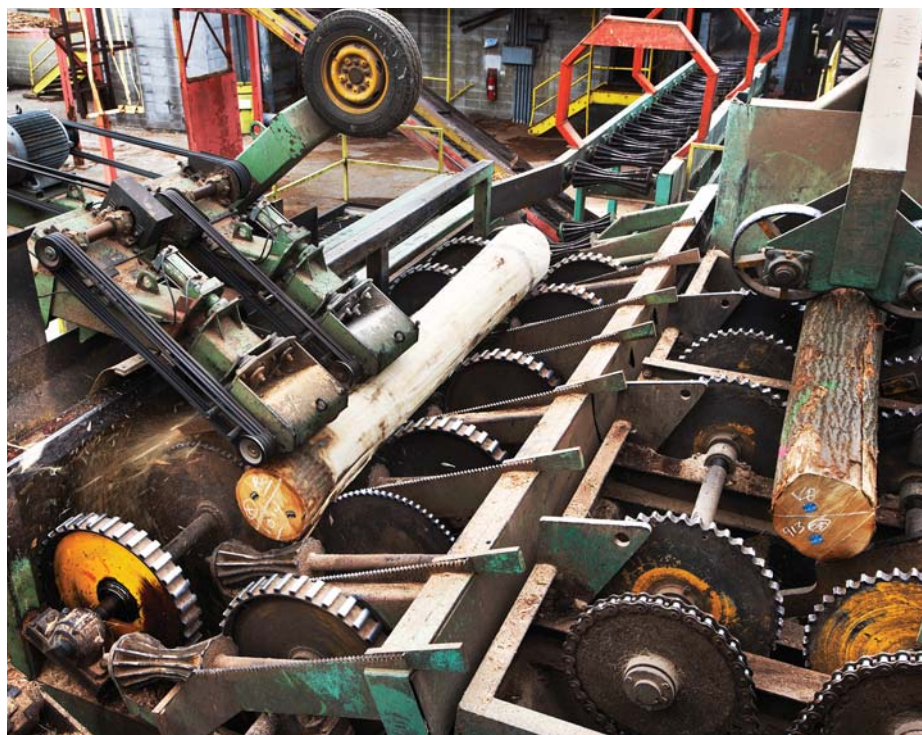
Ground to round. Within about a minute, this machine can strip the bark off a full-size log and get it ready for slicing on an enormous band saw mill.
