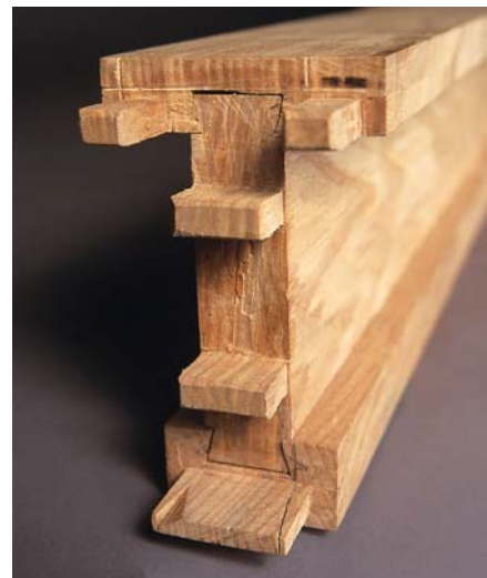
Built for strength. Three pieces stack to make up the center rail. The top piece has twin tenons, the middle piece has two tenons that stack vertically and the bottom piece has only one tenon, and that single tenon is blind-wedged.
