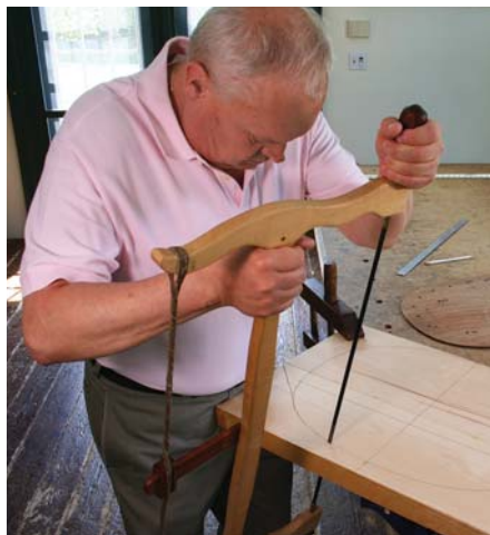
Rip away. When you are ripping with the large saw, tilt the frame away from you slightly to help stay on your line.
