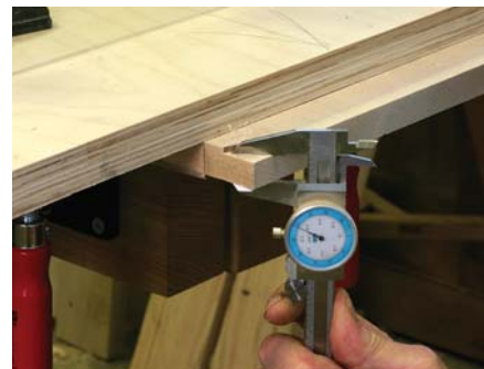
Knowledge is power. Measuring with calipers reveals the exact thickness of the tenon and how far to set the depth of the router bit.
