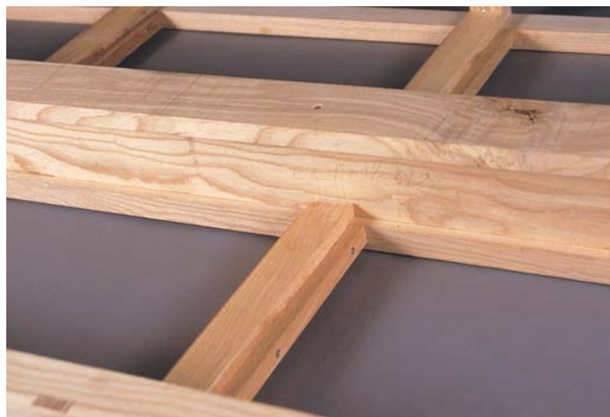
It's an easy fix. Because drawer runners receive a good deal of wear, it is advisable to allow for simple replacement. The runners are held to a support with stainless steel screws, no glue.
