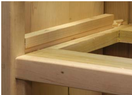
Adjustable guide. The drawer guides are glued to the web frame. The short length and rabbeted bottom edge provide room to adjust the width with a block plane.
