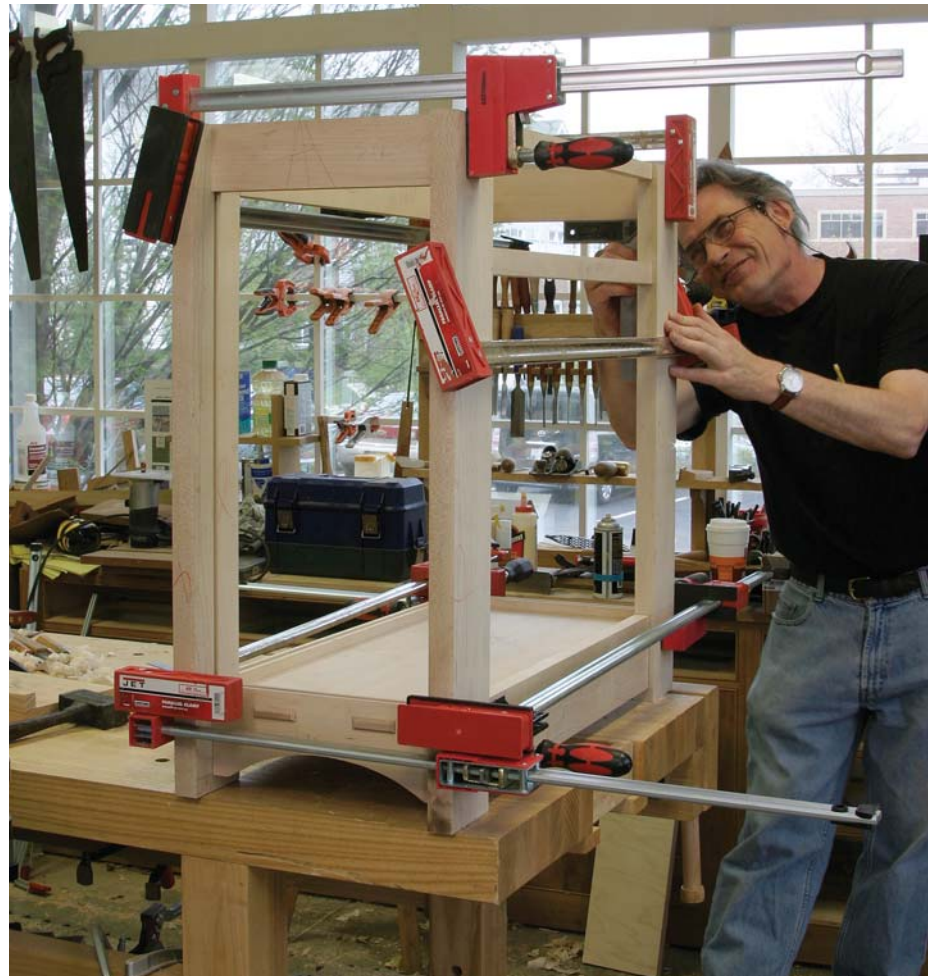
Dry-fit now, panels later. The only way to know if things will really fit is to put the carcass together. The panels will be added the next time around.
