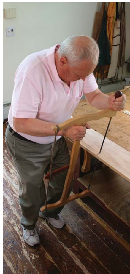
Use your whole body. When using the large saw like this, don't use only your arms. Use the mass of your body to help bring the saw down. Flex your knees and bend slightly at the waist.
