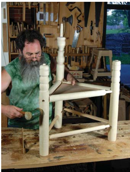
Test-fit. Each rectangular tenon is fully seated in its mortise. Here, I'm holding the seat in place in its grooves as I pound home the round tenons for a dry-fit.
