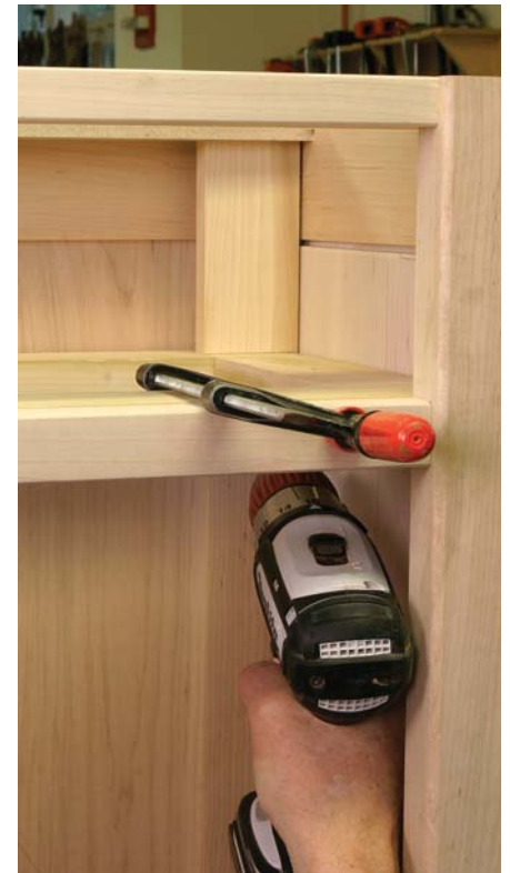
Simple fix. A pocket screw at each end attaches the drawer frame to the inside of the back legs.
