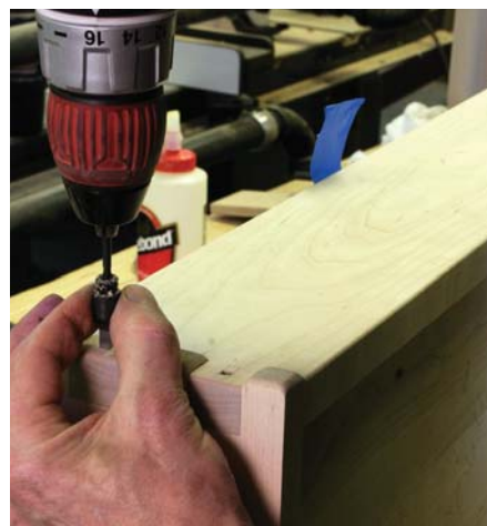
Waste removal: Follow with a drill through the hole in the punch body. This removes the waste within the square recess.
