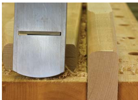
Why this slides. Opening the mouth of the block plane provides room to skew the iron.
