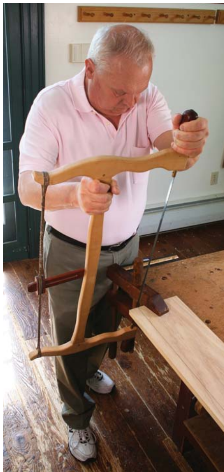
Get a grip. When ripping, grasp the strut with one hand and the handle with the other. Begin your kerf with the lower part of the blade engaged in the wood.
