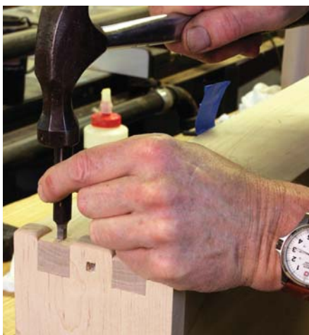
One-two punch. Locate the punch and smack it a couple times with a hammer. This cuts sharp corners and straight sides for the plug hole.
