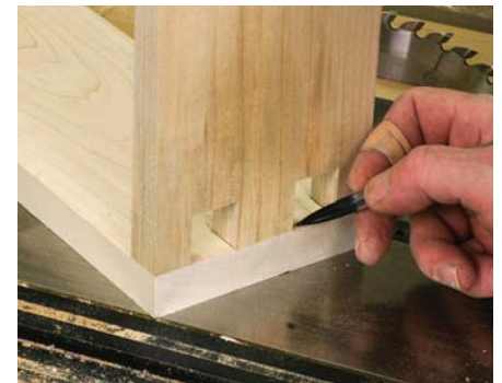
Balancing act. After cutting the first set of fingers, place the end of a side on the drawer front to mark the matching parts of the joint.
