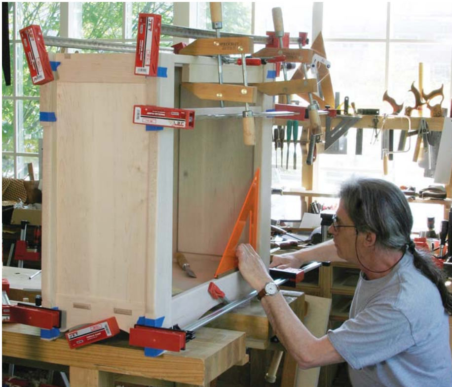
Sliding home. Start all the mortises and get the parts close with a rubber mallet. A few clamps close the joints side to side.
