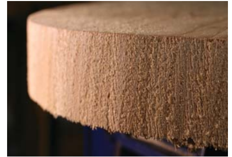
It tracks tightly. While the surface from a bowsaw might be rough, I find a bowsaw is easier to keep from drifting off line than a band saw.
