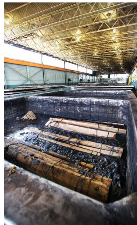
Primordial pool. These deep pools of hot water soak the logs to soften the wood for slicing. The smell is surprisingly powerful, like a primeval swamp.
