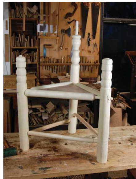
Staggering. While the seat rails are all on the same plane, the stretchers are not. So fitting both the top and bottom of the chair simultaneously can be a challenge (and don't forget to hold the seat panel in place, too).
