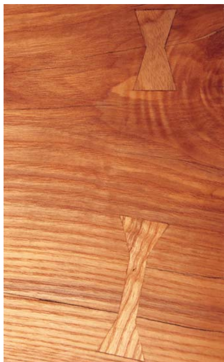
Old-school fix. Any small hairline cracks in the tabletop are bridged with inlaid butterflies. On the bottom face of the tabletop, we use a matching hardwood, but any splits in the top face are fixed with a contrasting wood. (We used purple heart.)
