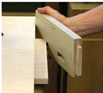
When to stop. When a corner can be forced into the mortise, the thickness is close. Then it's time to cut the edges of the tenons.
