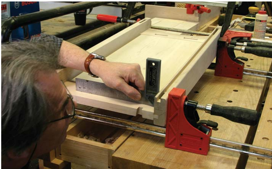
E pluribus unum. Subassemblies minimize the number of pieces to contend with during the final assembly. After clamping, check to see that they are square.
