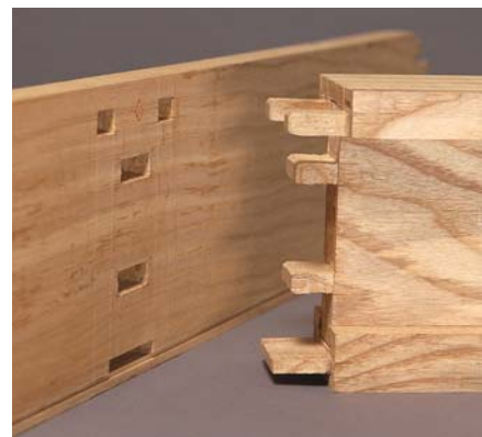
Great grasp. A properly fit mortise-and-tenon joint is very strong. The center-rail-to-end-rail joinery has five such joints.
