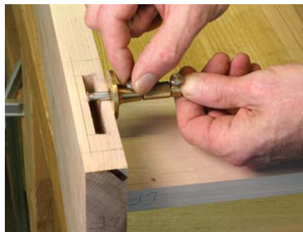
Better than numbers. Setting the marking gauge directly to the edge of the mortise ensures exact alignment of the rail and leg.
