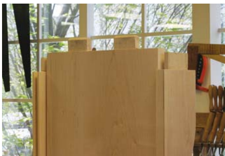
Where bottom and side collide. This isn't as hard as it looks; the side will be one piece, and trial runs ensure that everything fits.
