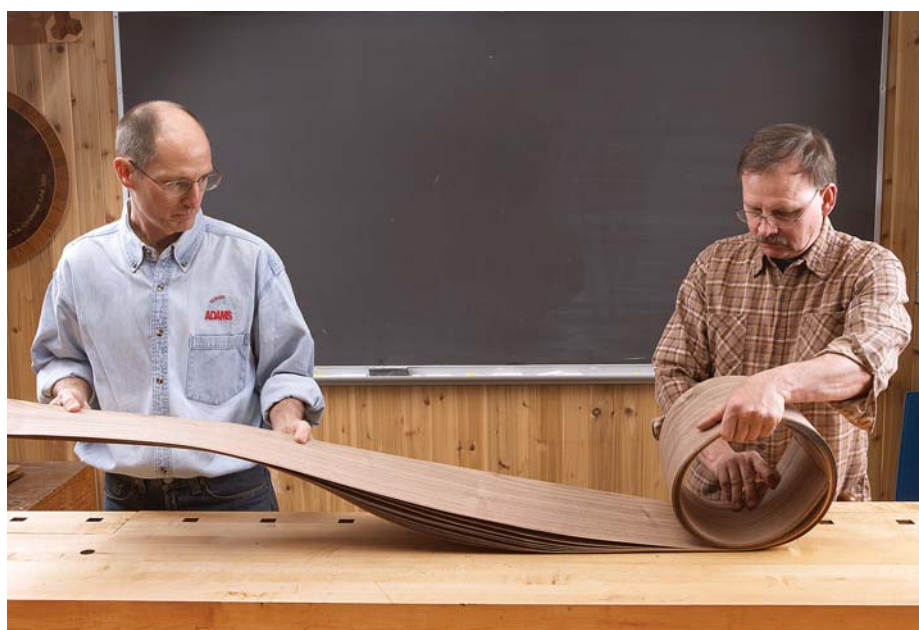
Unroll and use. Veneer typically comes rolled up or flat. If it's rolled, you should unroll it as soon as you can. Here Zane Powell (right) gives the author a hand with some walnut veneer.
