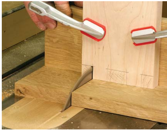
Hold the line. Place the pencil line next to the kerf in the guide to cut just inside the line.
