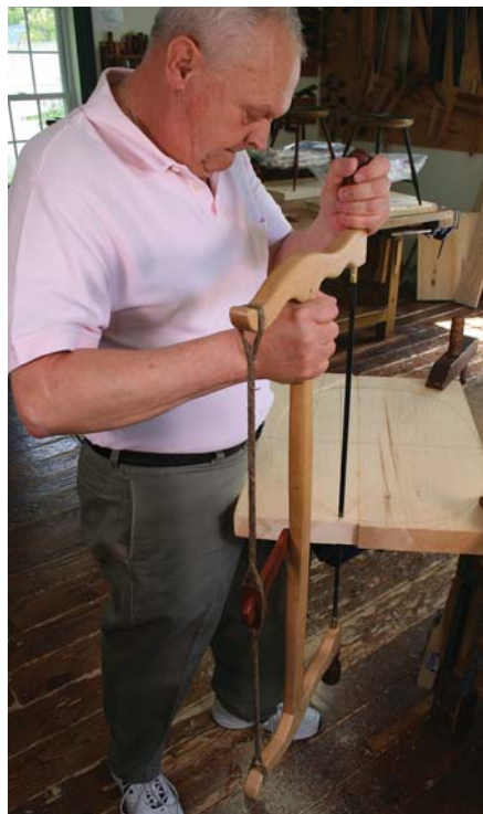
Straight through the curves. When you turn a corner, bring the frame up until it's vertical, which prevents the edge from becoming beveled.
