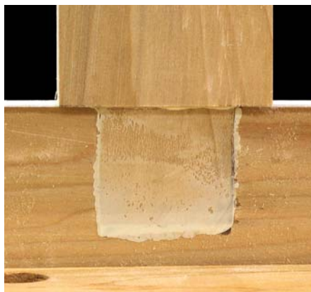
All wet. When a joint is first assembled, the glue spreads into any available space, whether it was brushed or not, as shown here in our first of several tests.
