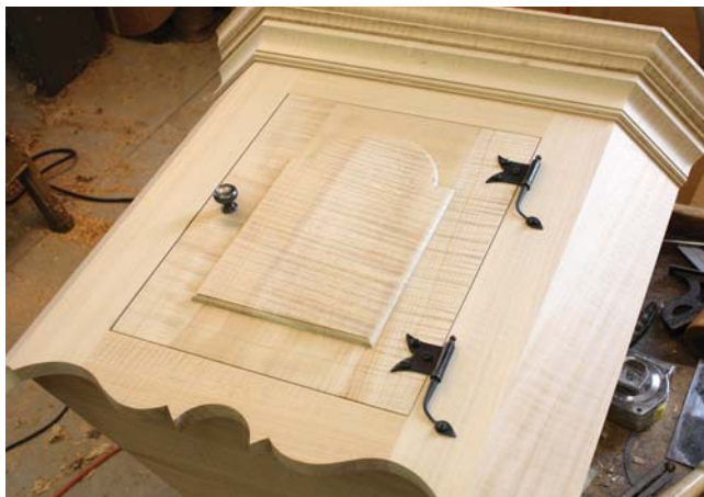
A tight curve. The groove for the inside edge of the upper door stile is cut with the same slot cutter used on the tombstone panel.
