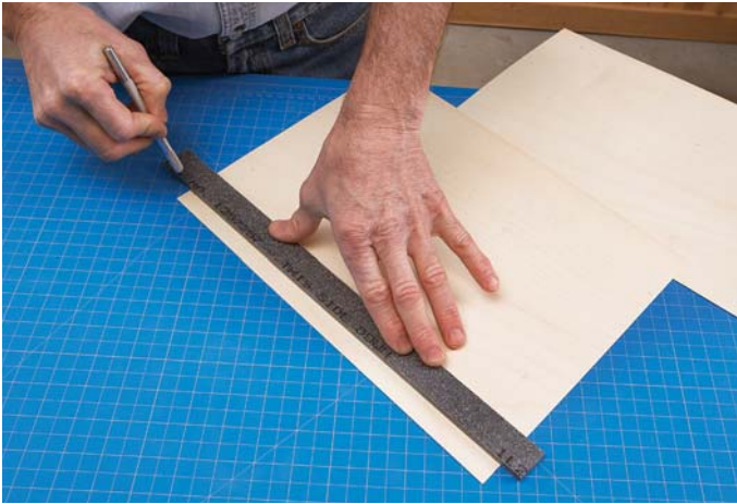
Essential tools. A self-healing cutting mat, an X-Acto knife and a shop-made straightedge can perform many cutting chores.
