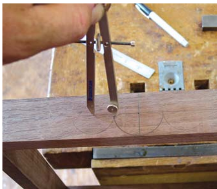
Series of circles. Lay in the center drop with a compass set at \frac{7}{8} ", then scribe the first half of the cyma curve using a compass set at \frac{3}{4} ".
