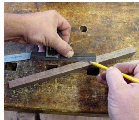
Jagged layout. Scribe a centerline down the edge of your sawtooth leg, mark the \frac{3}{4} " vertical divisions, then use a straightedge to lay in the angles.
