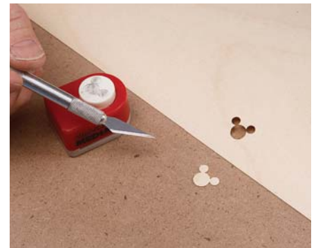
Feeling punchy? You will be surprised what you can do with veneer and a paper punch. It makes both the hole and the piece to inlay.
