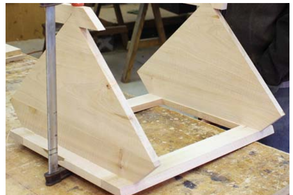
Caul me. A V-notch cut into a scrap makes a perfect caul for clamping the odd-shaped top and bottom.
