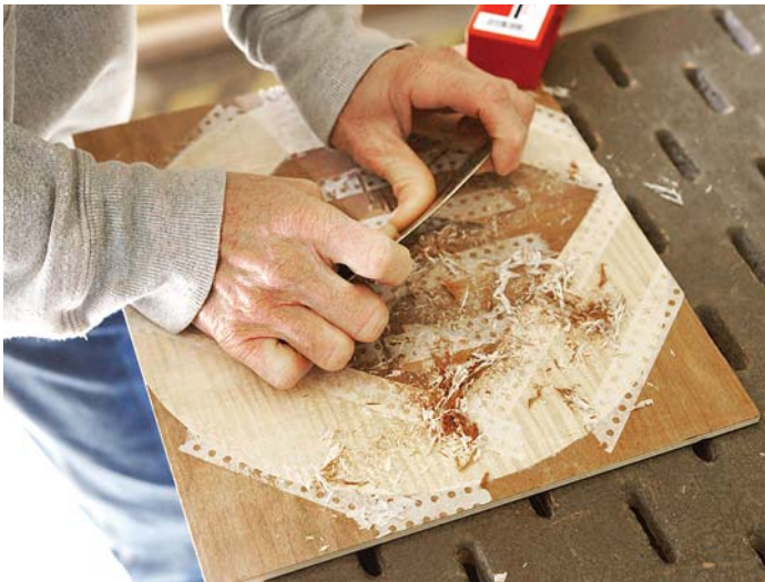
First scrape. Remove most of the veneer tape using a scraper, then sand the remainder using a random-orbit sander.
