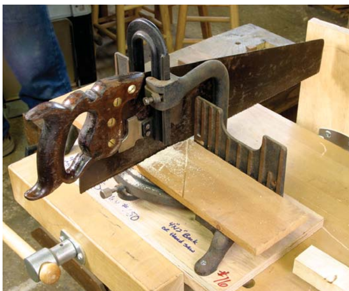
Open-front box. Here's a Stanley No. 150 equipped with a panel saw. These are superior to simple miter boxes and have a huge crosscutting capacity.
