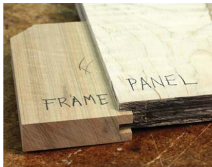
A proud panel. This mockup of the door panel construction shows how the panel is held in the door frame groove yet overlays the face of the door.
