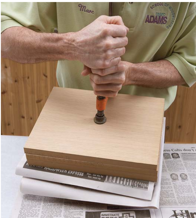
Start at the center. When clamping up veneer using a particleboard sandwich (as shown), begin by applying one clamp to the middle of the stack.
