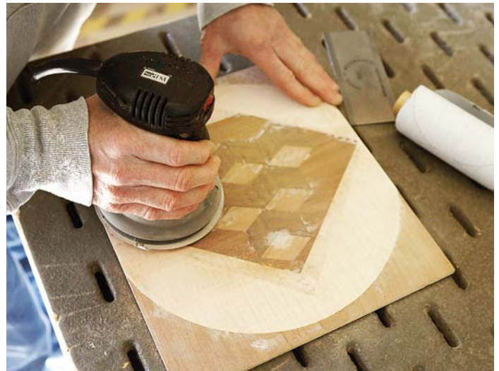
First scrape. Remove most of the veneer tape using a scraper, then sand the remainder using a random-orbit sander.
