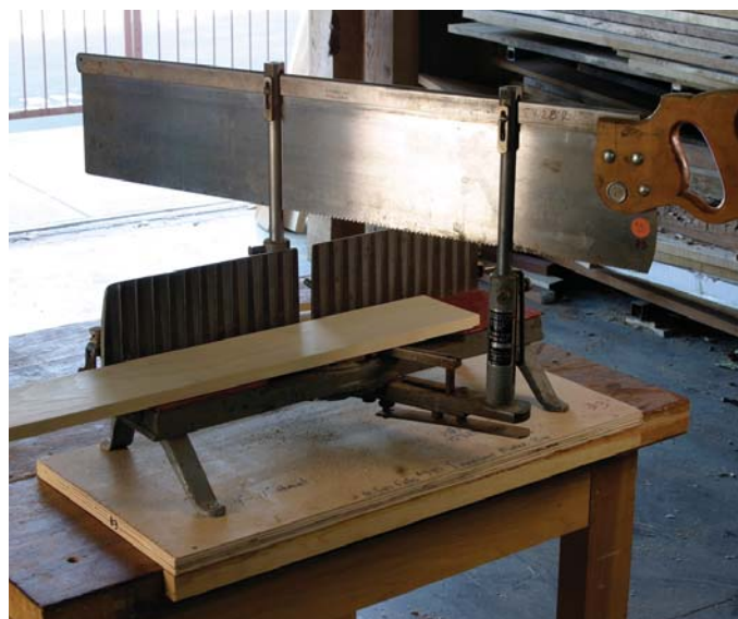
The full enchilada. This fully framed Millers Falls miter box has all the bells and whistles, including a system to hold the blade locked above your work when you're not using it. This is the most accurate style of box.
