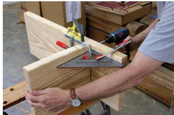
Square to start. Square subassemblies will make the overall structure easier to put together.
