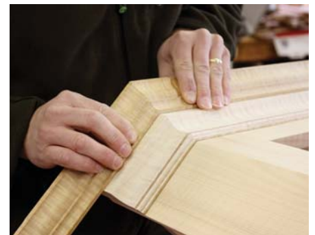
Many happy returns. When running mouldings around a cabinet, it is easier to begin at the front. Install the center piece first, then fit the returns to it.
