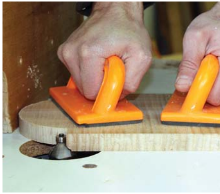
Go on, bead it. A \frac{1}{4} " roundover bit is used to rout the bead and fillet on the tombstone panel.
