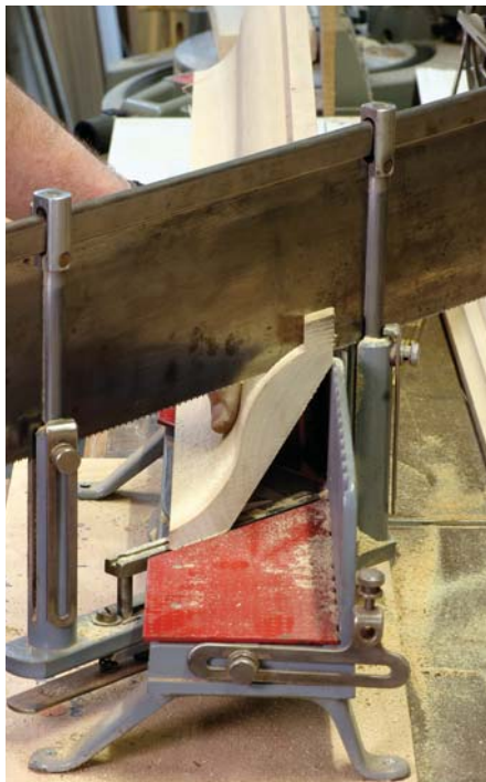
Open wide. Miter boxes can have an enormous capacity. And their cuts are unmatched for accuracy and safety.
