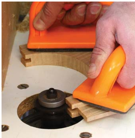
A tight curve. The groove for the inside edge of the upper door stile is cut with the same slot cutter used on the tombstone panel.
