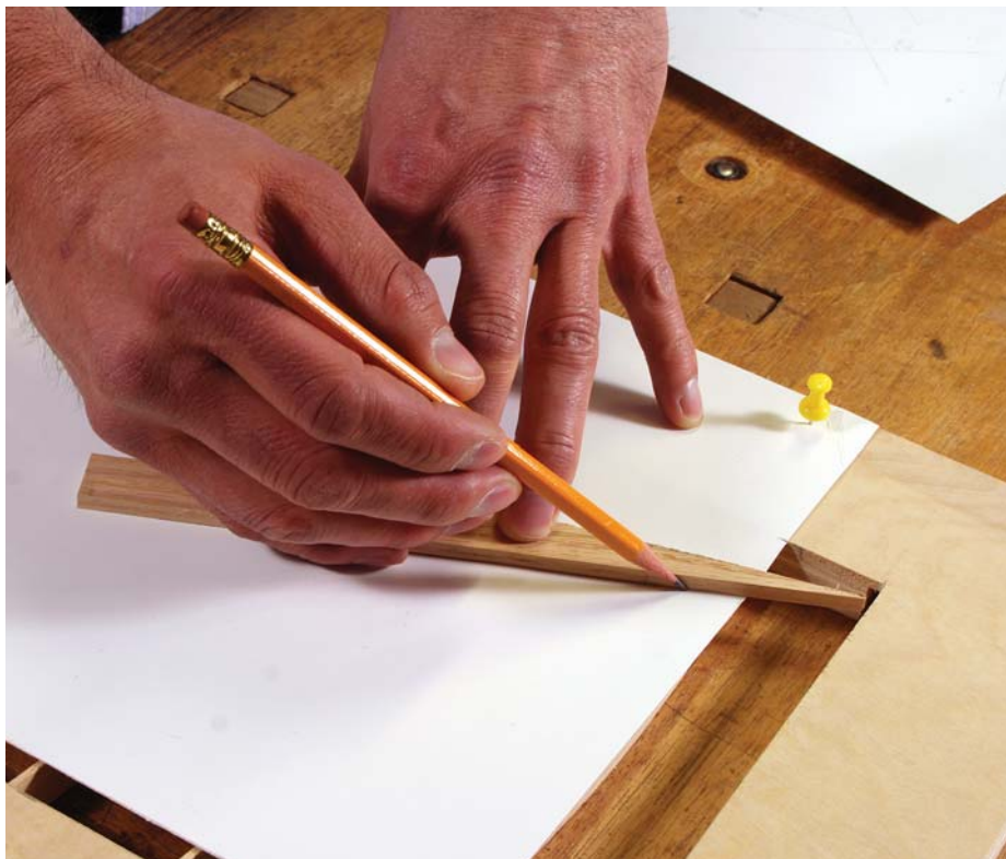
This is a ticking stick. In the past, many carpenters used ticking sticks to fit built-ins into irregular spaces in a house. You can apply the same principles to fit doors to face frames.
