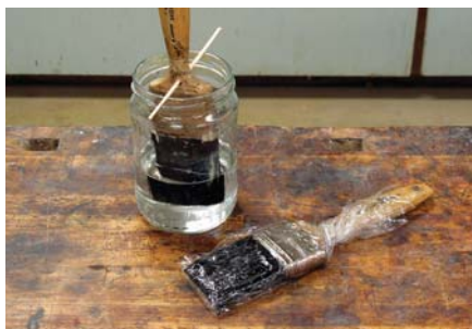
Brush storage. There's no need to clean your brush between coats unless you expect a lot of time to elapse. Store your brush by wrapping it in plastic wrap or hang it in a jar of mineral spirits.
