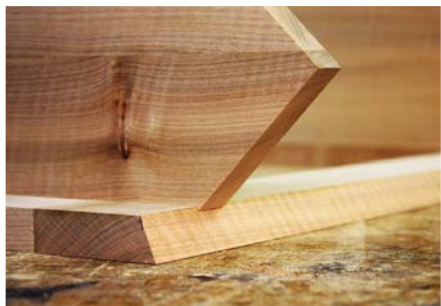
A careful layout. The cabinet top and bottom are centered left to right in the dados then each corner is marked at the bottom of the dado. The sides of the face frame are then mitered away from these layout lines. The top and bottom can now be glued in place.
