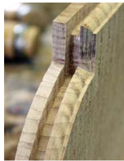
It's an inside job. Because neither the roundover bit nor the slot cutter used to rout the groove around the panel arch is capable of cutting an inside corner, both of these areas must be finished by hand.
