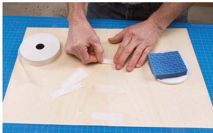
Licked and sealed. Veneer tape is activated by moisture and is used on the show face. First tape across the joint.
