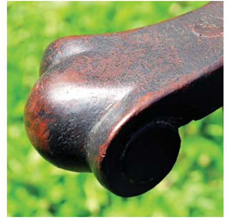
Your hand was here. Applying this wear over the entire piece would be wrong. This burnished sort of rub-through occurs where your hands rest.
