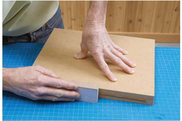
Edge repairs. You can fix or true the edge of veneer by sandwiching it between pieces of MDF and using a sanding block to remove damaged fibers.
