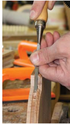
A fitting cut. The inside corner of the panel is shaped to fit around the arched upper door stile.
