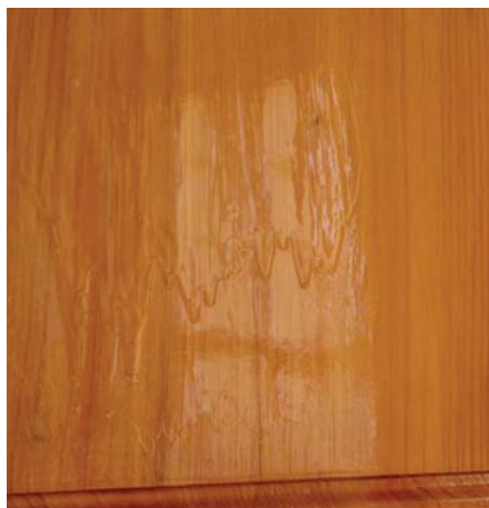
Reflected light. When working on a vertical surface, check often in reflected light to see problems, especially runs and sags like the ones here.
