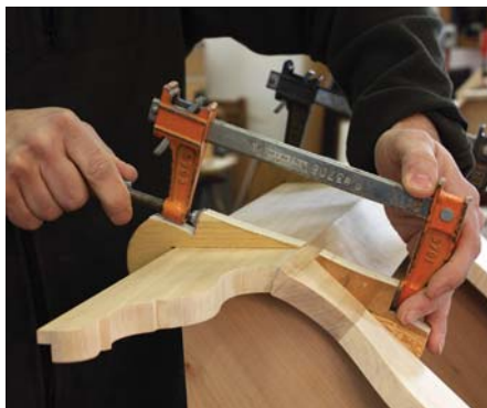
Angled clamping made easy. These cauls hook over the edges of the face frame and return, applying pressure right where it is needed.
