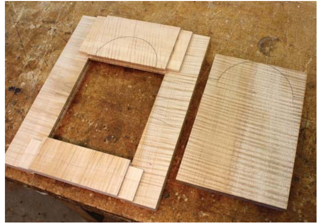
Arch madness. The radius of the arc of the top door stile is \frac{5}{16} " less than the radius of the panel arc. Note that the tenons have not yet been haunched.
