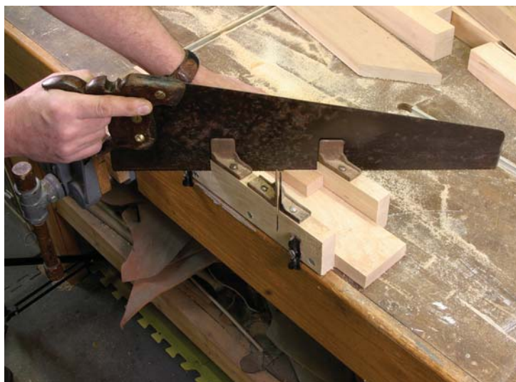
A simple box. A miter box can be as rudimentary as a U-shaped trough. This one has some commercial metal guides added to it to improve its accuracy.
