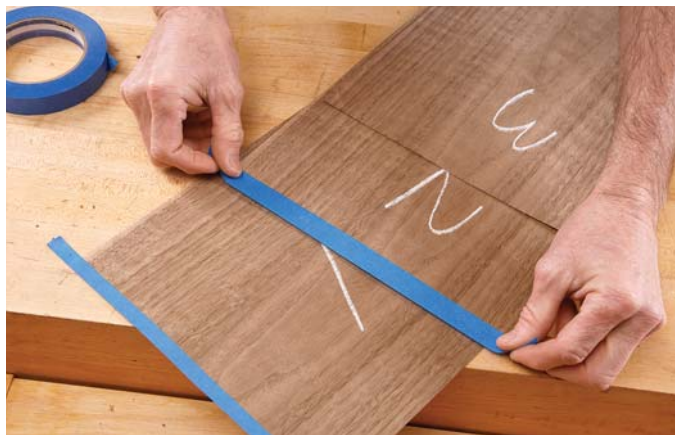
Blue has less goo. The blue “painter’s tape” is one of the ideal tapes for veneer work. Here I am using it to reinforce the fragile edges of this walnut veneer.
