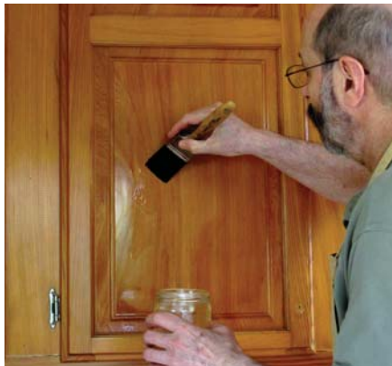
Brushing on. The first step is to get the wiping varnish onto the surface. You can brush it on in any direction or you can wipe on with a cloth. Here, I'm using a brush to apply the wiping varnish to a vertical surface that already has several coats built up.
