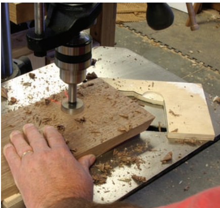
Form the foot. Use a 1 3 / 4 " Forstner bit to clean out the rounded portion of each design that forms the spur. Then at your band saw, cut away the remaining waste.
