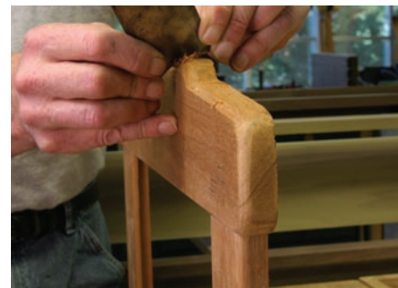
Final slices. A curved-edge card scraper efficiently removes the marks left by the rasp and removes any high spots along the edges.
