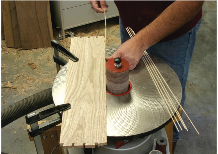
Sized right. Clamp a fence at your spindle sander to perfectly size the stringing thickness. Run a sample. If the fit is too tight, adjust the fence and try the setup again.
