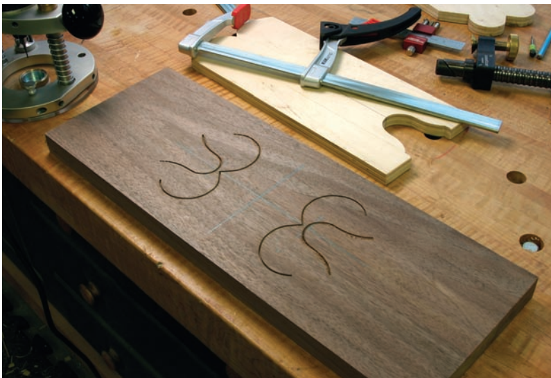
Step two. The completed tulip design faces away from the drawer center and is spaced just outside the bump design.
