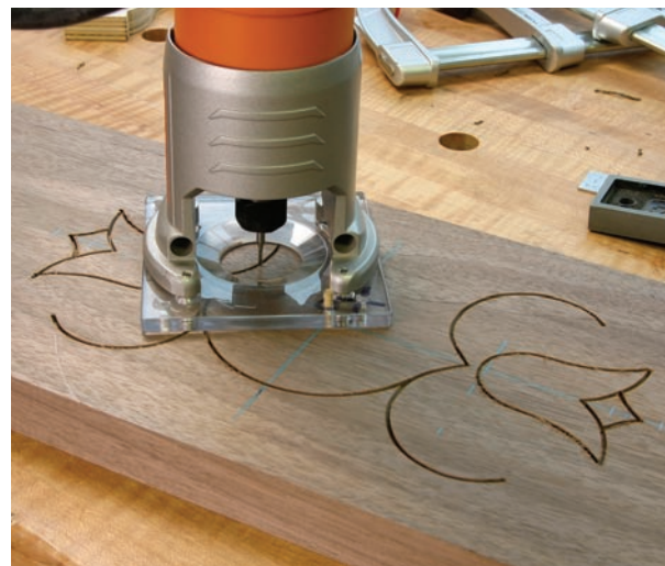
It's all in the base plate. The arcs around the center of the design are cut using the router base plate as a circle-cutting jig. Place a dowel into the drawer front's centered hole, slip the router plate over the pin then cut the groove from bump to bump.
