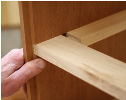
View from the back. Here is the rear of a drawer web frame with the rear tenon's shoulder cut short and left unglued to accommodate movement of the solid wood case side.
