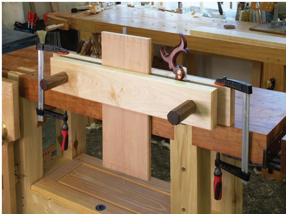
Back to the future. This vise might not have originally been intended for cutting dovetails, but boy is it great for it. It raises your work, then stows away when you don't need it.
