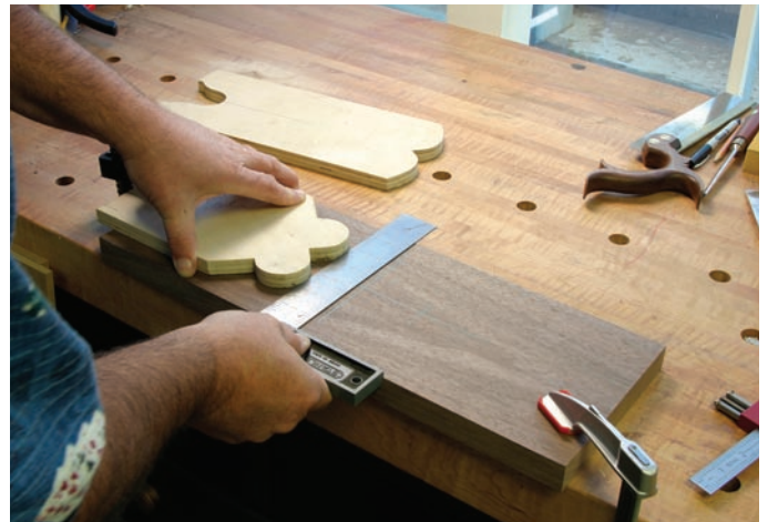
Keep it straight. The jigs used in this project are all held square to the drawer front. Proper placement is essential to the task.
