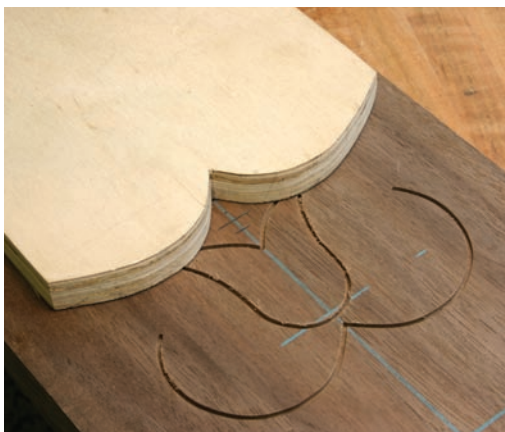
A simple reversal. Flip the wave pattern then set the distance between the pattern and the previous groove at 1" for the two top drawers and 1\frac{1}{4} " for the lower drawers.
