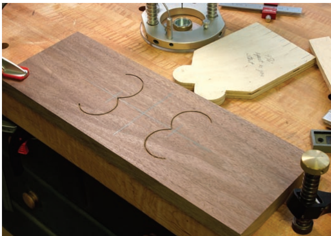
That's step one. These are the first set of lines in the design. The depth should be a strong \frac{1}{16} " for a secure fit that's easily trimmed after installation.
