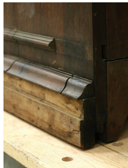
End grain return. In this solid wood dining room piece, the end-grain method for creating the return mouldings was used. This piece was subject to flood damage, so the delicate end-grain mouldings deteriorated.
