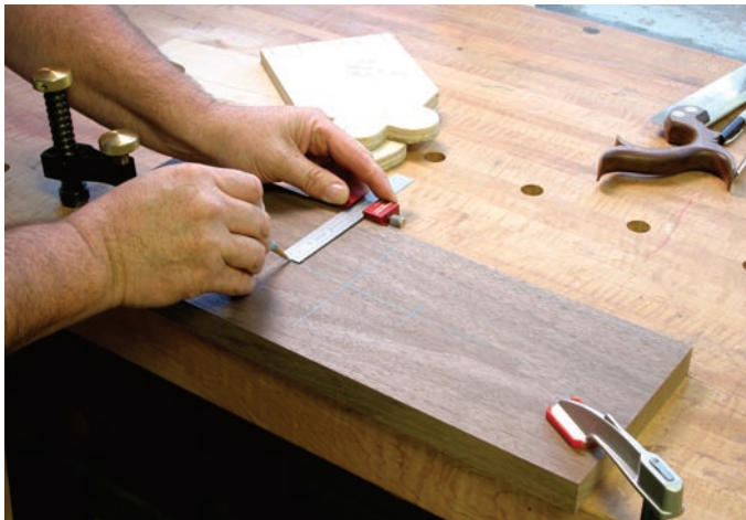
Proper layout. The design of the drawer fronts is dependent on getting your layout right. Space the lines off each drawer's center to keep the designs aligned.
