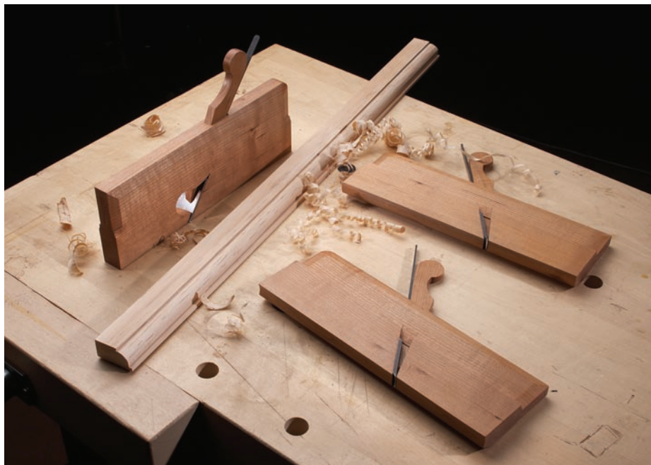
Making mouldings. Short runs of mouldings are easy to make with these planes. And here's a bonus: No more sanding mouldings.
