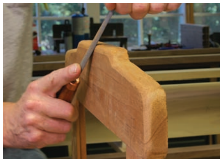
Variable curves. The radius of the rounded edges varies along the length of the edges. A series of rasps will allow you to go from rough to nearly ready in a short period of time.
