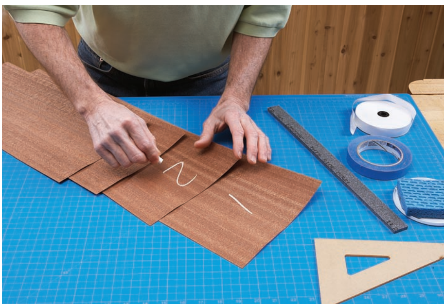
1 The numbers game. In order to cut a four-way match you will need four sequential pieces of veneer. Verify that they are in sequential order and with a piece of chalk, number each piece in succession.
