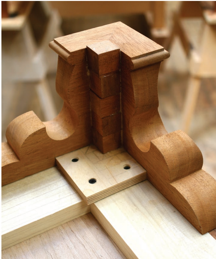
Stack them up. Hot hide glue makes quick work of gluing up a sandwich of corner blocking segments. This tactic prevents the bracket foot from splitting over time.
