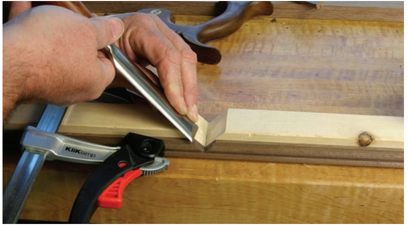
Back up that cut. The V-shaped notches that accept the drawer blade bead moulding need to be perfectly cut, as do the mouldings. Use a backer with a 45° opening cut made at the table saw to pare them.
