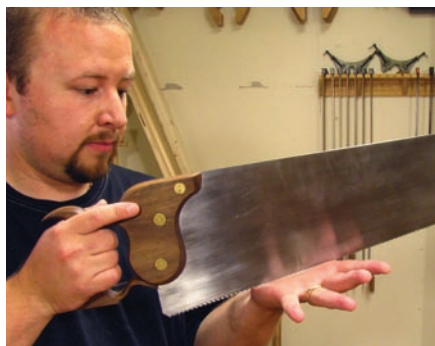
Test for sharpness. If the teeth don't grab the skin of your flattened palm when you try to gently move the saw across it, it's not really sharp.
