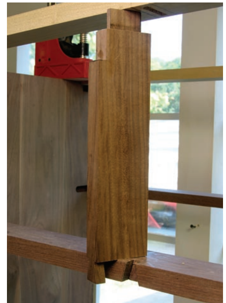
Want to make it easy? All the joinery work on the center divider is hidden—covered by the mouldings or the top. To make quick work of the divider, attach the piece to the blade and support rail with screws.
