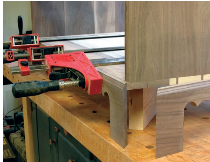
Work on your bench. Use scrap 8/4 to raise the chest off your bench and make fitting the base that much easier. One piece at each corner does the job.
