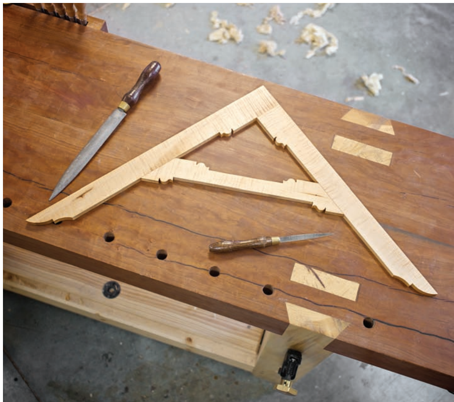
All this useful beauty. Tool pusher Patrick Leach found the original of this square in England. I built this reproduction, which is an excellent tool for layout chores.
