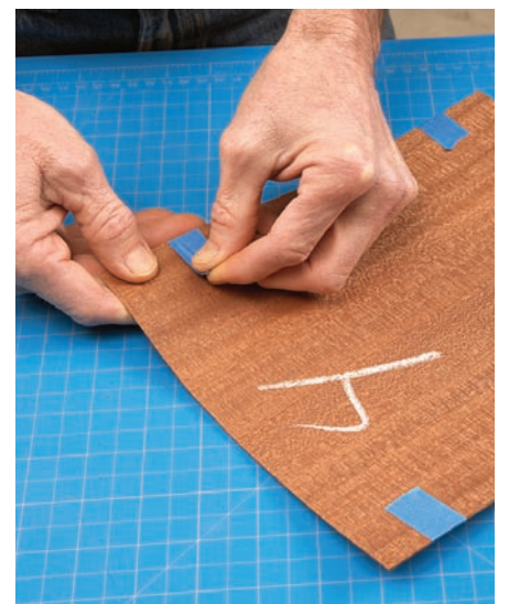
2 Stack it to be accurate. With masking tape, tape the entire bundle together to create a packet of veneer; this will keep each piece from shifting when cutting. I recommend that you stack cut all four pieces.
