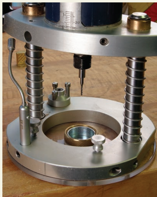
Stretching the point. Collet reducers, chucked into regular collets, can help to lengthen a router bit's reach.
