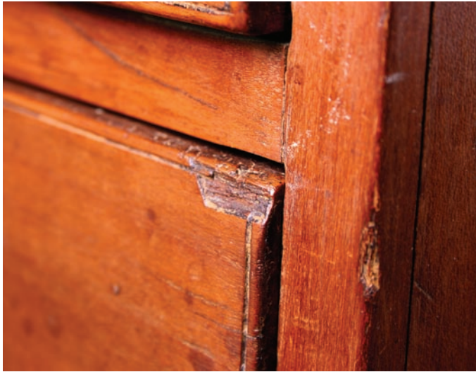
Busted. The corners of drawers are vulnerable, and it is common to see their edges chipped out like this.
