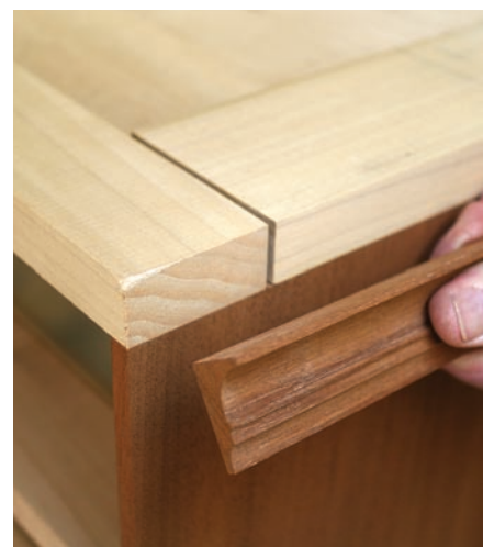
Elegant solution. A plinth built like a drawer web frame with an unglued, short-shouldered tenon at the rear accommodates the side movement.
