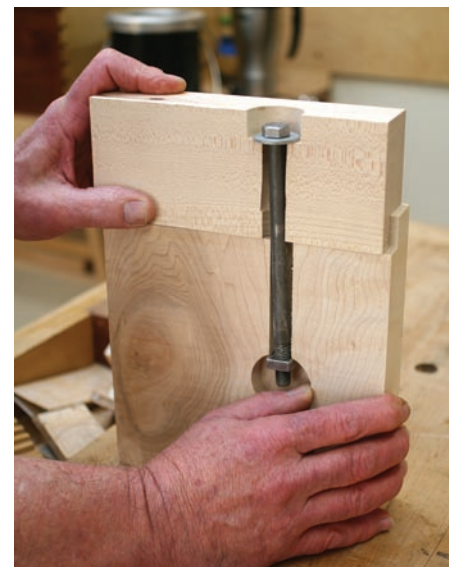
Flexible connection. This mock-up shows how a metal fastener can be installed with an oversized hole to avoid cross-grain splits.
