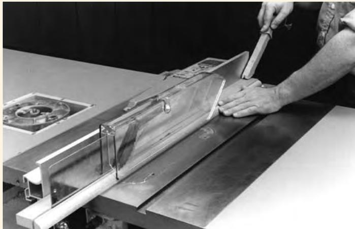
To make an applied moulding or picture-frame stock, cut the shape you want in the edge of a wide board, then rip it to the proper thickness, which I'm doing here on my table saw. Don't try to rout a shape in narrow stock – it may chip, splinter or kick back at you.
