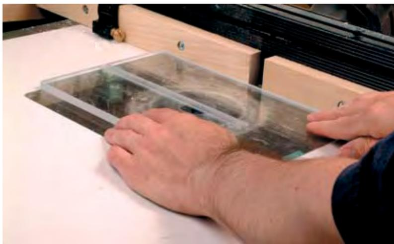
Running the grooves for the mounting hardware in both the offset base and the extension is a two-step router table operation. The  $\frac{1}{4}$ "-deep stopped groove is run first, using the router table fence to locate the slot in the center.
