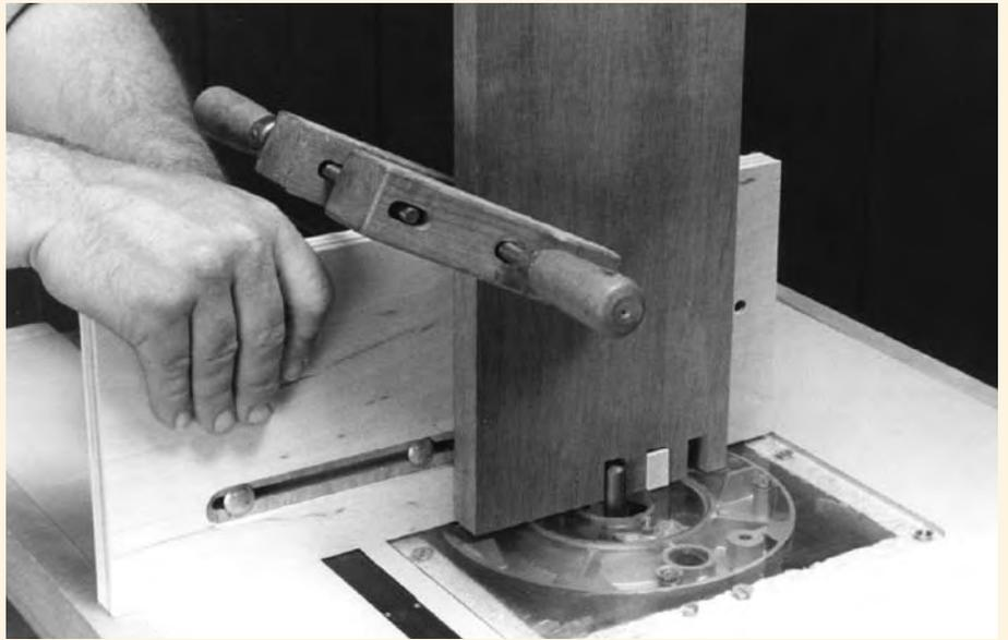
To use the jig, screw or bolt the mount to a miter gauge. Loosen the wing nuts that secure the face to the mount and slide the face sideways until the stop is the proper distance away from the bit. When the stop is positioned properly, tighten the wing nuts.
