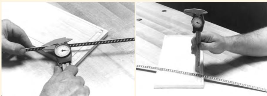
When inlay materials are thick, you can rout a recess to make the inlay "proud," then sand it flush. When inlay materials are thin, you risk sanding through them if you mount them proud. Instead, use calipers to measure the inlay thickness, then adjust the depth of cut to match.
