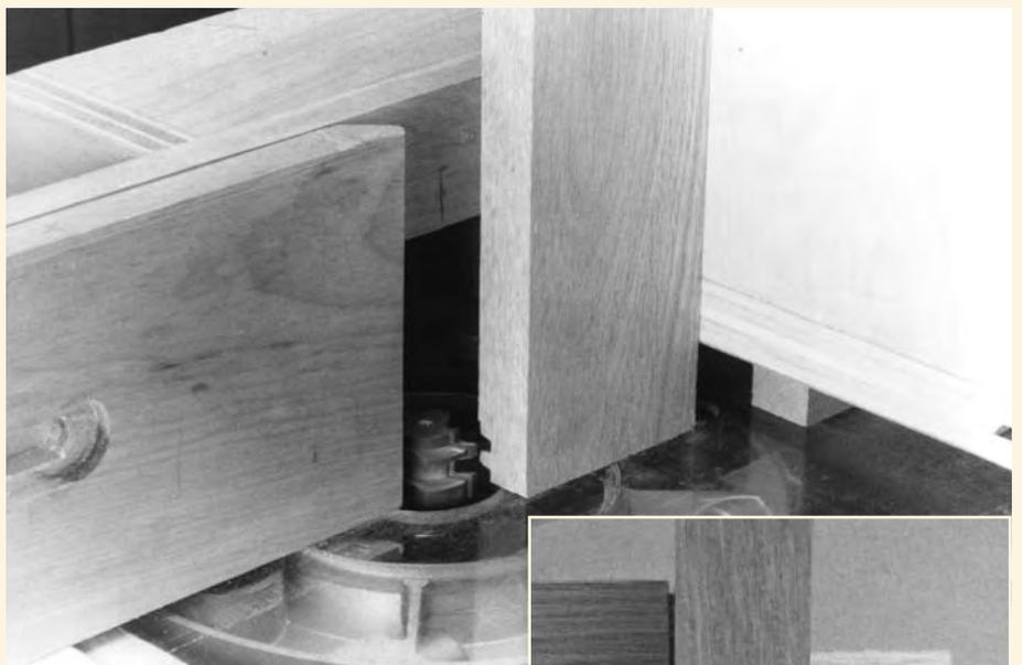
A drawer-lock joint requires only one bit and one setup. However, instead of reversing boards face for face as you cut them (as in the finger glue joint), you must cut the drawer front with the face of the workpiece against the router table, then cut the drawer side with the face against the fence. Adjust both the depth of cut and the position of the fence so the members fit together properly.
