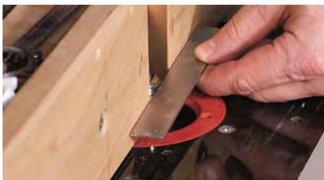
Setting up and using a cope-and-stick set of bits is relatively easy after the shimming is done. First, make sure the bearing on the bit is flush with the fence on the router table. Flushing the bearings makes sure that the profiles will match up. Use a straightedge that spans the two fences and tap the fence flush to the bearing. If possible, close the fence faces so there’s approximately 1/8" clearance on both sides of the cutter.
