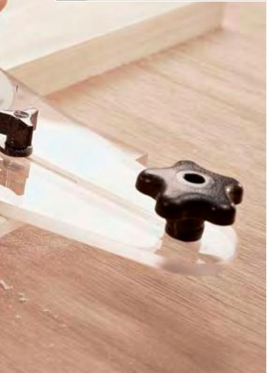
By swapping a few pieces of hardware, you can use this system as either a small (above, top) or large (above) circle-cutting jig, or simply as an edge guide.
