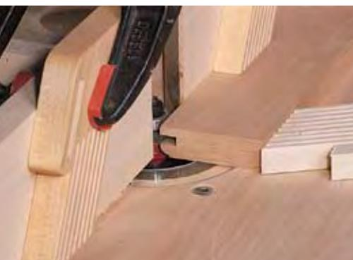
Using featherboards to keep your stock in place, press the stock into the fence and down onto the router table. Which profile you cut first isn’t critical. Use test cuts to get your bits in the ballpark. I cut the stick first. For door construction, you can cut your stock to finish length, but I prefer to leave the stiles a little long for trimming later.
