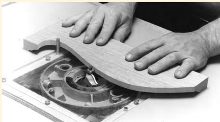
This safety consideration also applies to making curved mouldings, such as a classic "goose-neck" moulding. Cut the inside curve in the wide moulding stock, sand it so the curves are fair, then rout the shape in the edge.
