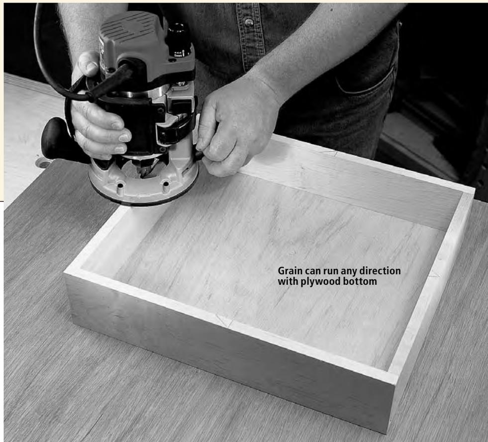
Grain can run any direction with plywood bottom
