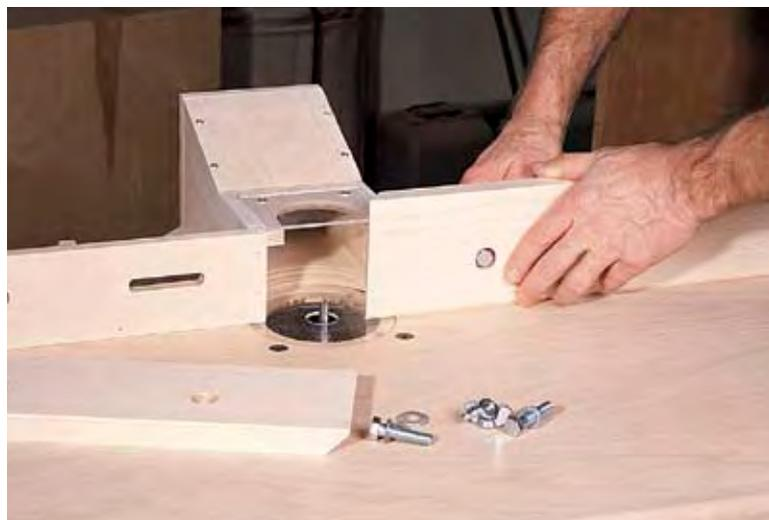
Attach the fence faces using  $\frac{3}{8}$ " roundhead machine screws, a star washer, flat washer and wing nut. I tried using hex-head bolts but switched to screws because a screwdriver can be used and makes a more secure attachment with less trouble.
