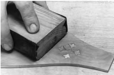
After gluing the inlays in, let the glue dry completely before you scrape away the excess. If the inlay is proud, hand-sand it flush with the surface. Don't use a power sander because inlays tend to be very thin and you might sand right through them.
