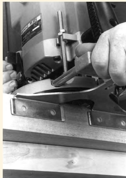
Most base-mounted guides will follow either straight or contoured edges, depending on the shape of the guide. Here, a straight guide – which looks like a small fence – rides along the edge of a board.
