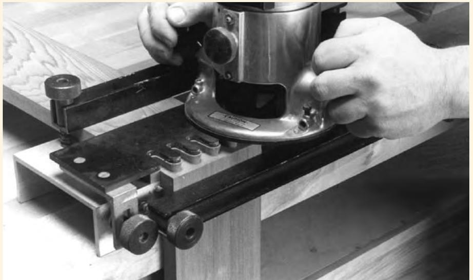
**When using a fixed through-dovetail template you can't change the size and position of the tails and pins. Rout the tails first, using the tail template, a guide collar and a dovetail bit. Then you can switch to the pin template and a straight bit. Fit the pins to the tails by moving the template forward or back on its holder. This will change the size, but not the location, of the pins.**
