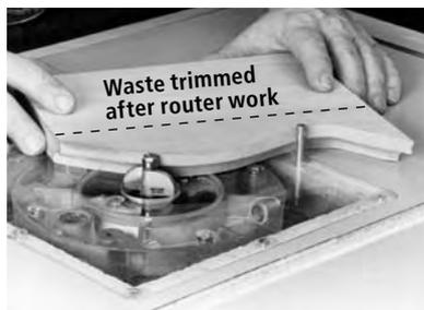
If a workpiece is very small, your hands may come too close to the router bit as you rout it. In this case, you have two choices – you can rout the work with a portable router using a commercially available foam rubber “routing pad” or double-stick tape to hold the work, or you can rout a portion of a larger workpiece and cut a small piece from it, as seen above.
