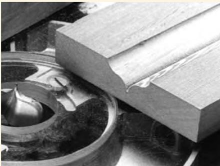
Point-cut bits with a complex shape, such as this pilotless ogee bit, cut a broad groove with an interesting shape. The sides of the grooves are mirror images of each other.
