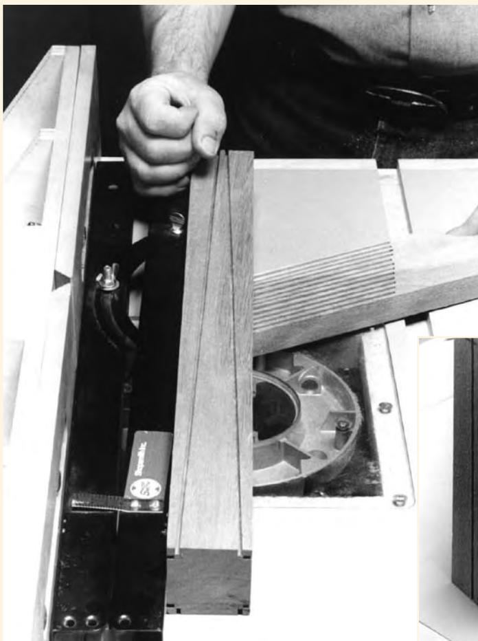
When cutting straight grooves, you can use a variety of jigs to get a decorative effect. Here, a tapering jig produces a pattern of angled grooves in a table leg. The grooves create the impression of a tapered leg, even though it's straight.
