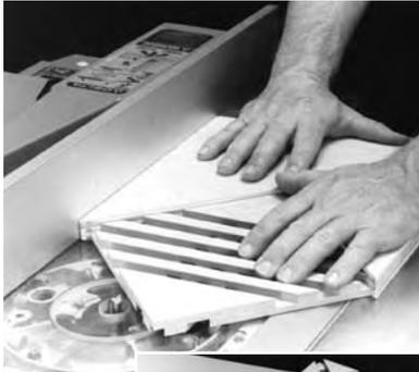
Cut a set of grooves in a board that are parallel to each other. Make each groove a little more than half as deep as the board is thick. Then turn the board upside down and cut another set of grooves at an angle to the first set. Where the grooves intersect, they will create openings. The size, shape and spacing of these openings depends on the size, shape and spacing of the grooves.
