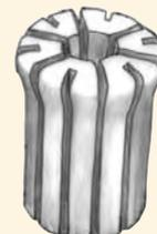
Collets with just two to three segments (left) don't squeeze router-bit shanks evenly. In fact, they make contact at just a few points. Collets with multiple segments (right) are more flexible and make contact all the way around the shank, which helps keep the bit from slipping.
