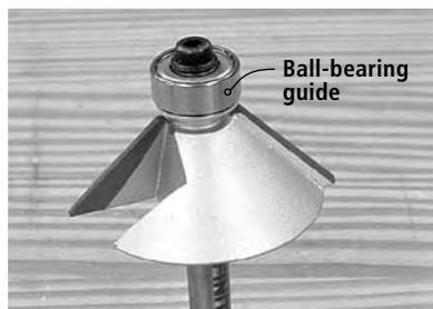
You may still find a few piloted router bits out there, but ball-bearing router bits are far superior, and have all but replaced the older design. Upkeep is easier on the ball-bearing design because all you have to do is add a little lubrication from time to time.
