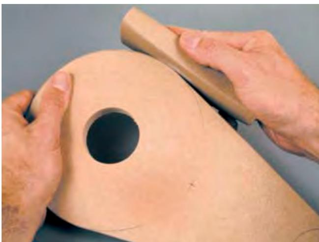
With everything cut, bored and sized appropriately, the last step is to clean up the edge so that it's smooth. A block and sandpaper can do most of the work, but an edge sander (if available) will be much quicker.
