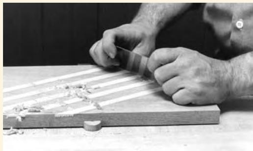
When the glue is dry, remove the board and the covering, then scrape away any glue that remains on the surface. But be careful – you don't want to scrape through the banding.
