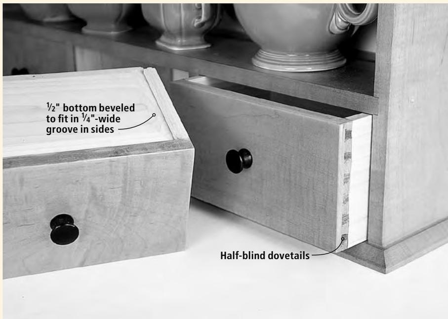
1/2" bottom beveled to fit in 1/4"-wide groove in sides
