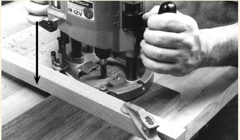
To rout a mortise with a plunge router, clamp a straightedge or guide to the workpiece and adjust the depth stop. (You also may use a base-mounted guide attached to the router.) Position the router over the work, holding the base against the straightedge (or the guide against the work). Release the height clamp and push the bit into the wood.
