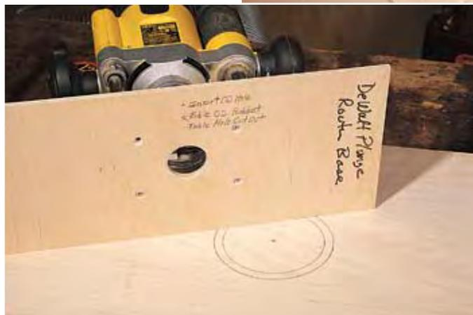
A larger base for the router was the ticket for bridging the open areas left by routing out the plywood for the router's base. It was also used as a small circle-cutting jig for the tabletop and plastic inserts. Use the same cutter and it's easy to keep track of dimensions for cutting inside or outside circles.
