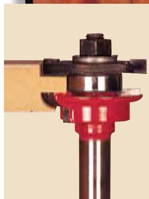
Cutting the cope on the rail's end.
