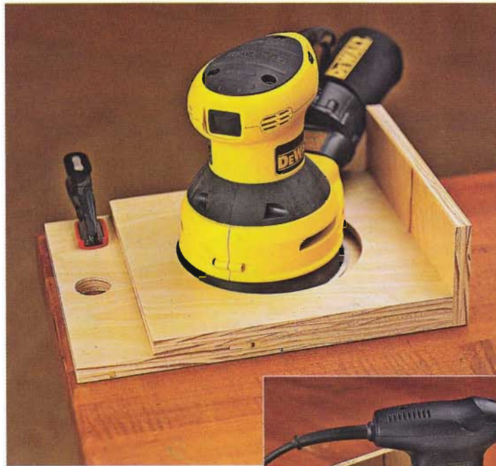
The optional support at right , works well for the vacuum hose to rest on, preventing the sander from tipping over.
