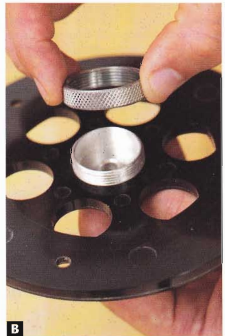
Two-piece guide bushings easily attach to your router's base and offer exacting accuracy when lining up holes.
