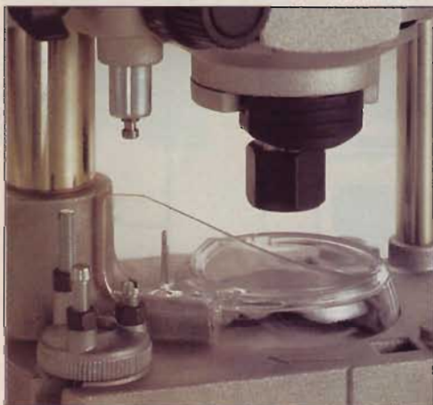
Like a cyclone chamber, this plastic shroud causes the vacuum air to swirl around the bit and pull debris toward the hollow post.
