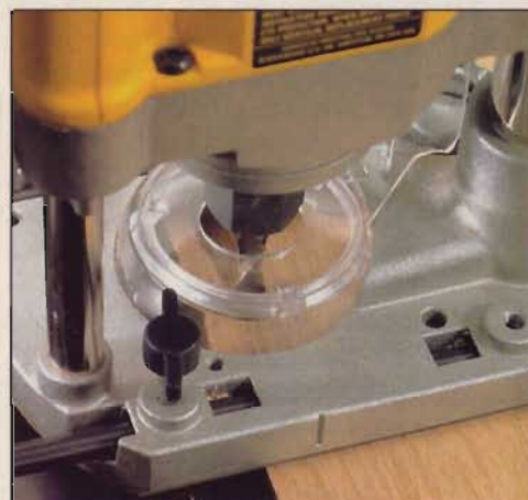
With the shroud installed and the vacuum hooked up, the bit area is so clean that you can easily see your routing layout lines.
