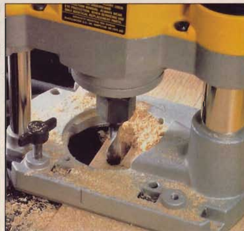
Without the plastic shroud, the DW621 performs like any other router, meaning dust piles up on the workpiece, bench, and floor.
