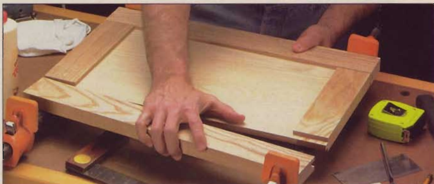
Stub tenon and groove joints are perfect for light duty frames, page 34.
