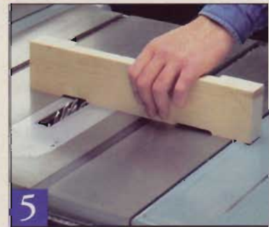
5 Rip the two feet from the blank, then stand the pieces up and cut away the waste that remains in the insteps.
