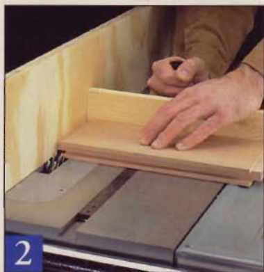
2 Clamp a scrap wood face to the saw fence to avoid having the blade score the fence during the tongue cutting operation.
