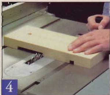
4 To form the wide dado, first make two passes to define the ends of the dado, then remove the waste between the first cuts.
