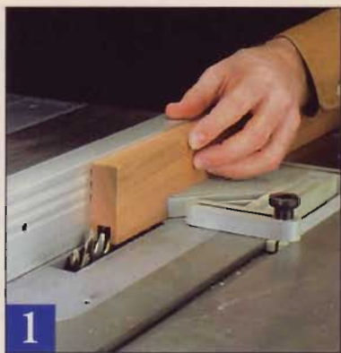
1 For consistent grooves, keep steady pressure on the rails and stiles as they pass over the 1/2" dado blade.
