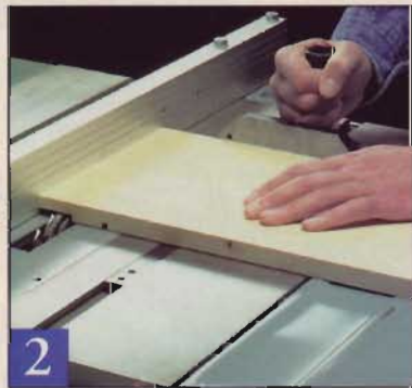
2 Switch to a 1/2" dado blade and make several passes to cut the wide dado at the top end of each side. Then cut the shelf dadoes.
