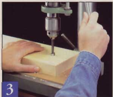
3 Lay out the feet on a 6 1/8"-wide blank, then bore 5/8" diameter holes through the stock to form the curve at the ends of the instep.
