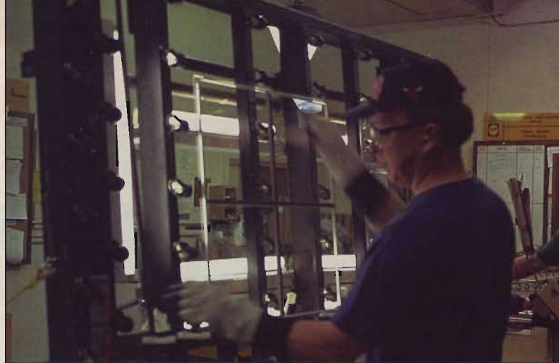
An aluminum frame mounted between the panes of glass creates the gap for the argon gas. Foam inserts prevent light from glancing between the panes on windows with mullions.
