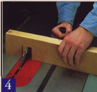
4 Positioning the rip fence as an end stop lets you make the outside cuts for the notches; a few cleanup passes finish the job.
