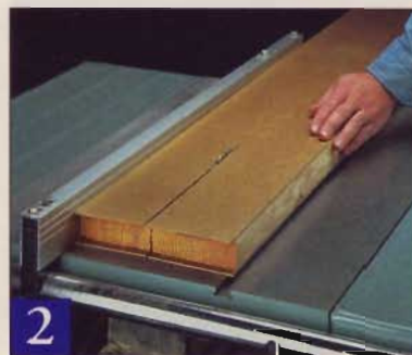
2 Rip the rails from the oversized glued-up blank. Cupped or twisted stock may require multiple passes to produce square edges.
