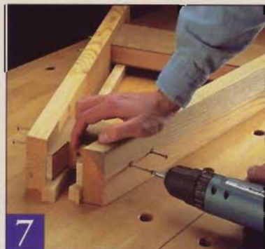
7 A pair of \frac{7}{8} "-thick spacers will help align and center the gussets while you're assembling the A-frames. Use exterior glue here.
