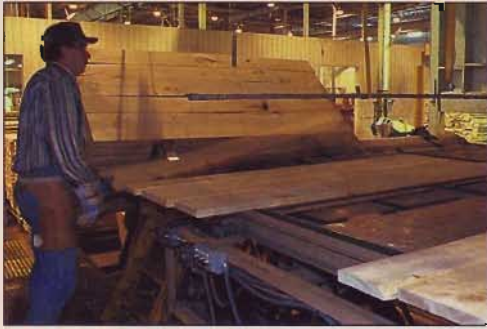
Conveyors move lumber over a moisture sensor. Boards that meet the standards line up for evaluation at the shadow line station.
