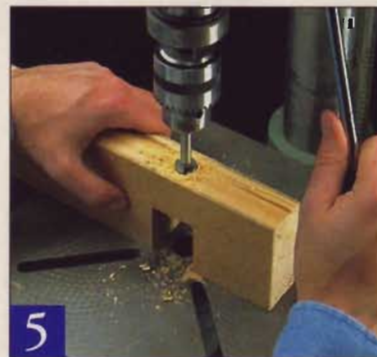
5 Counterbore the stretchers so the bolt heads and the T-Nuts will nest below the surface, then drill for the bolt shank.
