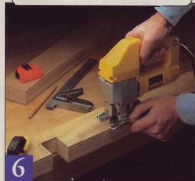
6 The cloud-lift contour on the rails can be cut with a jig saw, or, since they're non-functional, left out of the design altogether.
