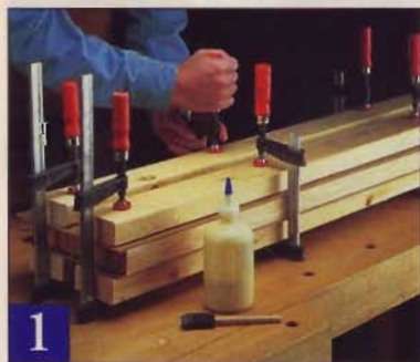
1 When you laminate the hardboard skins onto the rail and gusset stock, use clamping cauls to distribute the pressure evenly.
