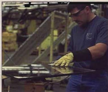
A coat of polysulfide applied to the edges of the aluminum frame seals the argon gas in the insulating gap between the panes.
