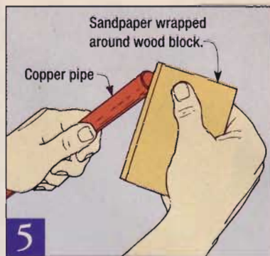
5 Wrap 120-grit sandpaper around a wood block and chamfer the ends of each pipe. Chamfers ease the pipe installation.
