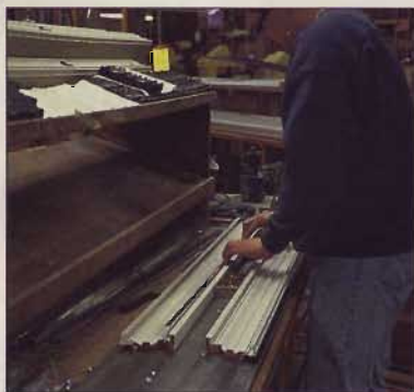
The jambs mate to wood back-up pieces (mostly finger-jointed material). Adding glass weather seals and sash hardware is next.
