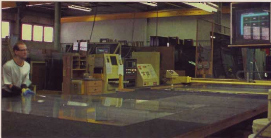
Short stock passes through a finger-jointing machine. After the joints are milled, the stock is glued into longer pieces.
