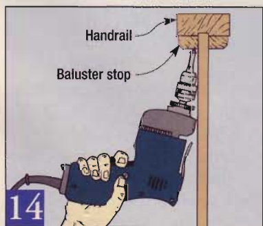
14 Screwing the baluster stops in place makes it easy to remove them without damage. Air-nailing (no glue) is a second option.
