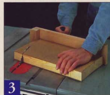
3 With a simple positioning jig fastened to your miter gauge, you can safely trim the ends of each gusset at a 15 degree angle.
