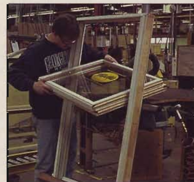
Screws join the jambs to the sill and cap, then the sash clip into the frame. The cables fasten to the sash, providing lift.
