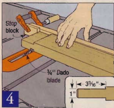
4 When you cut tenons, clamp a stop block to your wood miter gauge extension. This guarantees that all tenons are identical.
