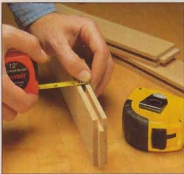
Matching tool size to the job is a prime ergonomic principle. I've switched to a small tape measure for benchtop chores.
