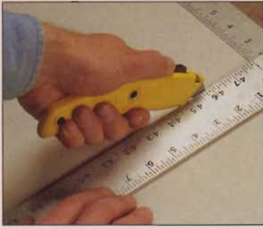
It may look like a banana, but Stanley's utility knife is a serious tool that keeps your wrist in the desired neutral position.
