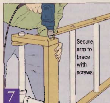
Slip the hinge bracket arms onto the PVC hinge assembly, then drill countersunk pilot holes and screw the arms to the base.
