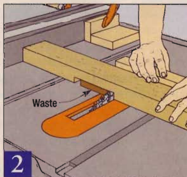
2 To cut the top end of the dado, butt the leg half against your rip fence. Remove the waste (shaded area) to finish the joint.
