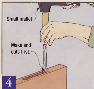
To square the mortises up, start with end cuts (across the grain). You can use a mallet, but cedar won't need brutal hits.
