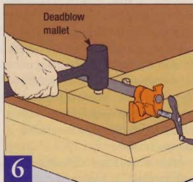
6 Use a clamp to close the joint, then check the assembly for square. Drive the pegs with a deadblow or wooden mallet.
