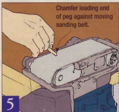
5 A belt sander makes quick work of the end chamfer on each peg. Don't skimp here — that "nose" is your navigator.
