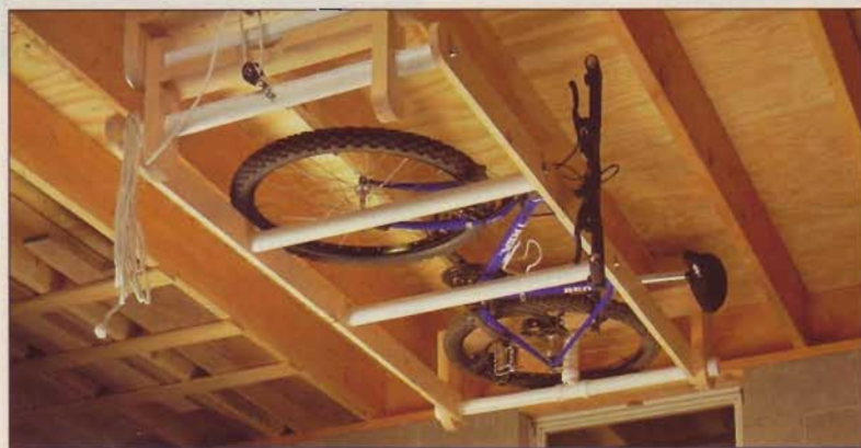
Thread the rope through the pivot bracket hole to the end rung pulley, then back up to the pivot bracket pulley.
