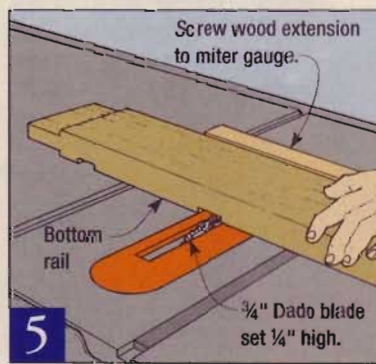
5 Use this table saw setup to cut dados for seating the stretchers. The bottom rails have two dados; the top rails have one.
