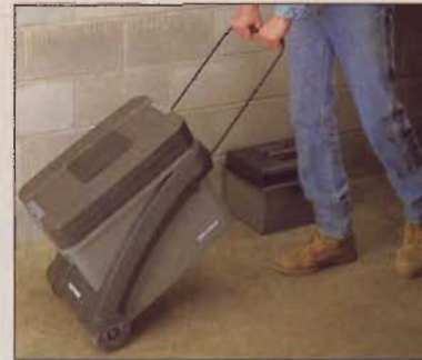
The Sears Craftsman SST tool box has a handle and wheels that can save your back. Push, don't pull, to eliminate twisting.
