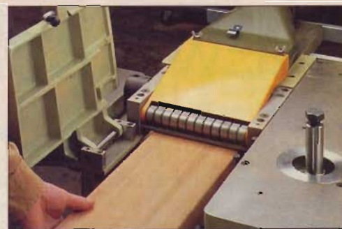
The jointer tables fold up to reveal the planer. The hinged dust hood pivots in place for either operation — a nice touch.
