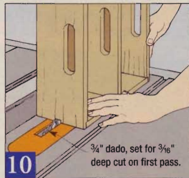
10 Use a 3/4" dado blade to cut the grooves in the drawer sides to accommodate the hardwood drawer runners.
