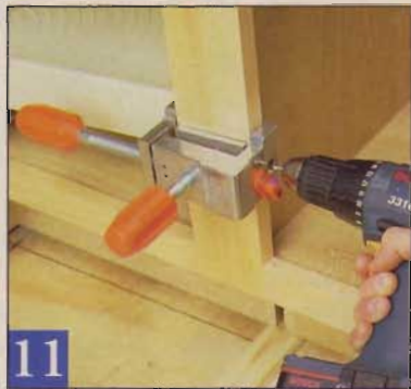
The Cabinet Claw not only clamps the face frames flush, it has a swing-away guide for drilling and for driving screws.
