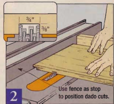
2 Cut matching dados in both side panels before moving the fence. Dado for the upper runners first, then the lower runners.
