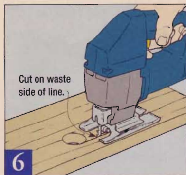
6 Use a jigsaw to remove the waste between the 1" holes to form the handle cutouts. File and sand the edges smooth.
