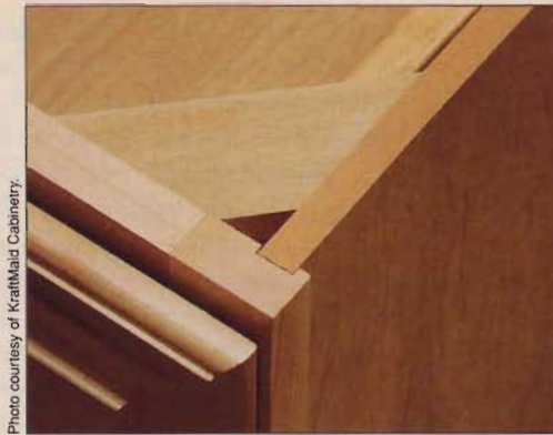
Higher-quality cabinets feature wooden corner bracing glued into grooves cut into the front and side panels. Side panels are also \frac{5}{8} " or \frac{3}{4} " plywood or MDF.
