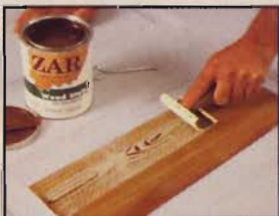
A graining tool and ZAR Stain create a rich wood-like finish on steel doors.
