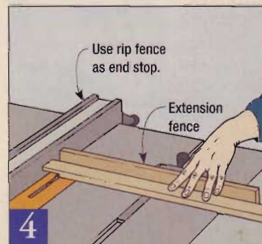
Using a miter gauge with a wood extension, cut half-lap joints in the frame stock with a dado blade. The rip fence acts as a stop.
