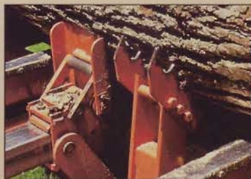
A hydraulic log turner rotates logs as long as 21-ft. and up to 3-ft. across. Hydraulic clamps secure the log.
