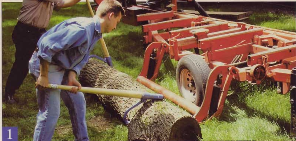
1 With help from Burl, Assistant Editor Dave Stone rolls a log onto the mill's hydraulic loading arms. Logger's cant hooks, or peaveys, give much-needed leverage.
