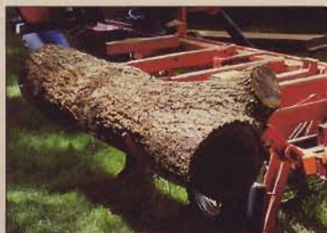
Once you manually roll a log onto the loading arms, you can use the LT40's hydraulics to lift it onto the mill's skids.
