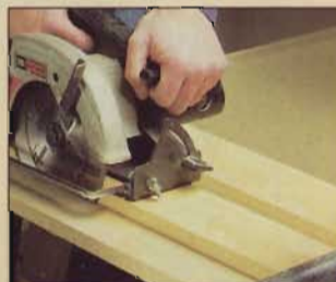
A guide clamped to the underside puts the saw flush with the edging lip and controls the cut.
