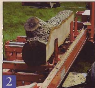
2 Burl cut away the sapwood on one log face then rolled it to square the adjoining face.
