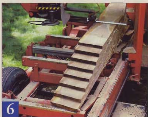
6 You can remove each board as it's cut, or leave them in place and slice the whole log before pulling the boards.
