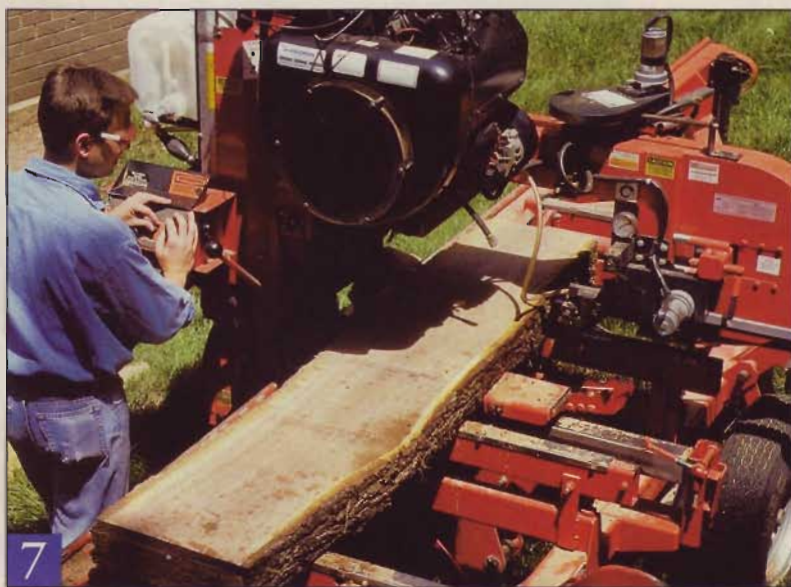
You don't have to shape a log into a cant. On a trunk section, Dave flattened one edge of the log, then flipped it over and flat-sawed the rest to create wide, rough-edged boards.
