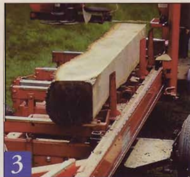
3 With the second face cut, the square core (called a cant) begins to take shape.
