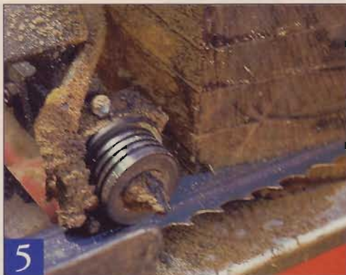
5 The mill's thin blade wastes little wood. Water keeps the blade running cool and prevents pitch buildup.
