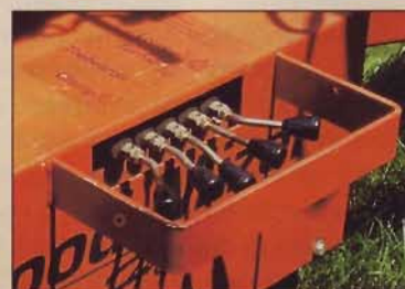
By operating these levers you can load, turn, clamp, and level a log using hydraulic power instead of your back.
