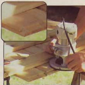
A wide, shallow rabbet allows the bottom edges of the doors to close against the shed floor.
