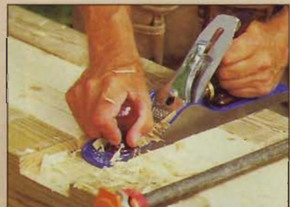
Clean up nibs and other high spots with a hand plane. You have to go across the grain, but minor tearout won't affect the joints.
