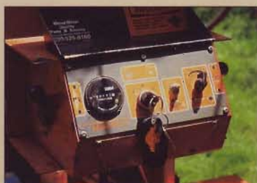
The controls move with the saw carriage over the stationary log as you walk along controlling cutting depth and speed.
