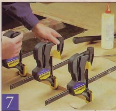
7 Once it's trimmed to fit, place the substrate sections upside down on a level surface, then glue and clamp them together.
