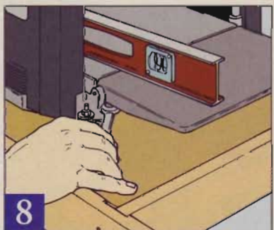
8 Use a level to check alignment of the planer's infeed and outfeed tables. Adjust them according to manufacturer's instructions.
