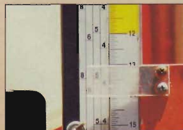
A large rule above the controls shows depth-of-cut in both inches and quarters — the thickness standard for hardwoods.
