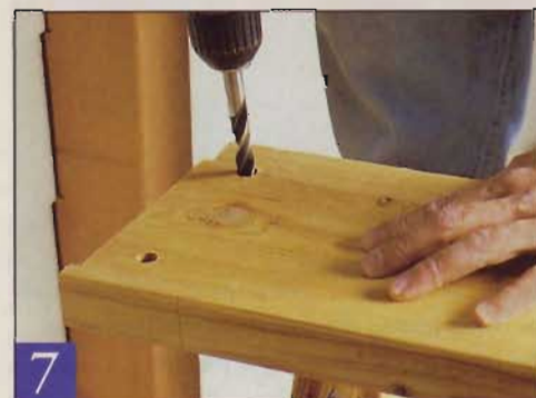
7 Carefully mark the location of the mounting holes on both ends of the beams. Then use a brad-point bit to drill 1/2"-dia. holes through the beams.
