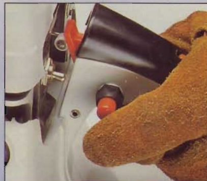
The trigger lock (orange switch near thumb) partially opens the throttle to aid starting. You release it immediately once the engine fires.
