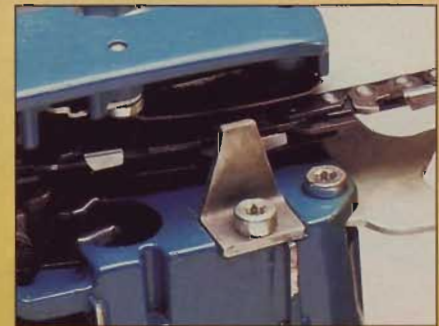
The chain catcher is there to snag a broken or derailed chain, preventing it from lashing back at the operator. On this Makita, it's a flat bar.
