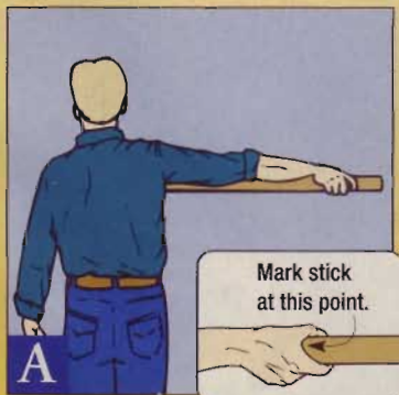
Extend your arm and nest an end of the gauge stick in your armpit. Mark on the stick where your thumb and palm meet.
