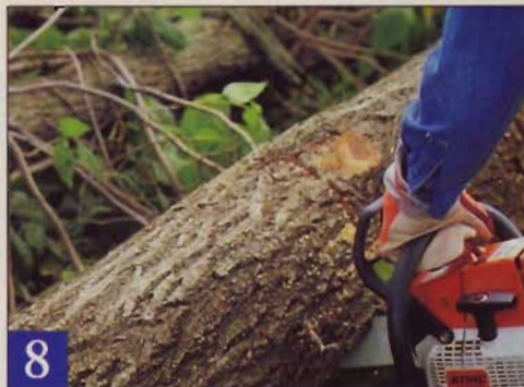
Reverse the procedure when a log is supported at both ends. This time, cut \frac{1}{3} into the top, then finish from below. This will keep the bar from binding in the kerf.
