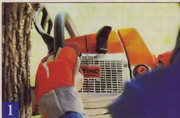
1 Align the saw’s felling sight (black line on housing) with the target stake. Use tape or a pen to add a sight if your saw lacks one.
