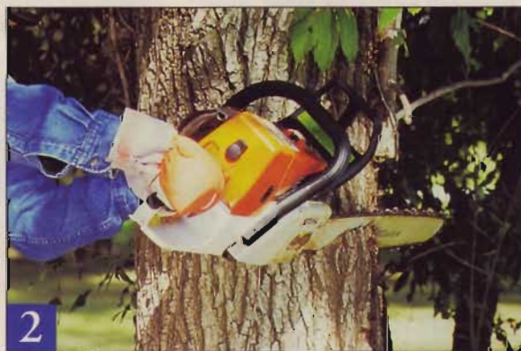
2 Prepare to cut the notch by standing next to the tree and facing the target stake. Hold the saw at a 45° downward angle.
