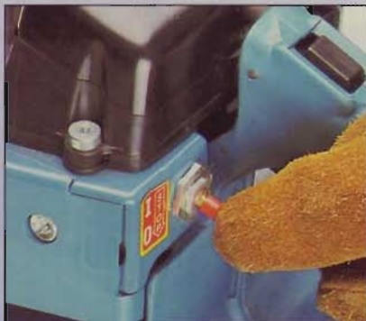
Location of the on/off switch is an important (and personal) consideration. Try out all the controls while wearing your working gloves.
