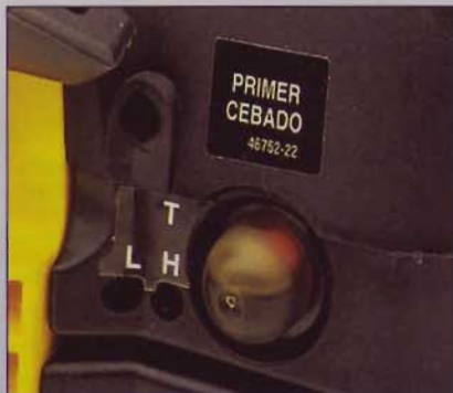
Some saws feature a primer bulb, a flexible clear plastic cap that when pressed helps pull fuel into the cylinder for easier cold starting.
