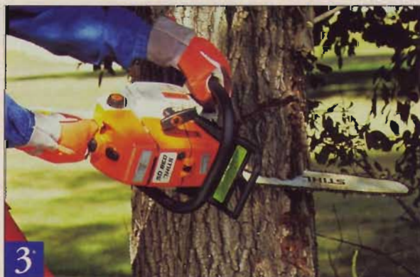
3 The lower cut of the notch slopes upward at about 45°. Make sure that the ends of the upper and lower cuts meet exactly.
