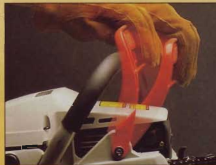
The chain brake lever gets bumped forward by your wrist if a kickback lurches the bar toward you. You also engage the brake for starting.
