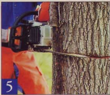
A horizontal line scored into the bark joins the two tips of the notch. This line helps you guide the saw during the felling cut.
