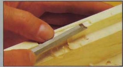
Step 5: Carefully form a shallow mortise in the lid banding for the catch plate.
