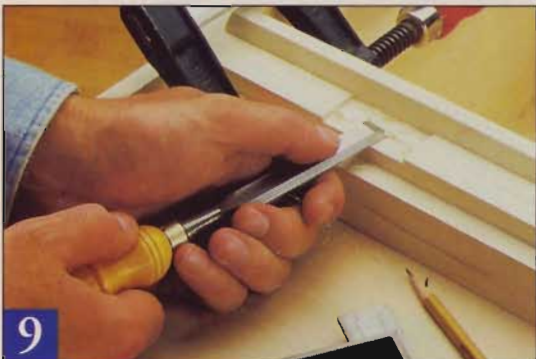
Clamp the lid to the case so the banding is flush with the upper molding. Then lay out and chisel the hinge mortises.
