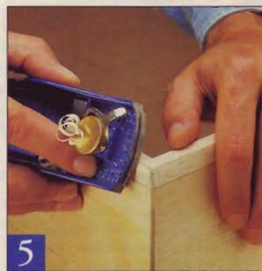
5 Form the chamfers with a block plane by removing the stock between the layout lines — go easy at the rabbeted corners.
