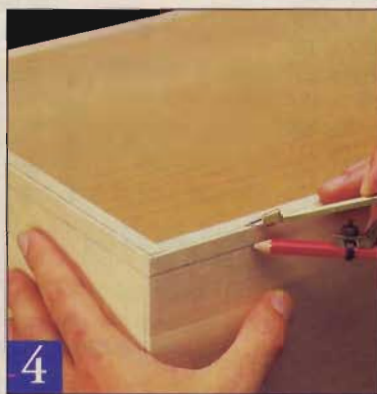
4 Using a compass, lay out the margins of the chamfers — \frac{1}{2} "-high \times \frac{1}{4} "-deep — along the top edges of the case.
