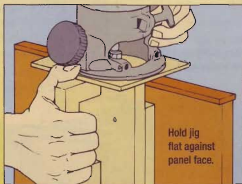
Use a flush-trimming bit and this jig to rout edging flush. Mount router so the bit aligns with the jig's base.
