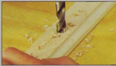
Step 1: Drill a 1/2"-dia. hole for the key barrel. Drill from the front to avoid visible tearout.
