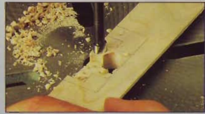
Step 2: Mark out the mortise location, then use a Forstner bit to remove most of the waste.
