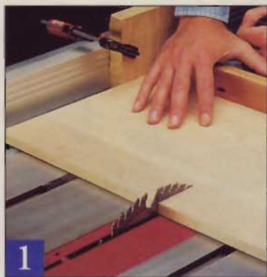
1 Clamping a stop block to the fence allows you to cut matching panels to the same length. Be sure to trim an end square first.
