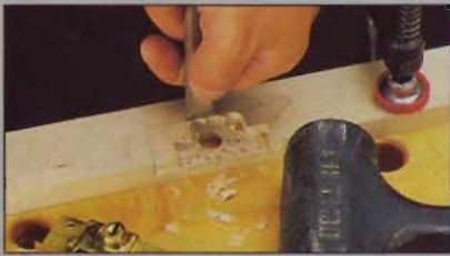
Step 3: Use a chisel to square the mortise to the layout lines and clean up the bottom.
