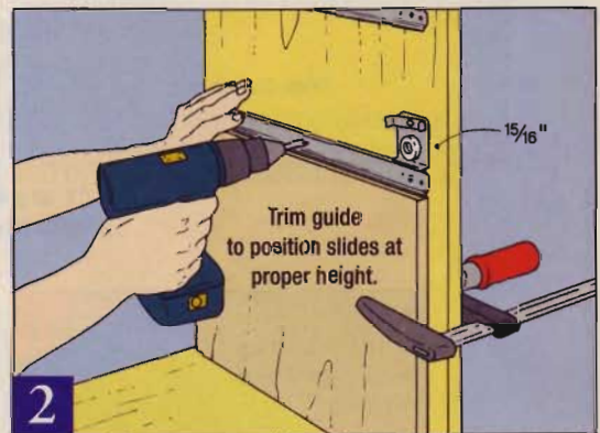
2 Rest a drawer slide atop the guide and drive the screws. Trim the guide to install each pair of slides.
