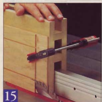
15 Beveling the panel's edges 8° requires a tall support. Raise the blade to meet the grooves you cut in the face of the panel.
