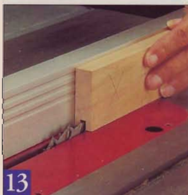
13 To ensure consistency, have the front of all your rails and stiles facing away from the fence while cutting the grooves.
