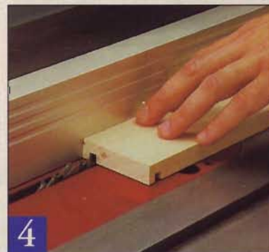
4 Cut grooves for the tray bottoms, then test fit the melamine panel. If the groove is too narrow, adjust the fence for a second pass.
