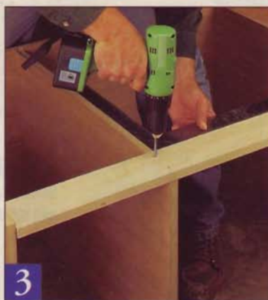
3 Make sure you square the dividers to the carcass rails before drilling countersunk pilot holes.
