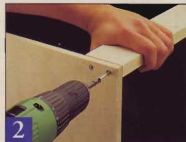
2 Screw the box together (no glue) and slip it into the cabinet to double check its width, height, and depth — a little play is ideal.
