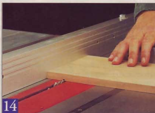
14 To raise panels, first define the raised area. Set the blade depth to 1/8", and clamp the fence 1 1/4" away. Cut four grooves into the panel's face (once with each edge against the fence).
