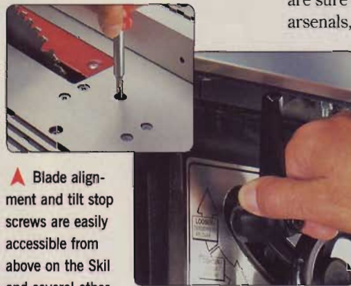
▲ The long lever and left-hand threads made the the Skil's tilt lock difficult to operate.
