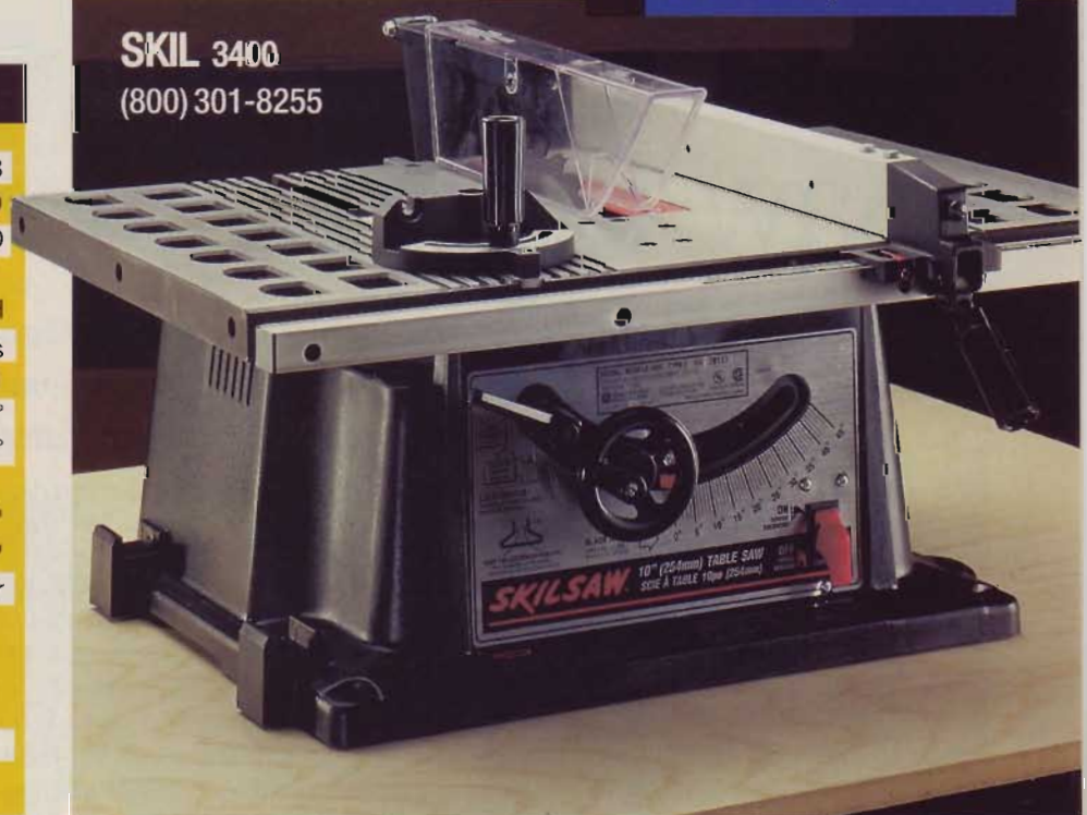
▲ The long lever and left-hand threads made the the Skil's tilt lock difficult to operate.
