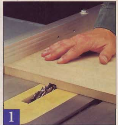
For crisp dados, keep the panel's edge firmly pressed against the fence as you steadily push the stock through the blade.
