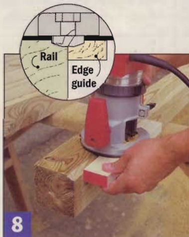
8 I used a faux raised-panel cutter to rout a shouldered bevel on the rails. Orient the rails face up for this.
