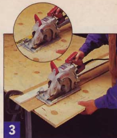
3 For finish cuts, an edge guide — either homemade or commercial — steers the saw in a straight line.
