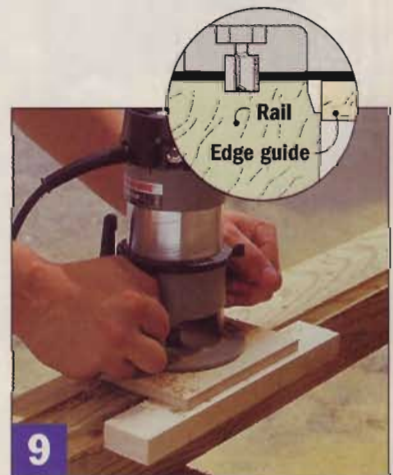
9 This edge-guided router setup, with a 3/4" straight bit, produced the spline grooves. Keep guide on the front face.
