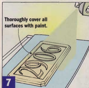
7 After removing the number templates and sanding the sign, spray on several coats of paint. Dark colors work best.
