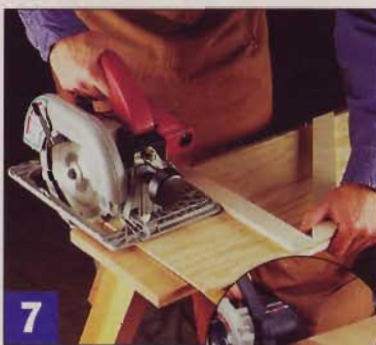
7 Square cuts on wide stock require a guide. This simple jig or a Speed Square helps cut angles too.
