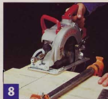
8 Clamping boards together lets you gang-cut them all in one pass. Though it takes time to set up, this one-cut method ensures uniform lengths.
