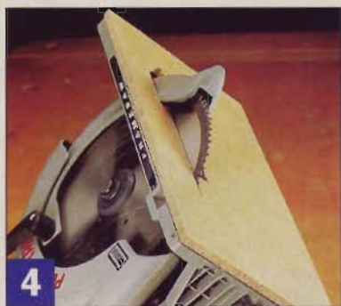
4 Double-face tape holds a zero-clearance plate to the saw. The plate and a fine-tooth blade reduce splintering.
