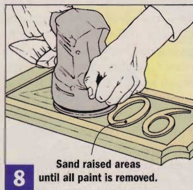
8 An electric sander and 120-grit paper quickly removes paint from the sign's raised surfaces, exposing the wood.
