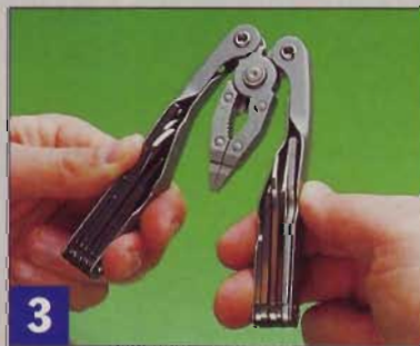
3 Schrade folded the handles around the pliers head. Though not as compact as some, its handles are comfortable.
