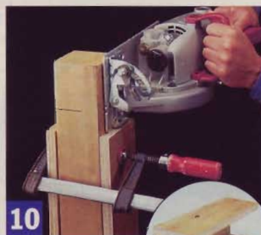
10 A U-shaped jig keeps the blade aligned when you make cuts from opposing sides of the post.
