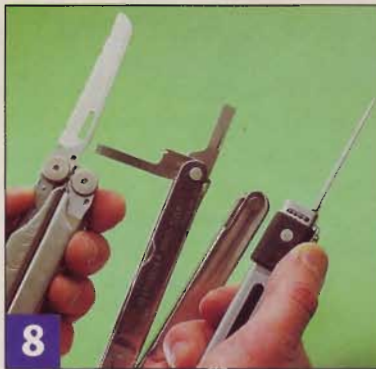
8 Spring locks (left) or sliding buttons (right) operate easily. To release the Leatherman SuperTool's lock (center) you must rotate another blade to 90°.
