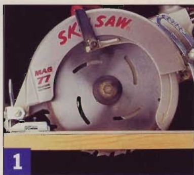
1 Adjust blade depth so the gullets extend past the bottom of the workpiece to clear sawdust from the kerf.
