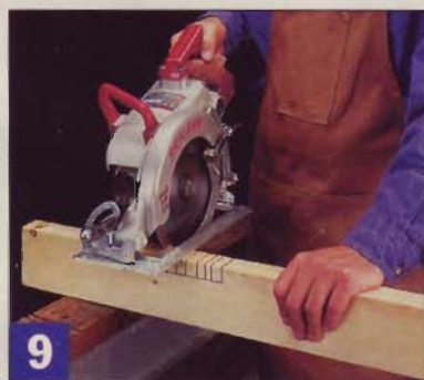
9 To notch your stock, make multiple cuts within the notch layout — with the blade set to the depth of the notch — then use a chisel to remove the waste.
