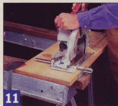
11 An edge guide lets you accurately rip stock. Clamps allow you to use both hands to steer the saw. Sacrificial top caps on your sawhorses are a must.
