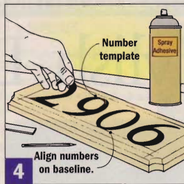
4 Draw a baseline to simplify aligning the number patterns, then stick them in place with spray adhesive.
