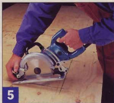
5 To make plunge cuts, retract the guard, line up the blade, then pivot the saw down into the cut.
