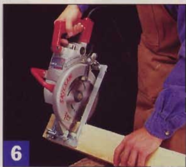
6 Framers often take advantage of gravity, letting it pull their worm-drive saws through the cut. Tilt the 2x stock on edge and simply guide the saw.
