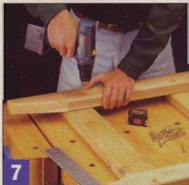
7 Position one foot and the inner top rail on a pair of legs. Hold the assembly firm and drill 5/32"-dia. countersunk pilot holes for the mounting screws.
