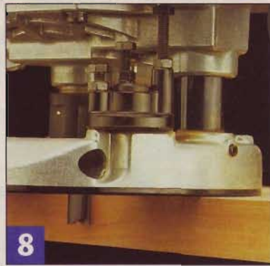
8 Most plunge routers have a turret with three adjustable depth stops. You can preset the turret stops to make a shallow cut first.
