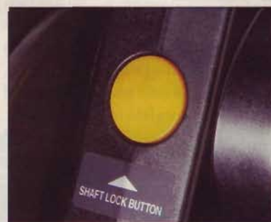
Adjustable kerf indicator on Panasonic saws eases cut line viewing. Spindle lock button is large and well-positioned.
