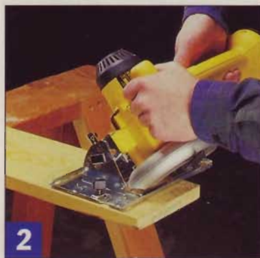
All the saws tested can be tilted to make bevel cuts of at least 45°. We did this with each one, noting capacity, adjustability, and ease-of-use.
