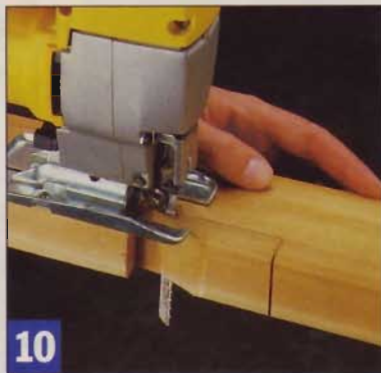
10 Make the two notch end cuts in the upper stretcher first. Make an angled cut from the center to one corner, then complete the bottom of the notch.
