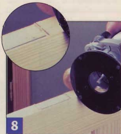
8 An ordinary router with a straight bit will clear most of the waste from each hinge mortise. Cutting depth should equal the thickness of the hinge leaf.
