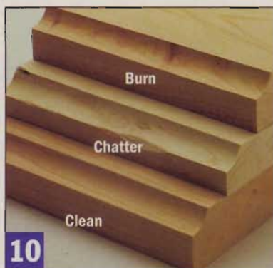
Using the proper feed rate is almost as important to a clean cut as a sharp bit. Push things too fast and you risk chatter and/or burn.
