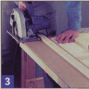
3 A simple cutoff jig precisely aligns the saw blade with the cut line, making it easy to match any angle you may need at the end(s) of the door.
