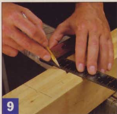
9 Align the ends of the upper stretchers and mark the centerline. Use a square to lay out identical notches for the tabletop center cleats.
