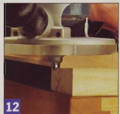
Raise the workpiece to provide clearance for the guide bearing. A board clamped flush with the workpiece edge can give added support for the bearing.
