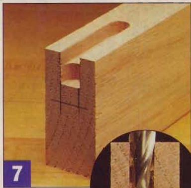
7 Make deep cuts in several passes. Also, an upcut spiral bit helps lift chips clear of the cut.
