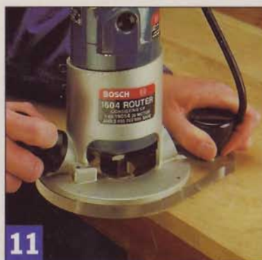
The wider stance and offset handle on an auxiliary baseplate gives you more control when edge routing, and helps keep the bit perpendicular to the edge.
