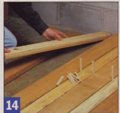
14 Place the tabletop boards, with the best faces down, on a clean, flat surface. A wall can help keep the ends aligned and spacers create uniform gaps.
