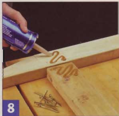
8 Spread construction adhesive on the mating faces of the joints. Realign the pilot holes and attach the rail and foot to the legs with #8 x 2 1/2" screws.
