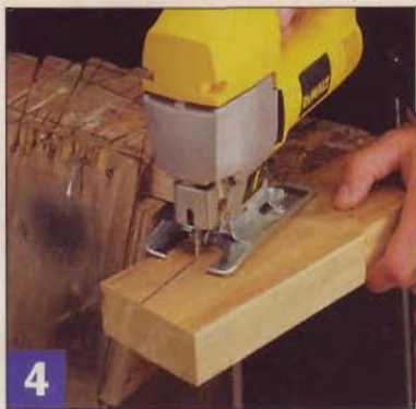
4 Layout the tapers on the top rails and feet, then make the cuts with a jig saw. Cut to the waste side of the line, then sand the pieces flush to your line.
