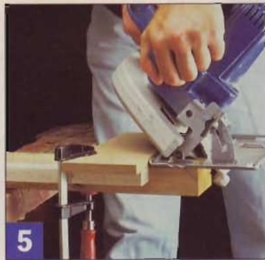
5 Clamp your cut-off guide to the center rail, tilt your circular saw to 45° and bevel one end. Reposition the guide and bevel the other end.
