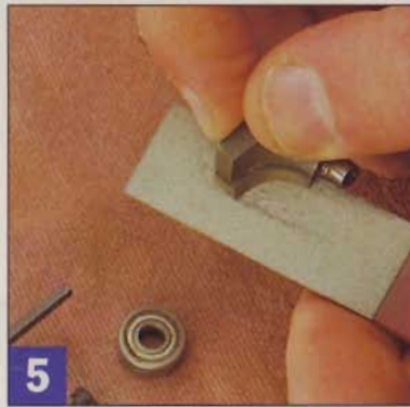
Use a crystalline diamond sharpening hone to touch up the edges of a carbide bit. Be sure to hone only the flat side of the cutting edges.
