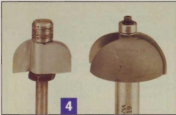
High-speed steel bit (left) produces inferior cuts. Choose carbide-tipped bits (right) with anti-kickback bodies that limit the “bite” the bit can take.
