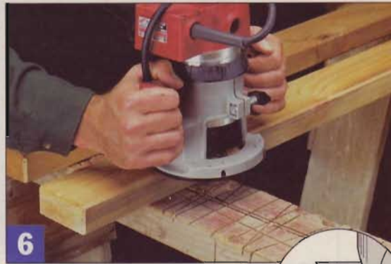
6 For some insurance against splinters, rout a 1/8"-deep chamfer on all edges and ends of the pieces, except the upper edges of the top rails.
