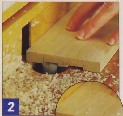
2 Turn the stock end-for-end and make a second pass. Move the fence to make the third pass.
