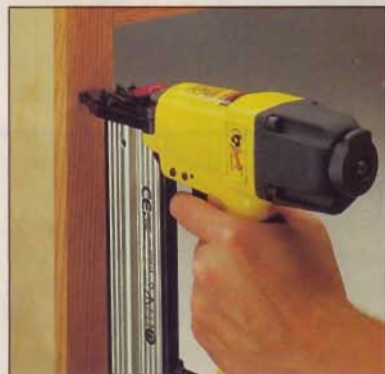
A brad nailer makes quick work of mounting cabinet face frames, and leaves a clean, countersunk nail.
