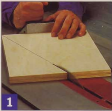
1 A piece of sandpaper taped to your miter gauge will keep the plywood from slipping while you make the angled cut.
