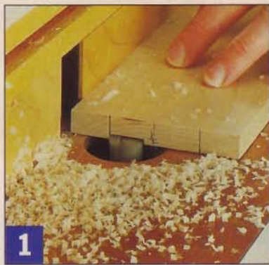
1 Layout the 2"-wide groove on an extra-long blank and adjust the router fence to make the cut that defines one edge of the groove. Use a 3/4"-dia. bit.
