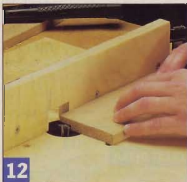
12 Rabbet the dial supports with a 3/8"-dia. straight bit. Make two shallow cuts to get the full 1/4" depth of the rabbet. Then bevel the ends at 5°.
