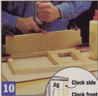
10 The clock side rests against a tall fence in the gluing jig. Add case cleats after both sides are on.
