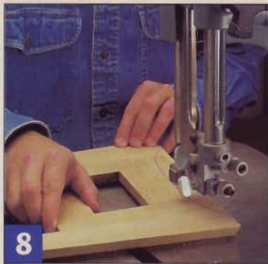
8 Use your band saw or jig saw to cut the arch opening. Stay just to the waste side of the layout line, then sand the arch smooth.
