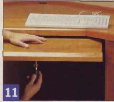
11 Attach the keyboard slide to the underside of the corner top according to the manufacturer's instructions. Then install the keyboard tray to the slide.
