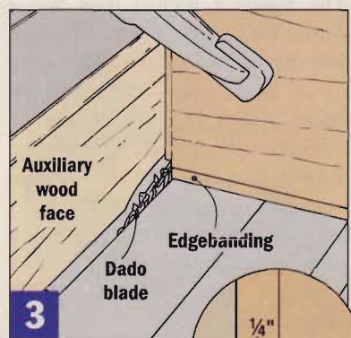
3 To trim the edge banding off the tongue, flip the panel on edge and guide it with your miter gauge.
