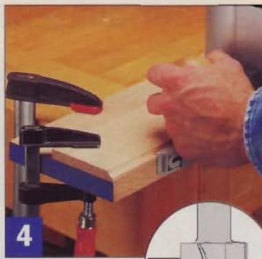
4 Clamp the shadow molding to another board for safety when routing the cove on this thin stock.
