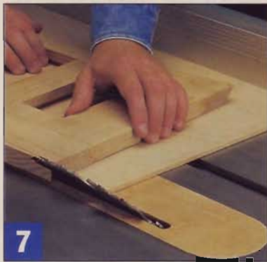
7 Aligning the clock front with the edge of a plywood sled lets you cut the angle for the sides and the 45° bevel in one step. Take it slow for a straight cut.
