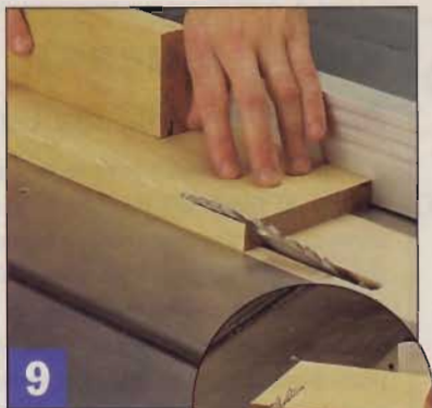
9 Press down on the side as you cut, and guide the stock with a push block. Bevel the ends at 5°.
