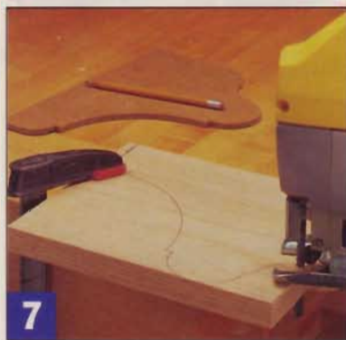
7 Trace the hardboard template onto your stock. Cut the end cap with a jig-saw, staying just outside the lines, then sand and file the cap to shape.
