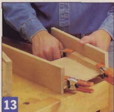
13 Glue the cleats to the dial supports first, then glue on the dial backer. Spring clamps work well to hold the pieces in place as the glue sets.
