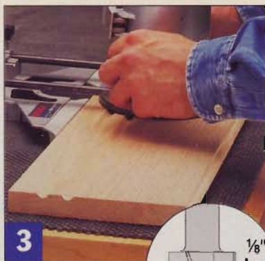
3 Using the router's edge guide, rout the three plate rail grooves with a 1/2"-dia. core box bit.
