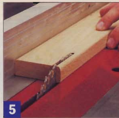
5 To make the retaining strips, roundover all the corners of some 3/4"-thick boards, then rip a 1/2"-wide strip from each edge.
