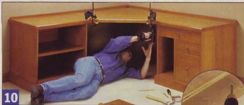
10 Position the corner and pedestal tops firmly against each other and clamp them together. Attach a wooden cleat across the joint for reinforcement.
