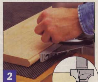
2 Routing the shelf's edge takes two passes. For the second pass use an edge guide.
