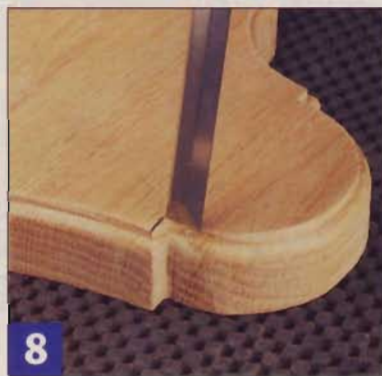
8 The roundover bit can't reach into tight, inside corners, so you'll have to chisel out what the router missed. Cut with the grain first to avoid tearout.
