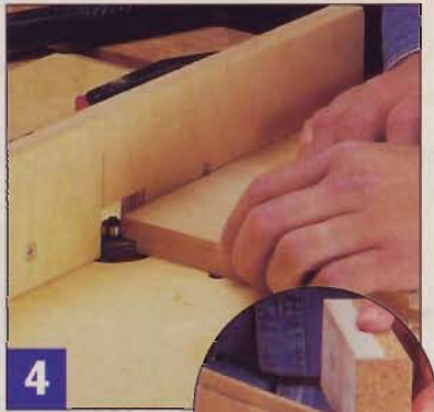
4 Test your router table setup using scrap stock, then form tenons on the front panel and rail.
