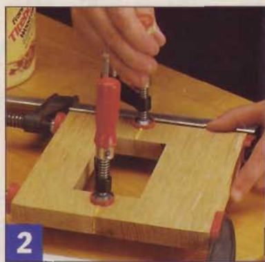
2 Careful grain matching and gluing make the two-part front panel look like a solid piece. Clamp across the joint to help keep the panel flat.
