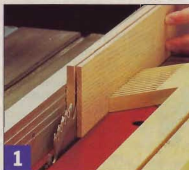
1 Resaw in several passes, raising the blade about 1/2" between cuts. Cut into both edges before raising the blade.
