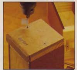
A simple jig centers the card holder pulls. Install the pulls with screws to keep them firmly fastened to the front of the drawer.
