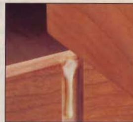
Put a glob of glue at the front of the dado and let the mating board spread the glue as it's inserted.
