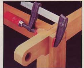
If the notch in the secondary leg fits loosely on the top rail, clamp the tab so it's firmly glued to the top rail.
