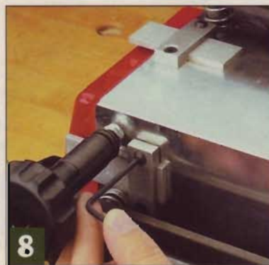
Stops on combination jigs adjust independently for different operations.
