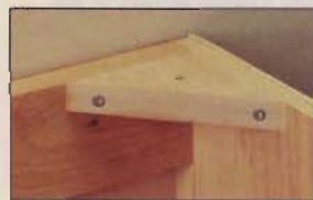
The nailer fits between the carcass sides and against the back. A brace adds support.
