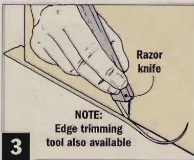
3 Let the glue cool completely before trimming the excess veneer.
