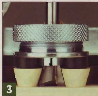
3 A guide bushing, secured to the router base, follows the template's fingers.
