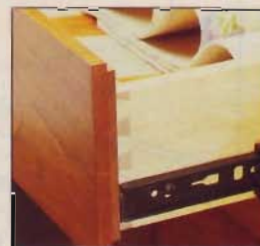
The drawer boxes feature 1/2" birch sides joined at the front and back with half-blind dovetails
