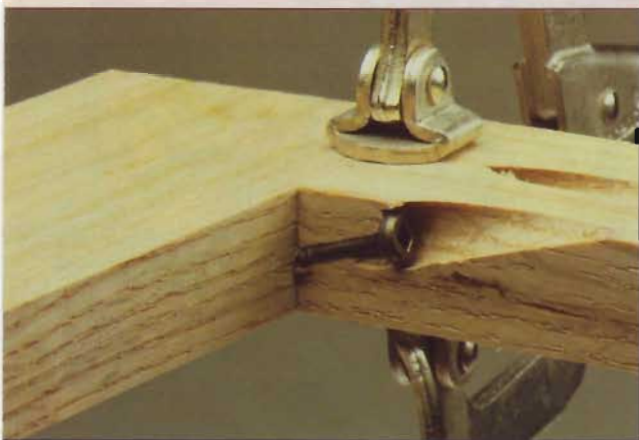
Another cutaway shows a self-tapping screw seated in the pocket hole. A special clamp holds the faces flush.
