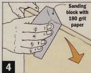
4 Sand lightly with the grain to avoid tearing the thin veneer.
