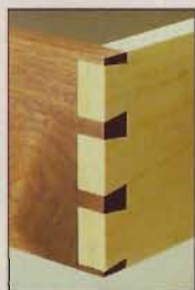
The pins and tails are visible on both sides of a through dovetail joint. This joint looks great from any angle.
