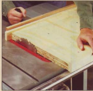
STEP 2: Trim ends flush using the table saw. Side edgings can be attached and trimmed the same way.
