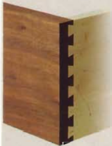
Standard half-blind dovetails
