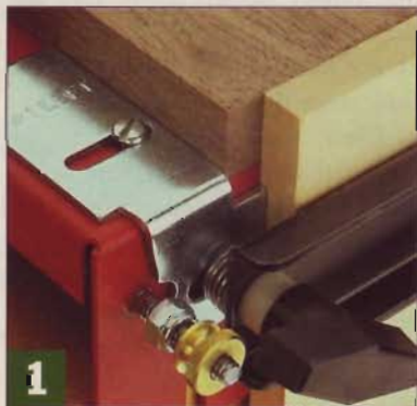
1 A single stop automatically positions the workpieces with the proper offset.
