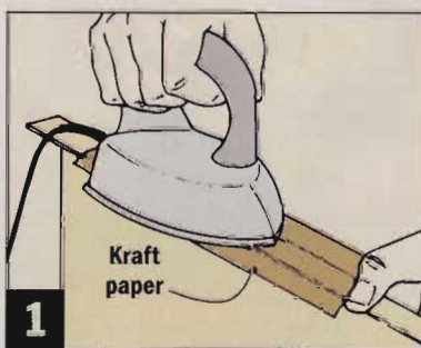
1 Move the iron steadily and don't let it sit too long in any one place.
