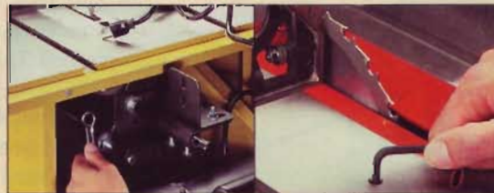
STOP ADJUSTMENTS: Reaching underneath to set the stops (left) is tougher than up-top adjustments (right).
