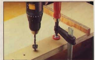
Use a stop collar to control the depth of the shelf pin holes.
