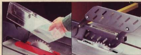
BLADE GUARD: Delta's guard (left) won't stay up, which is awkward. Powermatic's (right) flips out of the way.
