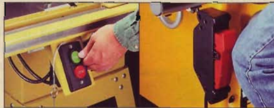
POWER SWITCH: Rail-mounted switches (left) are the norm. DeWalt's (right) can be shut off with your knee.
