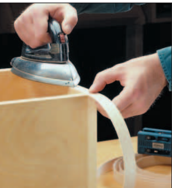
Iron-on veneer tape is an easy way to cover plywood edges.
