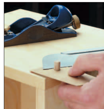
Dowels or wood plugs fill screw-holes and are trimmed flush.
