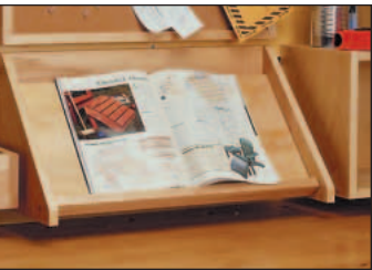
A slanted shelf holds plans while you're working in the shop.
