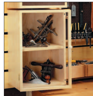
A door with 1/4" acrylic panel keeps out dust and still lets you see inside.
