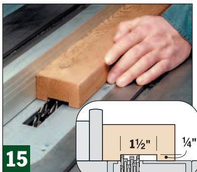
15 To accept the balusters in the lintel (and to fit over the stretcher), cut a centered groove in rails (H) and (J).
