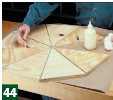
44 Carefully turn the roof over and brush a generous amount of glue in each joint and on one of the two exposed edges.
