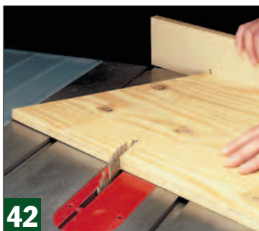
42 Flip the plywood over, align the tip of the triangle to the outside of the kerf in the fence and cut the second side.
