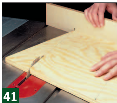
41 Tilt the blade to 10° and the miter gauge to 20 1/2°. Trim one end of the plywood blank.
