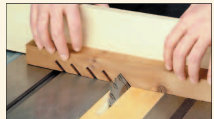
When cutting the angled slots in the stiles of the cupola's side panels, a jig with a wood index key ensures even spacing
