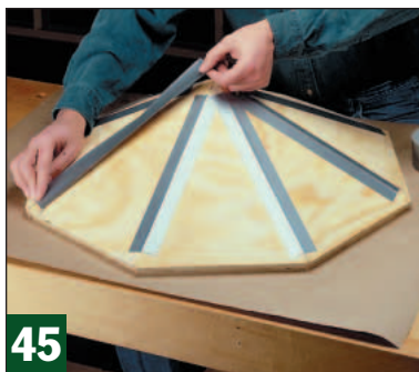
45 Turn the roof back over and pull the last joint together. Then tape it closed and let the glue dry overnight.
