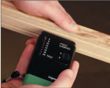
To check the moisture content, jab the prongs of the meter into the bottom of a strip of wood flooring.
