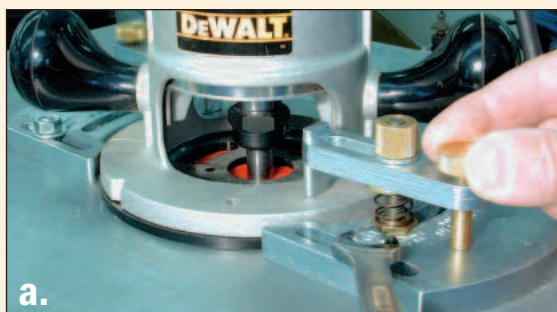
a. A unique, quick-clamp mechanism on the Veritas router table lets you mount or remove the router in seconds.
