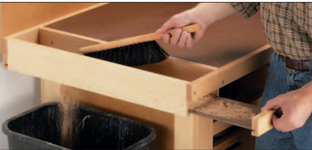
▲ To make it easy to clean the tool tray, just pull out the bottom and sweep dust and dirt into a trash can.
