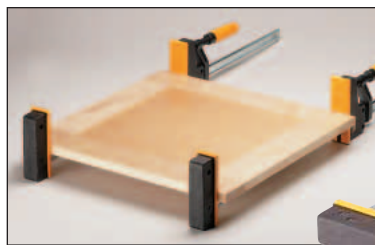
▲ The parallel jaws on these clamps ensure flat, square assemblies when gluing up a project.
