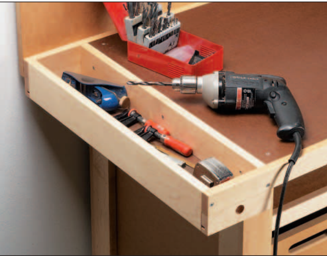
▲ A shallow tool tray mounted to the end of the bench holds small hand tools and keeps the work surface free of clutter.
