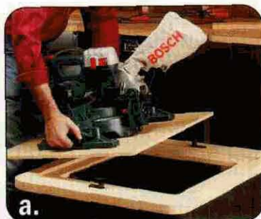
a. Quick-change inserts bolt directly to portable tools and then lock into the cabinet tops for easy changeovers.
