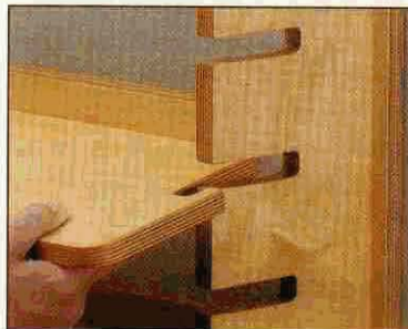
◀ Interlocking notches in the shelves and end supports create a strong shelf unit.
