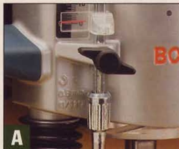
▲ Bosch's unique depth setting system has an extension at the bottom of the plunge rod for fine adjustments.
