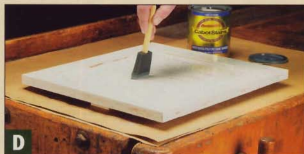
▲ In addition to the extra protection it provides, the topcoat "evens out" the dull spots caused by sanding. I used a water-based polyurethane finish to prevent the paint from yellowing.
