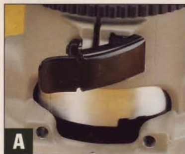
▲ The new lever release on the fixed-base makes depth adjustments and motor changes quick and easy.
