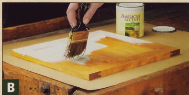
▲ Then brush on two coats of a satin, latex paint. When each coat dries, remove any "nibs" with 400-grit wet/dry sandpaper. To avoid clogging the sandpaper, I used water as a lubricant.
