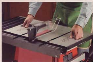
▲ Handles cut into the aluminum table let you take the saw to the work.
