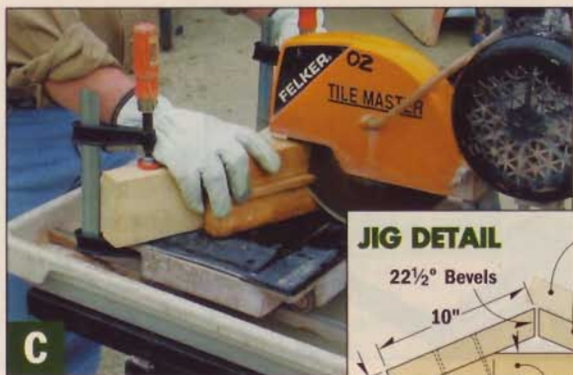
C I used a jig on a tile saw to bevel cut the stones for the corners of the firepit.
