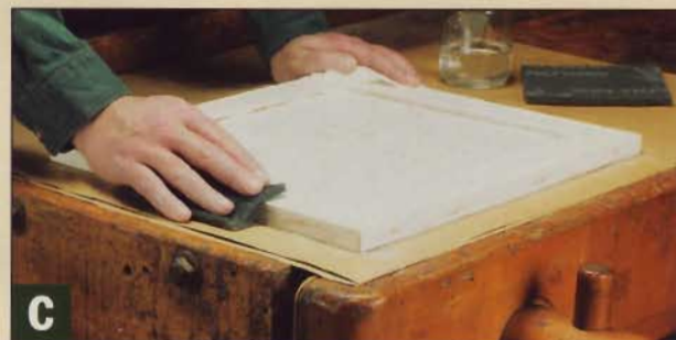
▲ Use an abrasive pad to sand through areas that are likely to get the most wear — edges, corners, and around knobs. I also sanded the beads on the door and side panels (photos above).
