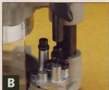
▲ The six-position turret is one small part of an excellent depth adjustment system on the plunge base.
