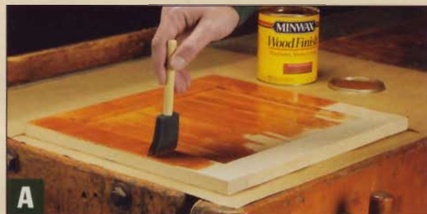
▲ To begin the "aging" process, start by applying a dark-colored stain with a foam brush. Don't worry about getting a nice, even stain. Just brush it on, then wipe off the excess with a rag.
