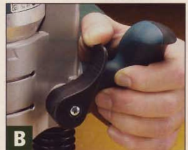
▲ Pistol-grip handles and an easy-to-reach plunge lever make this router comfortable and controllable.
