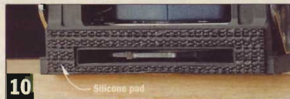
◀ Similar to a router mat, Ryobi’s anti-slip material is effective, though a bit “squishy.”
