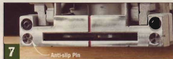
◀ Anti-slip pins, such as on the DeWalt, are effective only on wide boards.
