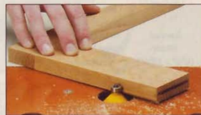
▲ Rout a \frac{1}{8} " chamfer on the outside edge of each end stile before adding the middle rail.
