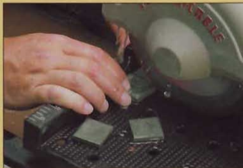
▲ A "wet wheel" tile saw makes quick work of cutting the 3" tile into four pieces. Be sure to keep your fingers back.
