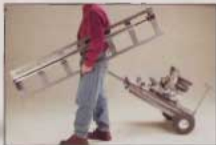
◀ The basic stand folds down, with the saw mounted, into a mobile cart. The support and stop options are a bit of a burden to move.
