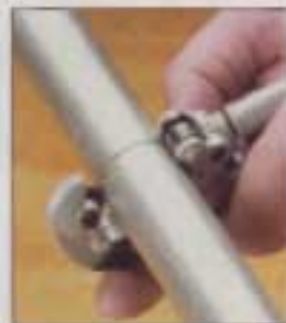
▲ An ordinary tube cutter makes quick, clean cuts in the 1"-dia. conduit used to make the sawhorse legs.
