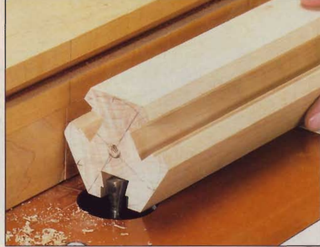
▲ The sockets that hold the legs are formed by routing a wide, shallow groove and a deep, dovetail-shaped groove.
