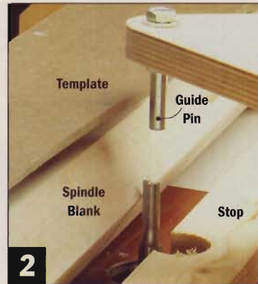
▲ With the spindle blank mounted in the carriage, raise the bit so it sticks up above the center of the blank.
