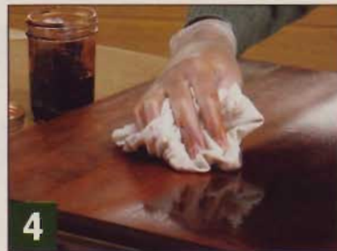
▲ Once the surface is saturated, use a clean, soft cloth to remove excess dye before it has time to dry.
