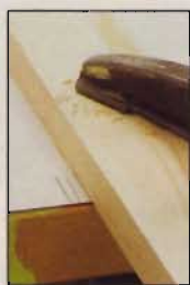
▲ Use pencil marks to gauge each adjustment of the stop.
