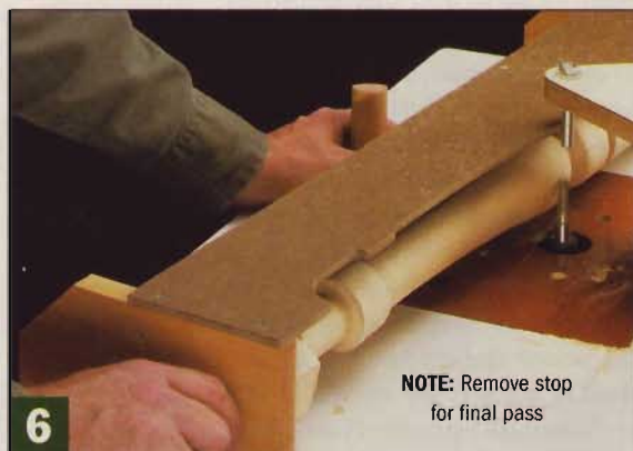
▲ When the rough shaping is done, carefully go back over the entire spindle to remove any ridges or high points you might have missed in previous passes.
