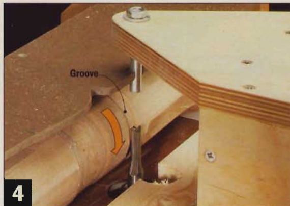
▲ Begin shaping the grooves slowly, nibbling away just a small amount of material at a time by rotating the spindle into the router bit.
