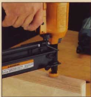
▲ DEPTH ADJUSTMENT In this test, we tried to set a nail perfectly flush to determine how adjustable the depth settings are.
