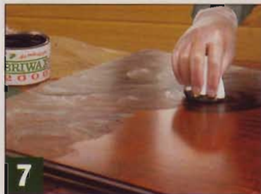
▲ After applying the final coat of shellac, rub on a coat of dark brown paste wax to hide any tiny blemishes.
