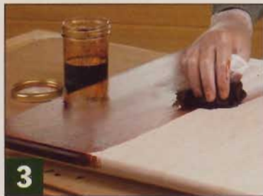
▲ After preparing the dye, flood the surface with dye and keep a “wet” edge at all times to avoid lap marks.
