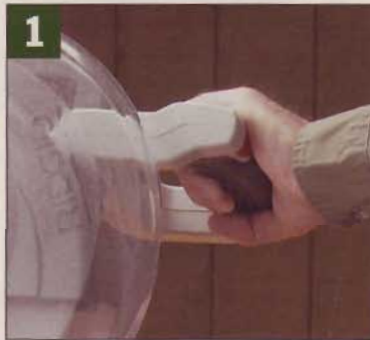
▲ The safety switch on the Ridgid appears to favor right-handed operation, but it's easily depressed with the heel of the left hand.
