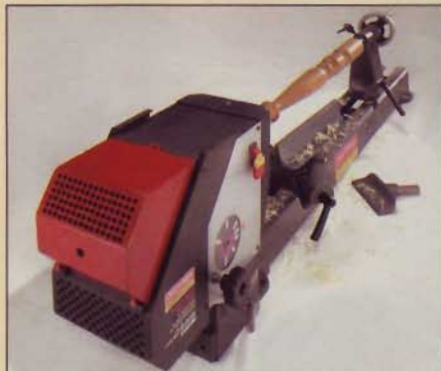
▲ Craftsman's new 15" wood lathe boasts a 2-hp motor, 20" of outboard capacity, and 38" between centers for turning spindles.
