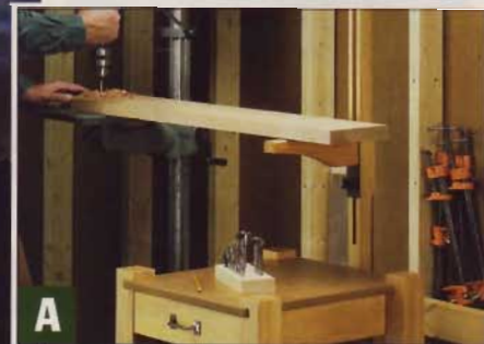
▲ To hold the end of a long workpiece, you can quickly remove the light and use the arm as a handy stock support.
