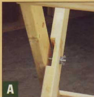
A The key to the work table's knock-down flexibility is the dado/carriage bolt assembly.
