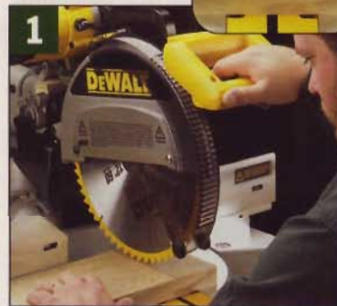
▲ The handle and trigger are easy to use with either hand. Slots in the blade guard provide a clear view of the intended cut line (Detail a).
