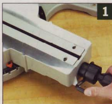
▲ Makita made their saw user friendly with easy operating controls for the detent override (the lever) and rail lock (the thick collar).
