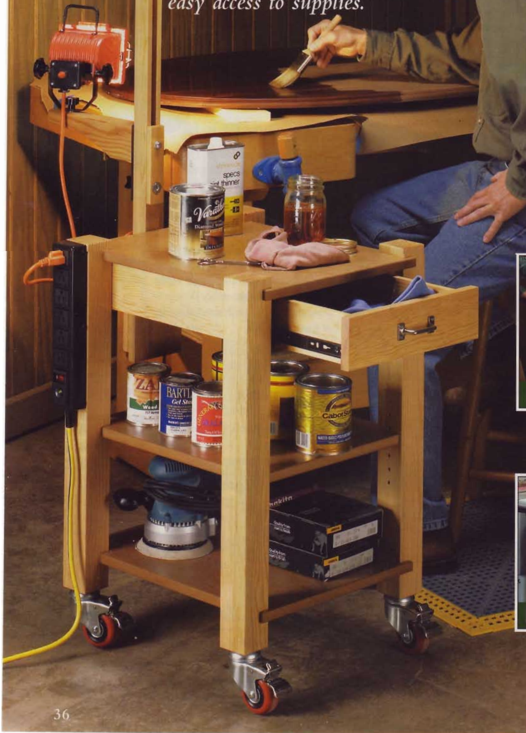
▲ To hold the end of a long workpiece, you can quickly remove the light and use the arm as a handy stock support.
