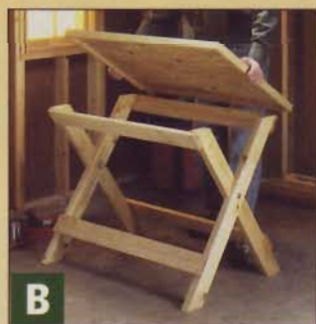
B The tabletop simply screws onto the tops of the legs to provide a sturdy work surface.
