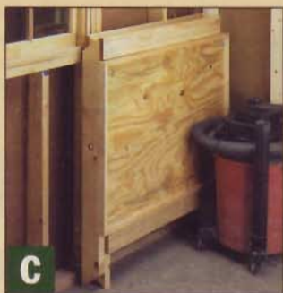
C When the job is finished, the work table folds up completely to tuck away in a corner.
