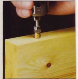
▲ To install a threaded insert, chuck a cutoff bolt with a couple of “jam” nuts in the drill press. Then turn the chuck by hand.
