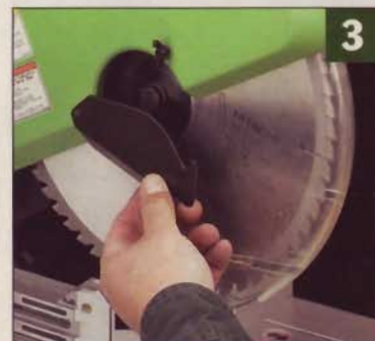
▲ Blade changing on the Hitachi is easy thanks to a cover that offers quick access to the arbor.
