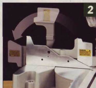
▲ Extending the subfence or moving it to allow the saw to bevel all the way to the left is a simple matter of flipping it out of the way.
