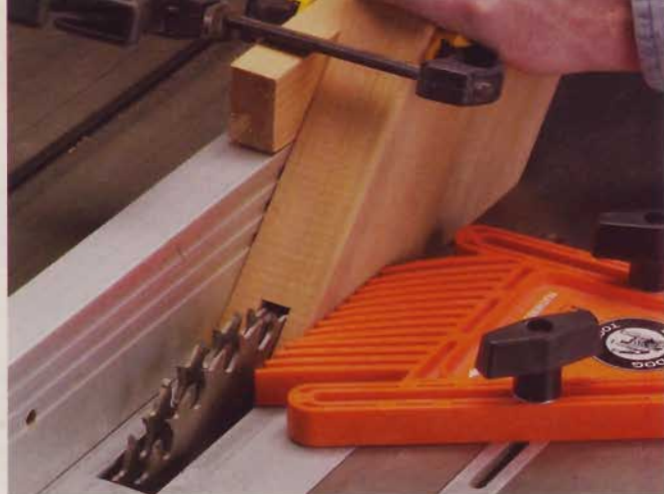
▲ A block clamped to the mitered frame piece and a featherboard ensure accuracy and safety when cutting the grooves for the splines.
