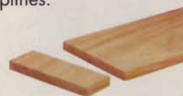
▲ Cutting splines from the length of the board creates the strongest joint.
