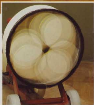
▲ To avoid gouging the floor, the ezV sander has three random-orbiting heads, like the heads on an electric razor.
