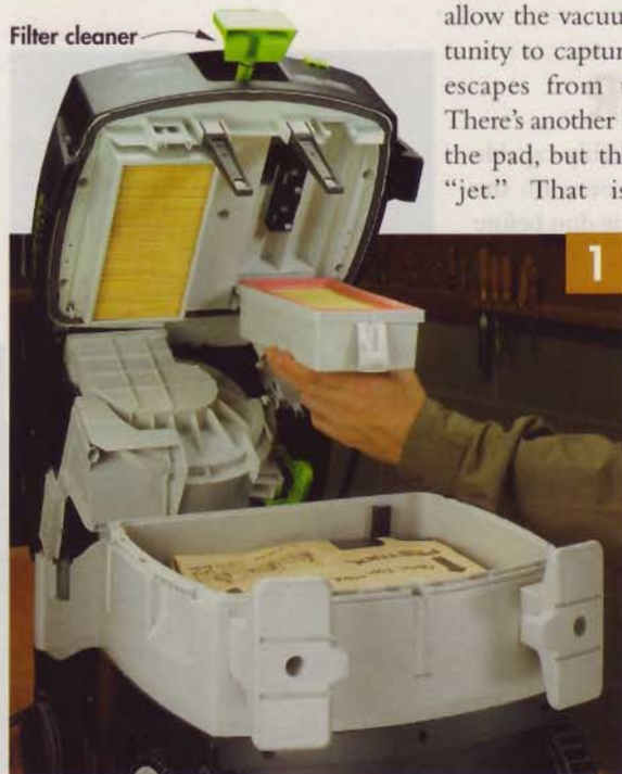
▲ A filter cleaner makes maintenance cleaning convenient. For more thorough cleaning or replacement, the filters snap out easily.
