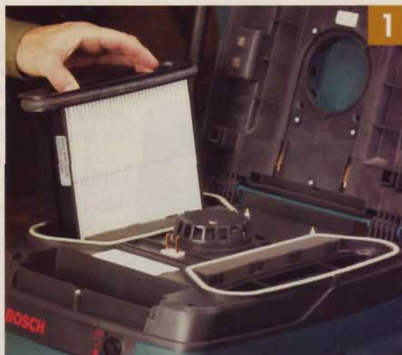
▲ The Bosch's pleated filters combine with a dust bag to capture nearly 100% of particles 3 microns and larger.
