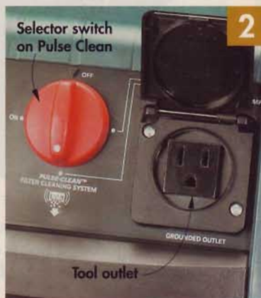
◀ A Pulse Clean mode automatically cleans the pleated filters. Also shown is the outlet for tool-actuated operation.
