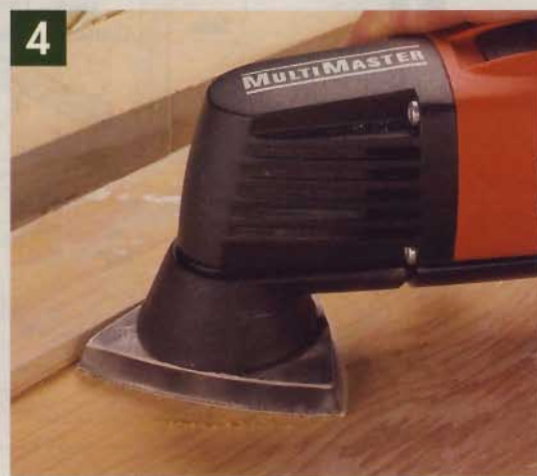
▲ Tight corners are no problem for the tapered, triangular sanding pad of the MultiMaster. Note also the effectiveness of the dust-free accessory kit (Fig. 1).
