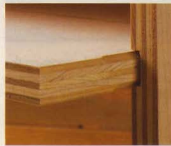
▲ To make it easy to slide the panels into place, rout chamfers on the top and bottom edges, stopping them about 2" from the front edge ( Inset Photo ).
