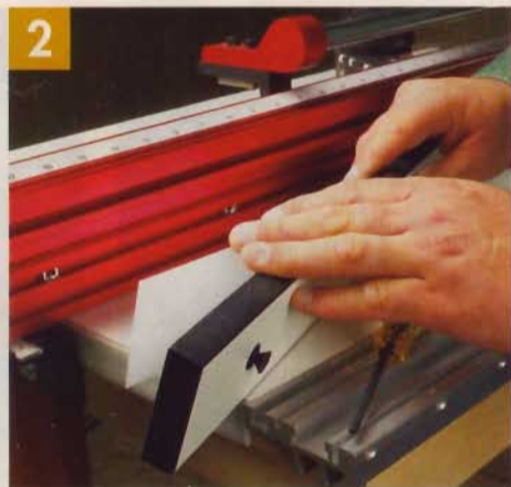
▲ The Mast-R-Fence uses plastic shims to offset the outfeed sub-face for jointing. They're a bit tricky to install, however.
