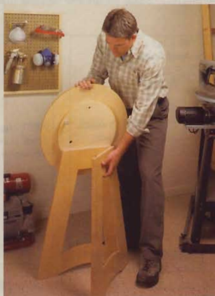
▲ To set up the finishing station, raise the turntable, which is hinged to one side, and then swing the other side open.
