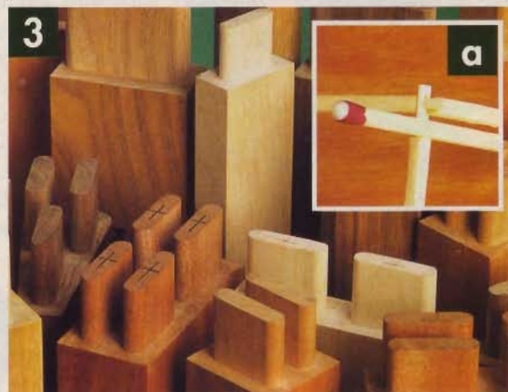
▲ From matchstick-sized tenons to triple and quadruple joints, the FMT offers almost endless possibilities for mortise and tenon design.
