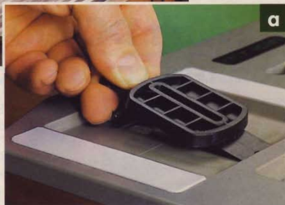
▼ The basic FMT jig comes with five templates that are capable of more than 20 sizes of mortise and tenon joints.
