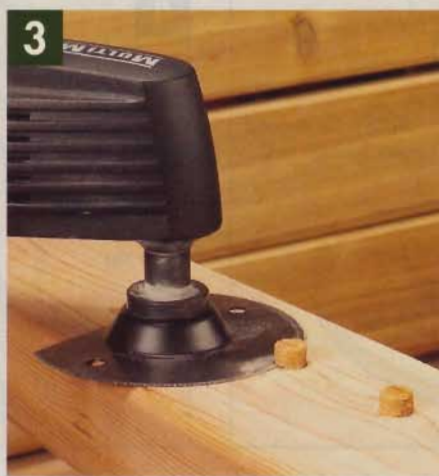
▲ A flush-cut blade on the MultiMaster is a fast and clean way to remove plugs or caps. It's also a great jamb saw for undercutting walls or molding.
