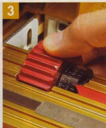
▲ A micro-adjustment knob and "zeroable" scale allow for adjustments as fine as .001".
