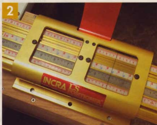
▲ Interchangeable scales are marked for specific joint types and sizes. The steel rule slides in its slot to allow the fence to be "zeroed" out.
