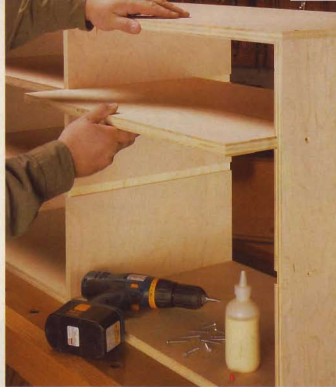
▲ To make it easy to slide the panels into place, rout chamfers on the top and bottom edges, stopping them about 2" from the front edge ( Inset Photo ).
