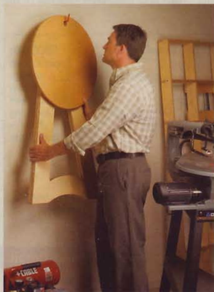
▲ Thanks to its unique, space-saving design, the finishing station can be folded flat and hung on the wall.
