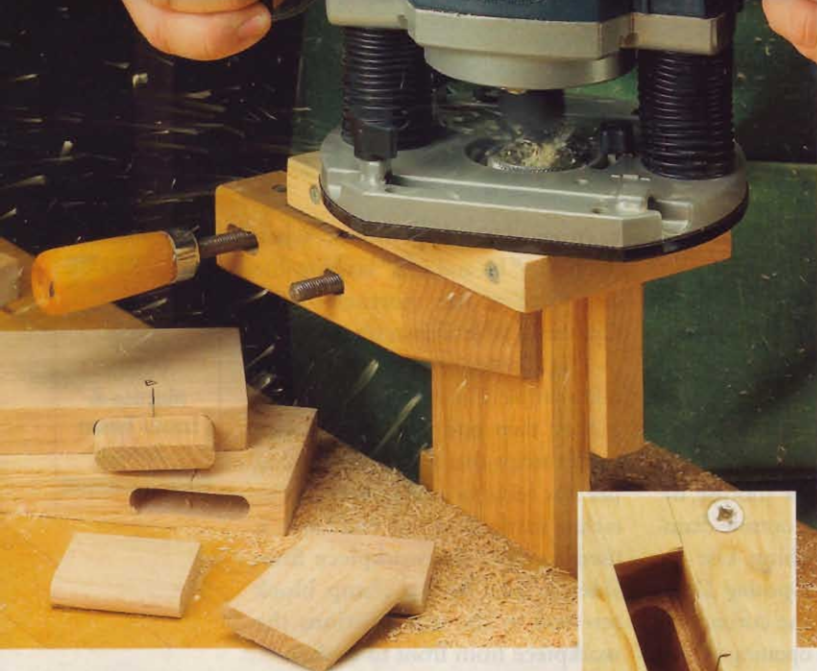
▲ With the T-shaped mortising jig clamped to the workpiece, make a series of progressively deeper passes, routing from one end of the opening to the other to cut the mortise ( Inset ).
