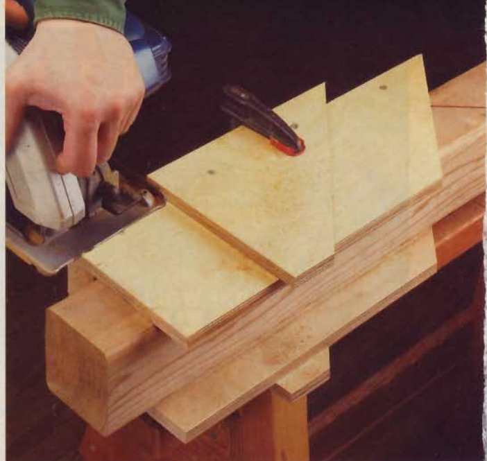
▲ When using a circular saw to crosscut or miter a 4x4 post, this U-shaped cutting guide lets you make two perfectly aligned cuts — one from each side.
