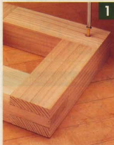
▲ In order to cut the bevels on the top face of each mid-cap, temporarily assemble the two unglued joints with brass screws.
