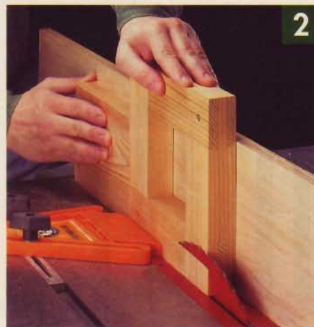
▲ Once the mid-cap is assembled, tilt the saw blade 10^\circ . Then, after attaching a tall fence and featherboard, make a beveled cut on all four faces of the mid-cap.
