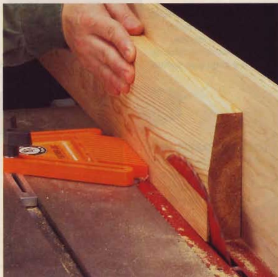
▲ After installing a tall auxiliary fence and featherboard, tilt the table saw blade 5° and then rip a wide bevel on both edges of the rail cap.
