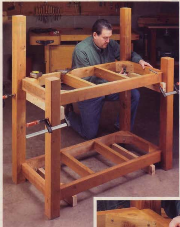
▲ A pair of scrap 2x4s hold each frame at the correct height while securing the legs with lag screws ( Inset Photo ).
