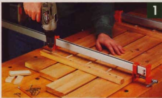
▲ To assemble the panels, use 1/4"-thick blocks to space the slats evenly. Then clamp across the panel and attach temporary cleats to keep the slats aligned.
