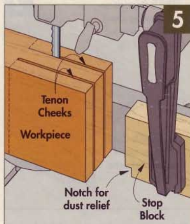
▲ Once the setup is just right, cut tenon cheeks like the mortise sides, flipping the piece between cuts.
