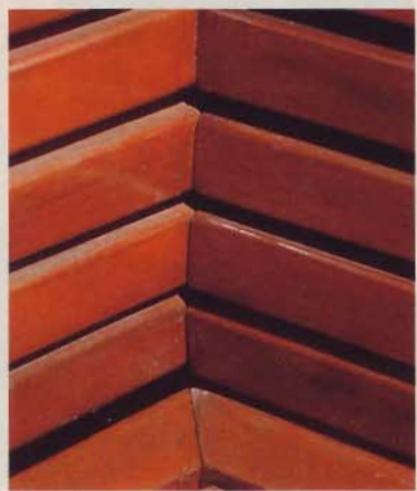
▲ Corner Craftsmanship Compound miters and scribed joints result in a perfect fit where the seat slats meet in the corner.
