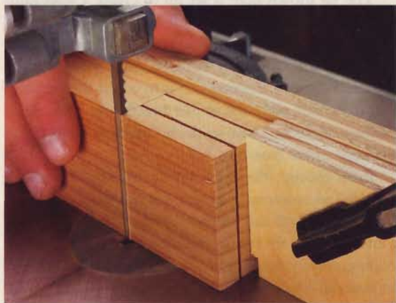
▲ For square, precise tenon shoulders, use a miter gauge on the band saw. Here the stop block determines the length of the tenon.
