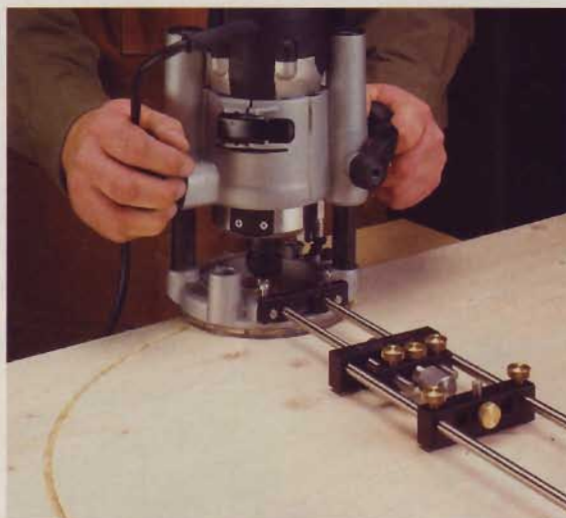
◀ The circle jig accessory kit turns the MicroFence into an incredibly accurate circle jig for diameters ranging from 6" to 24".
