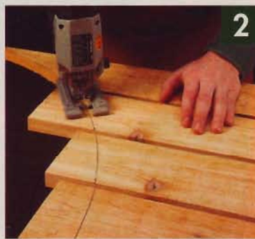
▲ After laying out the arcs on the panels (see page 24), use a jig saw to cut them to shape.
