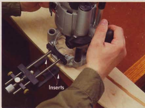
◀ Half-round inserts on the MicroFence make it capable of following contours, such as when routing a groove parallel to a curved edge.
