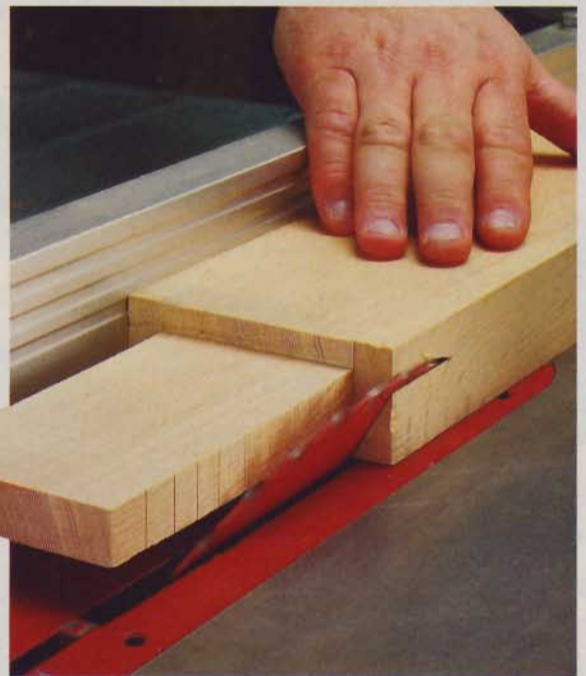
▲ After tilting the saw blade to 20°, rip a wide bevel on the top edge of the lower rail. This bevel will help shed water once the project is assembled.
