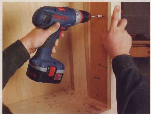
▲ For accurate results, butt the same edge of the hole template against the face frame (shown) and the divider when drilling the shelf support holes.
