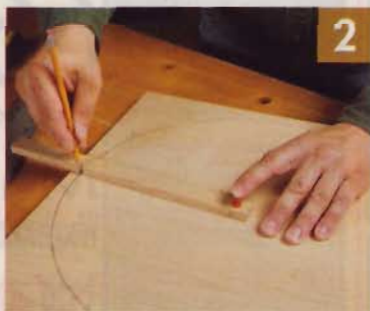
▲ Using a compass made from a scrap of wood, draw the circle on the top face of the workpiece.
