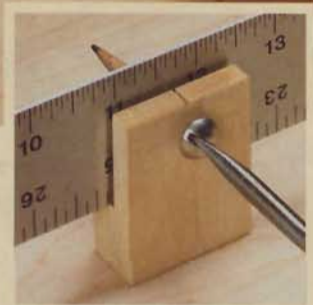
▲ A 36" steel rule and two wood blocks combine to make a simple beam compass. An adjustable marking block ( left ) lets you draw circles up to six feet in diameter.
