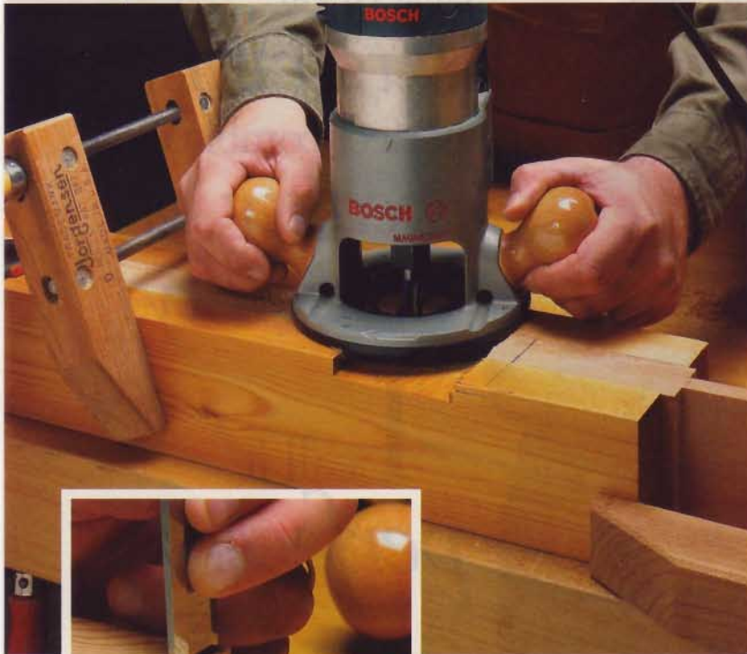
▲ Scrap blocks clamped to a rail provide a stable surface that keeps the router from tipping as you rout a mortise. Use a chisel to square up the shoulders ( Inset ).
