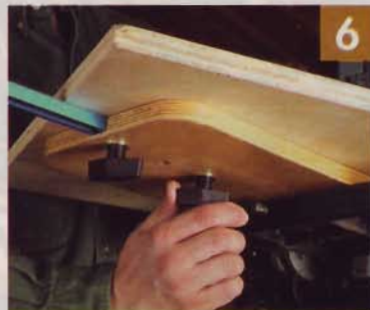
▲ When the blade begins to cut along the circle ( Fig. 5 ), tighten the knobs and complete the cut.
