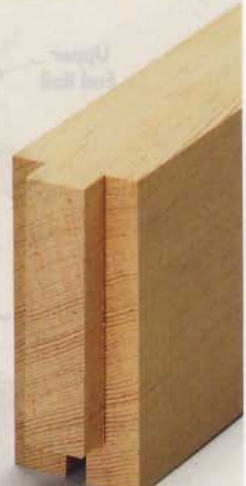
▲ Stub (short) tenons on the end rails are cut to fit snugly into slots in the legs.
