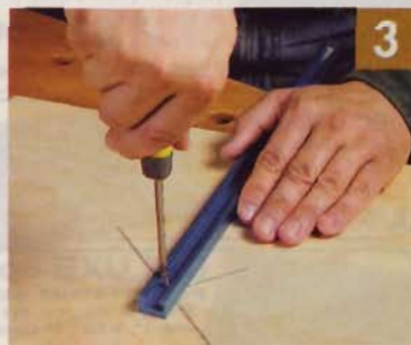
▲ Attach the rail to the bottom of the piece by installing the pivot pin (screw) at the centerpoint.
