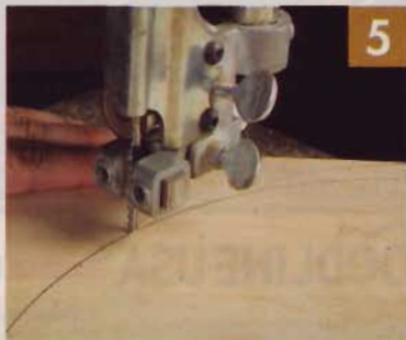
▲ Start the cut at the edge. Then cut toward the circle by rotating the work and sliding the rail in.
