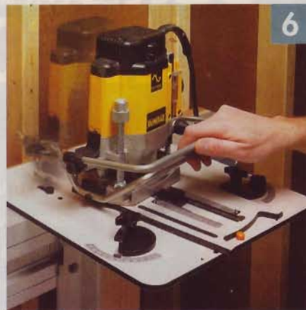
▲ WoodRat's optional plunge bar makes plunging the router to depth a one-handed operation.
