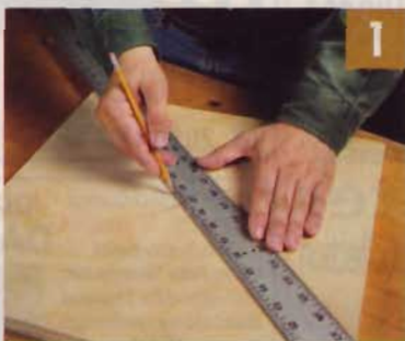
▲ Start by drawing diagonal lines to find the centerpoint on each side of the workpiece.
