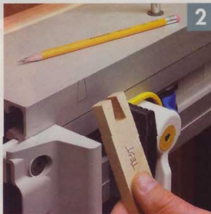
▲ Cut a socket in one test board. Move this board to the "Marker" position and trace the socket onto the channel.
