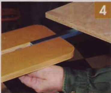
▲ Now slide the rail over the heads of the T-bolts. Note: Don't tighten the lock knobs just yet.
