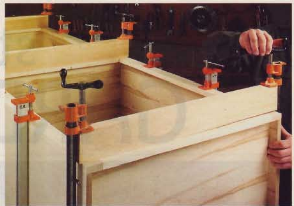
▲ Using a slightly tapered caul while gluing on the face frames ensures even distribution of clamping pressure. (For more on this, see page 34.)
