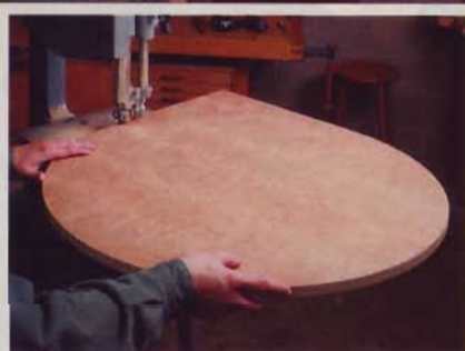
▲ A pivot pin on a sliding rail makes it easy to cut a circle on a band saw. With the rail inserted one way, you can cut smaller circles. Flip it end for end for larger circles (Inset).
