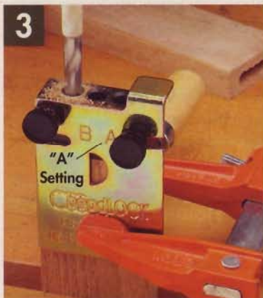
▲ With the jig clamped to the workpiece, lock the guide block to the left in the "A" setting. Drill holes.
