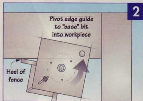
◀ To adjust the width of cut, the entire fence assembly slides diagonally in a groove in the base of the edge guide.
