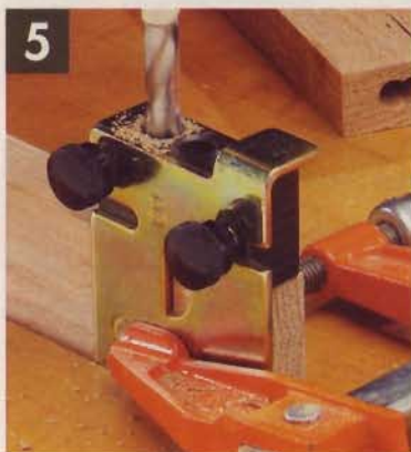
▲ Repeat the process described in Steps 2 through 4 to drill the mortise in the adjoining workpiece.
