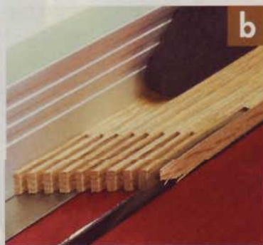
▲ Rip the waste material from the edge of the featherboard to make the last finger identical in width to all the others.
