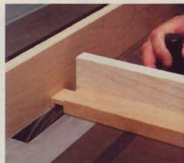
▲ To define the length of the tenon, butt the workpiece against an auxiliary fence, then make a pass.
