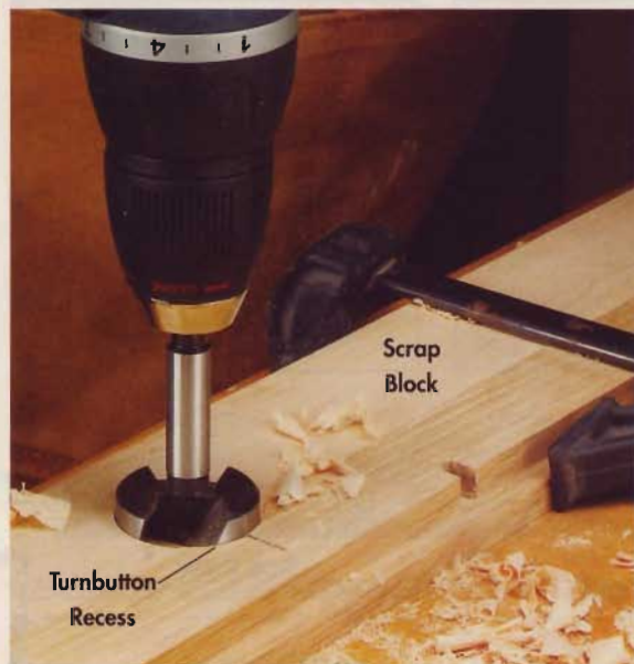
▲ I used a 2" Forstner bit to drill the shallow recesses that hold the turnbuttons. To prevent tearout, clamp a scrap piece against the outer edge of the stiles.
