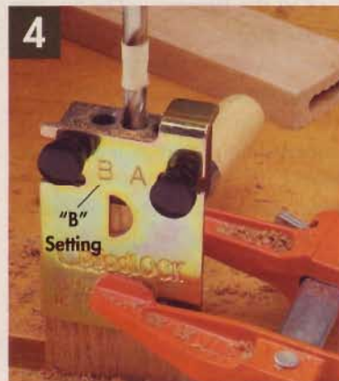
▲ Without unclamping, slide the guide block to the right, secure it in the "B" position, and drill holes.
