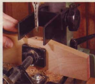
▲ A mortising machine and a \frac{1}{4} " square chisel and bit make quick work of cutting the mortises.
