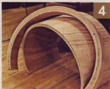
▲ The large, solid-wood molding mounts to a plywood base that is bent to shape on a cylindrical form.
