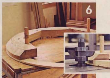
▲ A plywood ring and dowel handles aid in shaping a narrow molding that will cap the larger molding.
