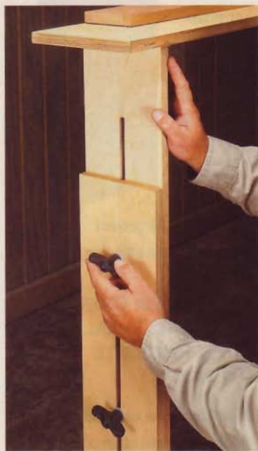
▲ The locking knobs and long slots in this two-part leg allow you to quickly adjust the height of the extension wing.
