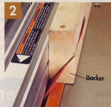
To make a backer, tilt the blade to match the molding's spring angle. Make a 12"-long bevel rip in a 2x4, turn off saw, then cut the backer to length.
