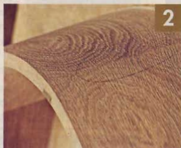
▲ The outer radius is formed by cutting the waste material with a band saw, then sanding the surface smooth.
