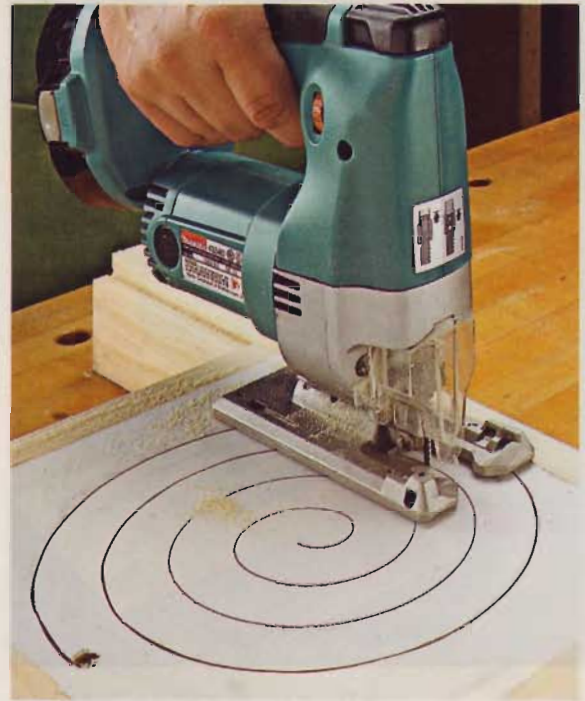
▲ Each saw was equipped with a 20-TPI scrolling blade to trace a tightening spiral. This measured the cornering and dust-blowing characteristics.
