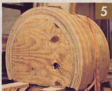
▲ To assemble these bases, multiple layers are glued up and bent around the form with band clamps.
