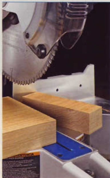
▲ This new 96-tooth 12" finishing blade from H.O. Schumacher & Sohn has a -6^\circ hook angle to produce ultra-smooth cuts.
