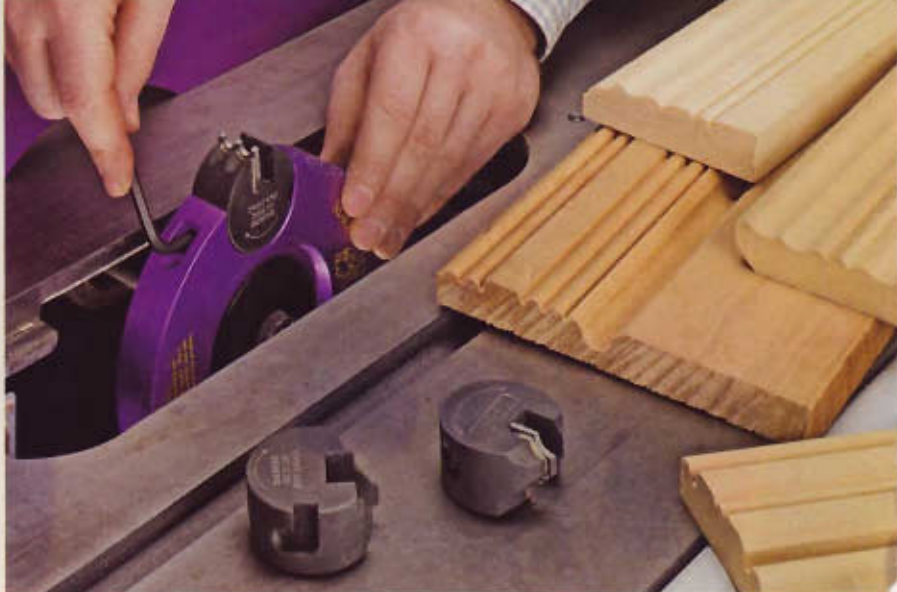
▲ The Magic Molder makes cutting molding on the table saw easy. You can even change cutters while it's still mounted on the saw.
