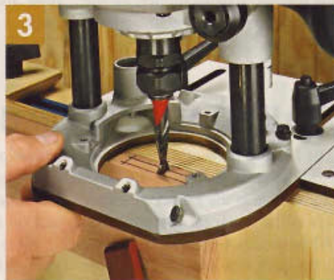
▲ Slide the router carriage into position so that the router bit aligns with the layout lines for the mortise, and then lock the knobs.
