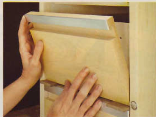
▲ A couple of 1/4" hardboard shims ensure even spacing between false fronts.
