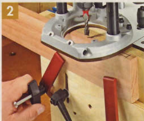
▲ Position the workpiece flush with the top of the jig. Then butt the fence against it, and clamp it in place by locking the hold-downs.
