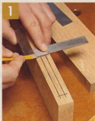
▲ Mark the ends, edges, and location of the mortise using a pencil and square.
