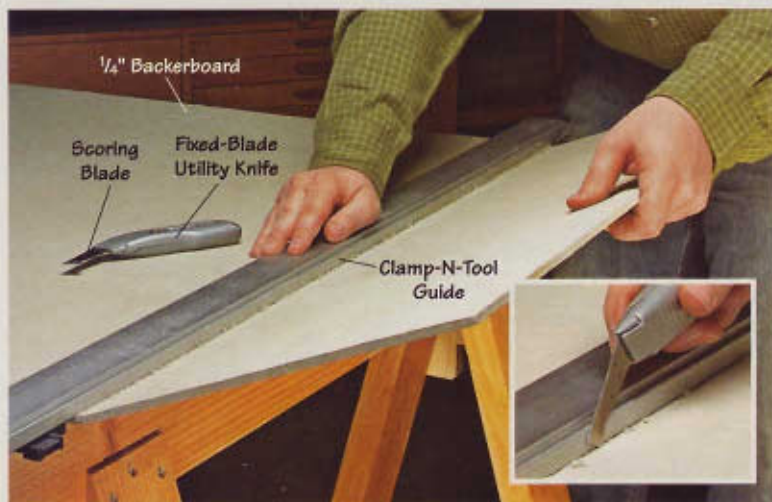
▲ To cut backerboard, first score it several times using a scoring blade guided by a straightedge. Then, snap it up toward the score line.
