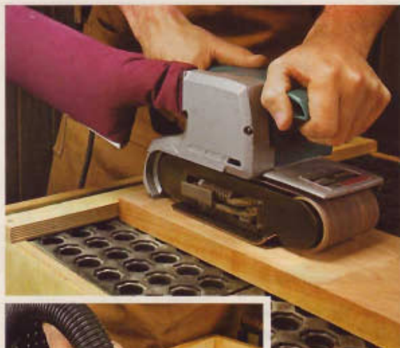
▲ A stop holds work in place when using a belt sander (top). Remove the mat and panel to vacuum the filters (left).
