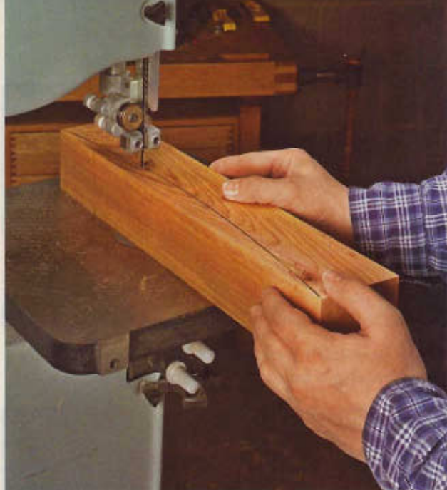
▲ The arcs on the stretcher pieces can be cut freehand on the band saw. After laying out the arc, cut to the waste side of the line, and then sand the surface to remove saw marks.
