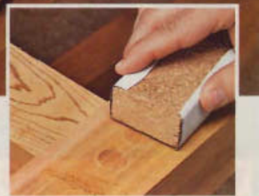
▲ Use an index card to protect the workpiece as you trim the plug. Then sand the plug flush with fine sandpaper, following the grain.
