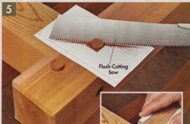
▲ Use an index card to protect the workpiece as you trim the plug. Then sand the plug flush with fine sandpaper, following the grain.
