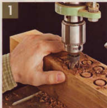
▲ Always cut to the full depth of the plug cutter. This chamfers the bottom end of the plug to make it slip easily into the hole.
