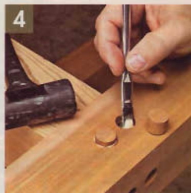
▲ To reduce squeeze-out, brush glue only inside the hole. Align the grain on the plug with the workpiece and tap it into place.
